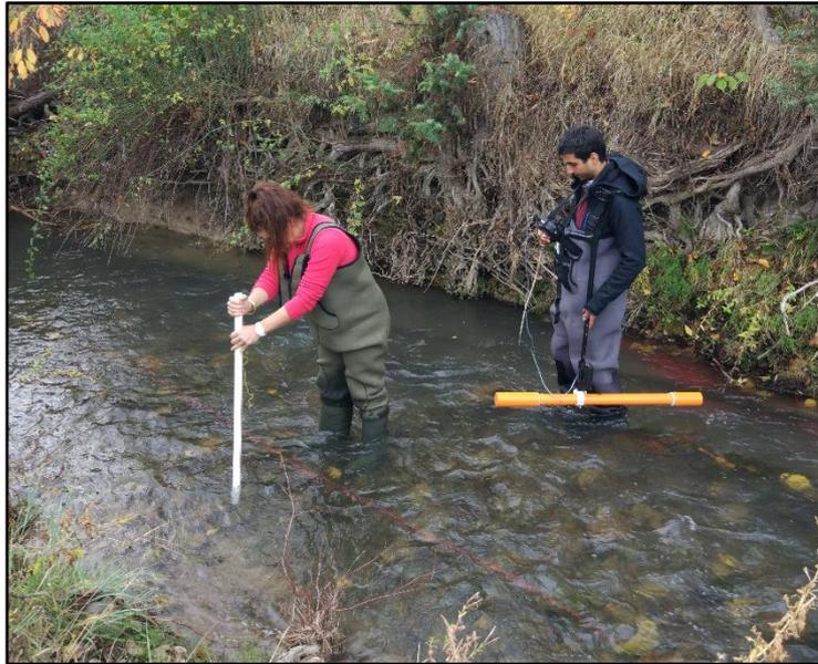
Figure 4.7. A view of EMI Survey conducted along Çakıt Stream. CMD (Orange device) is held horizontally at a certain distance from stream and HOBO (at the bottom of white stick) is dragged along the stream.
