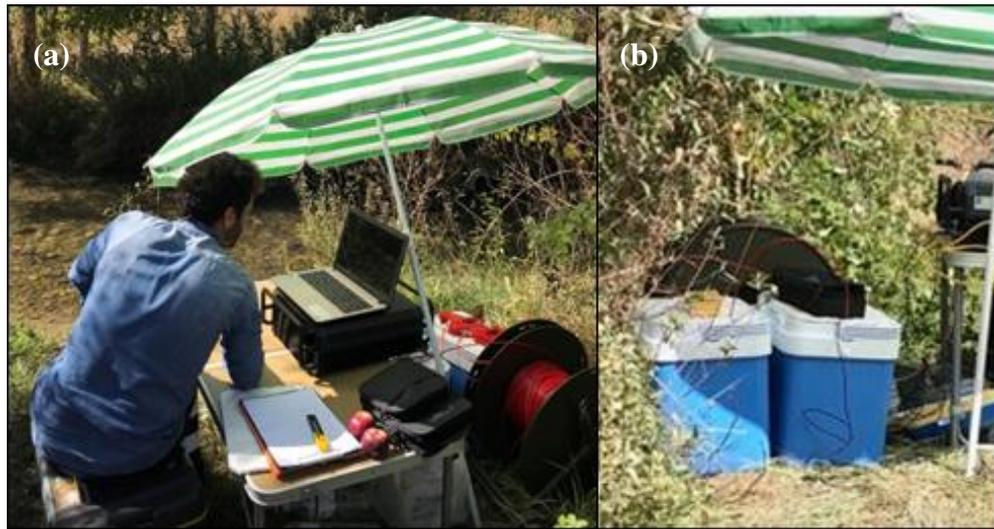
*Figure 4.13.* (a) A view of the field setup for the FO-DTS system and (b) calibration baths located near FO-DTS
