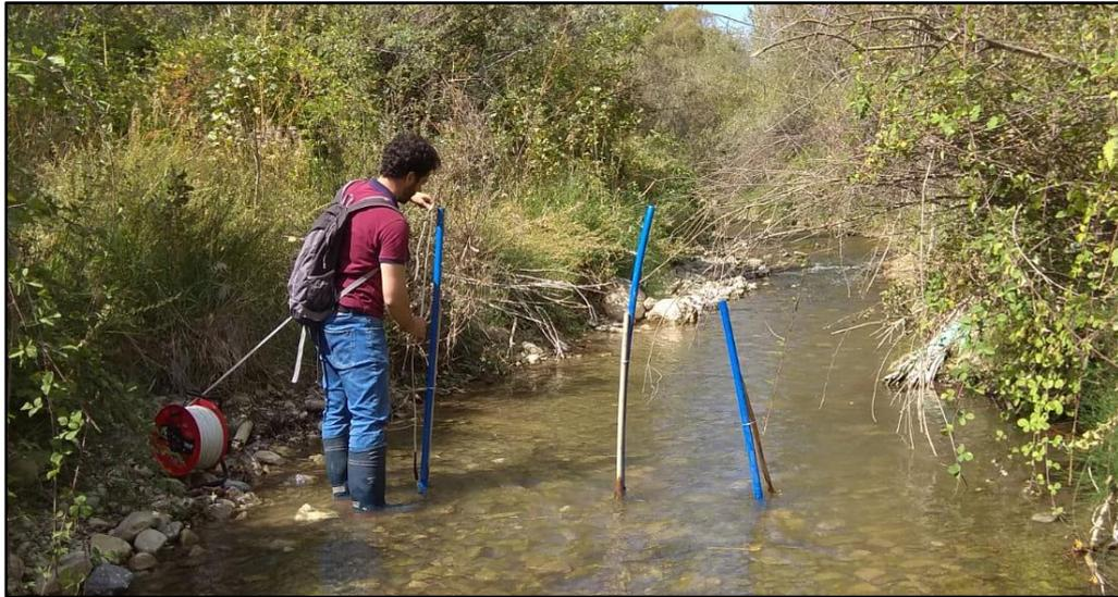
Figure 4.18. Water level, EC and temperature measurement using TLC meter
