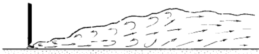
Figure 2.15. Form D – Effective Jump but Rough Surface Downstream (Strong Jump) (Chow 1959)
