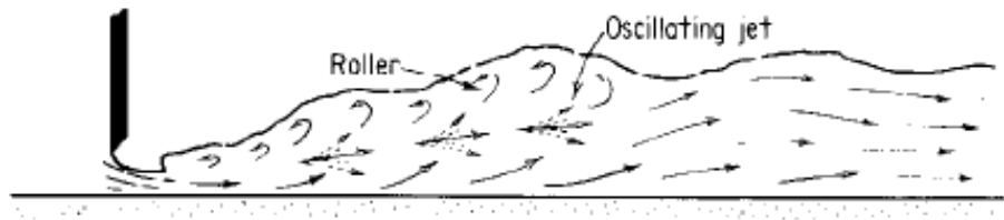
Figure 2.13. Form B – Transition Stage (Oscillating Jump) (Chow 1959)
