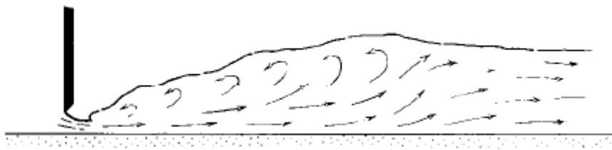
Figure 2.14. Form C – Well-balanced Jump (Steady Jump) (Chow 1959)
