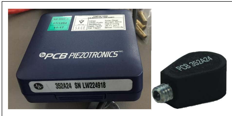
Figure 3-17: One of the accelerometers (calibration is valid until 20.11.2019)
