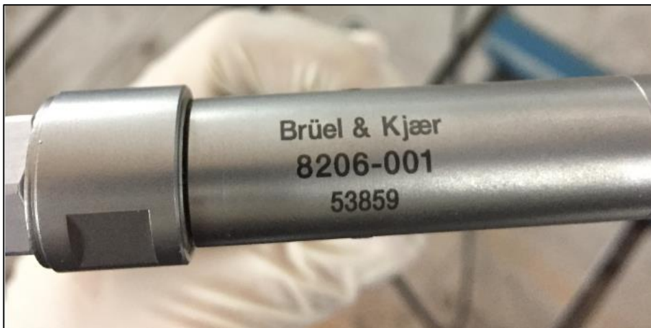
Figure 3-16: The impact hammer (calibration is valid until 26.01.2022)
