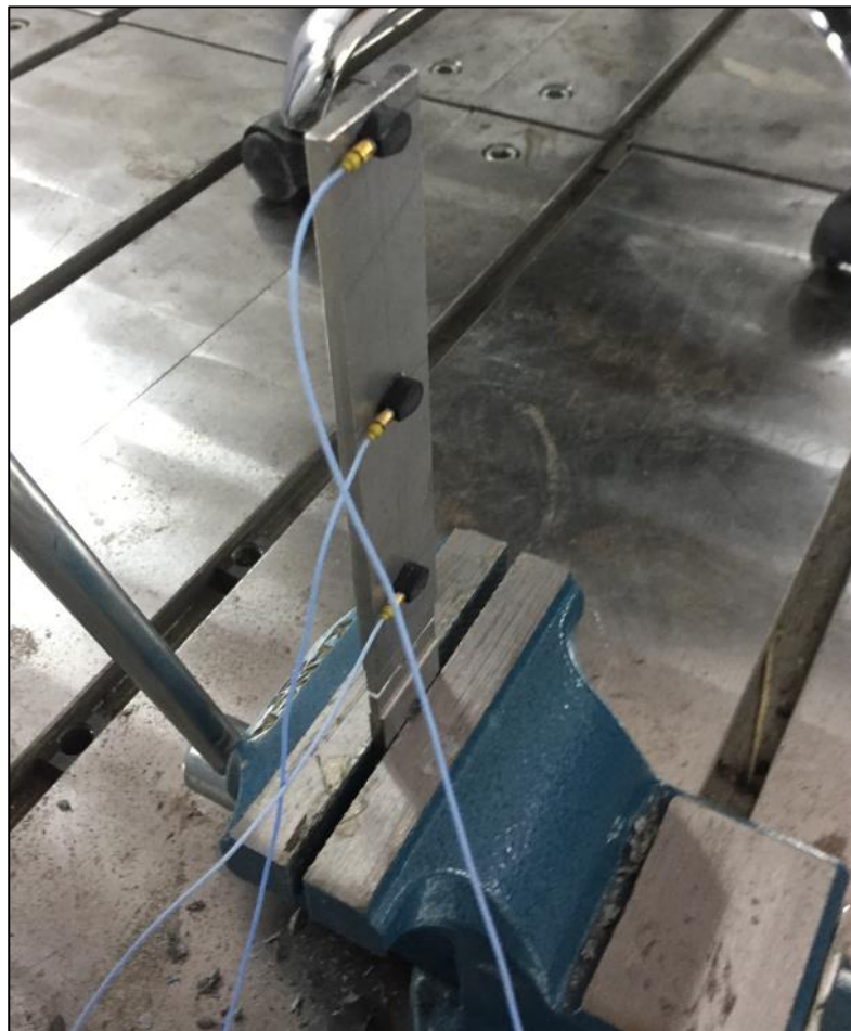
Figure 3-14: The modal test setup
