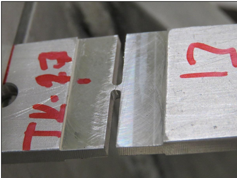
Figure 4-19: Steel notched beam with crack - Sample 4
