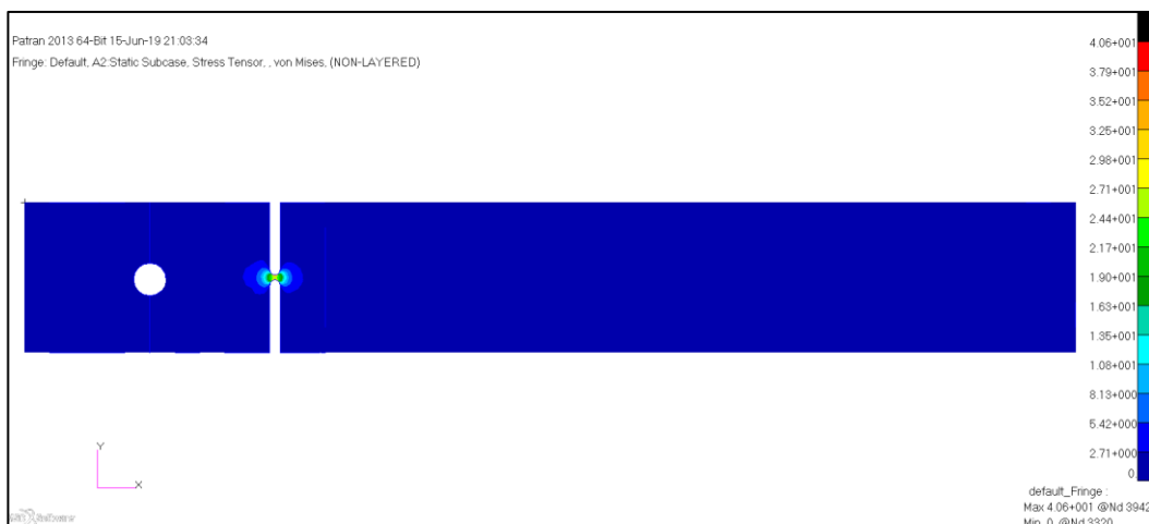
Figure 3-7: The von Mises stress distribution of the notched beam with mesh number 7
