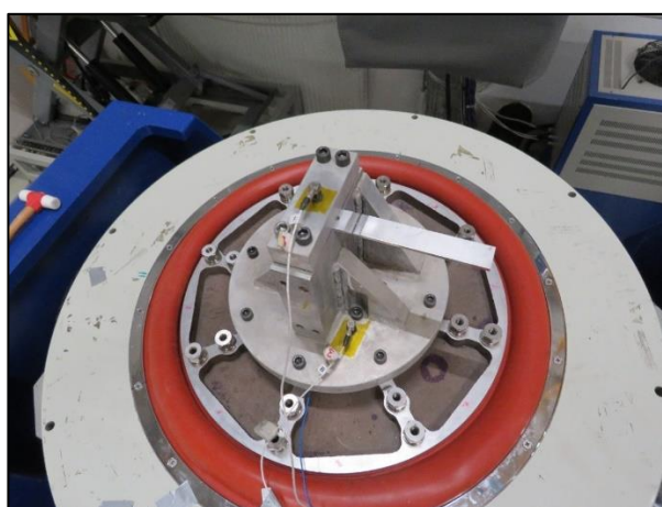
Figure 3-34: Test setup of the aluminum notched beam
