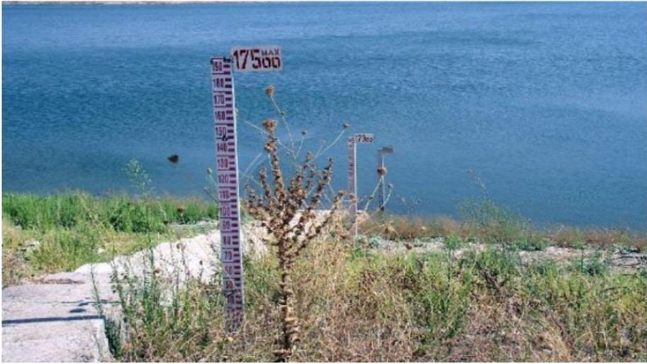
Figure 2.7. Staff gauge used in Lake level measurements (Sapcilar & Fakioglu, 2004)
