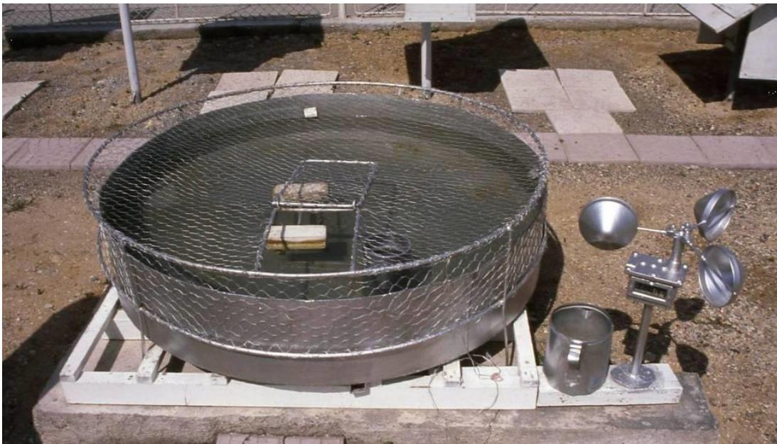
Figure 2.4. *Evaporation Pond (Instruments and Devices Used in Meteorology, 2019)*
