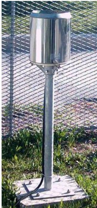
Figure 2.3. *Precipitation Meter (Instruments and Devices Used in Meteorology, 2019)*
