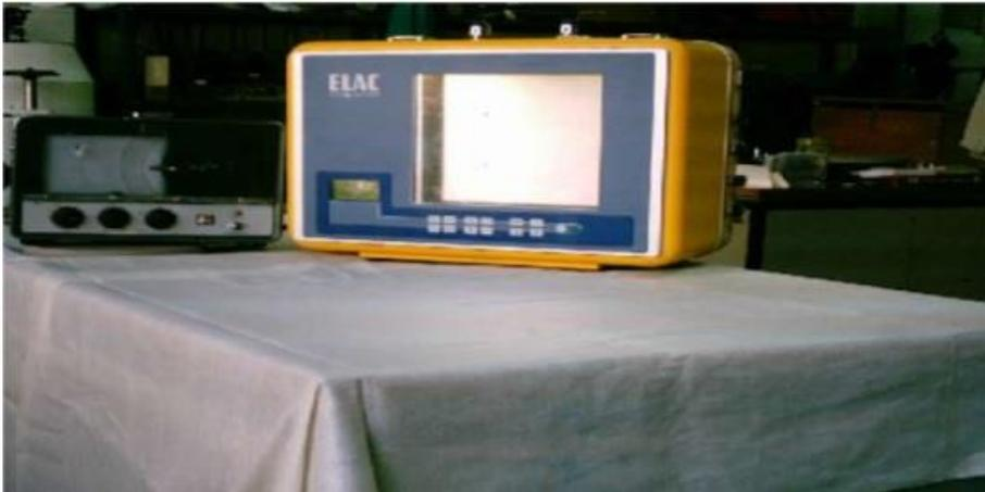
Figure 2.6. *Echo Sounder used for depth measurement (Sapcilar & Fakioglu, 2004)*
