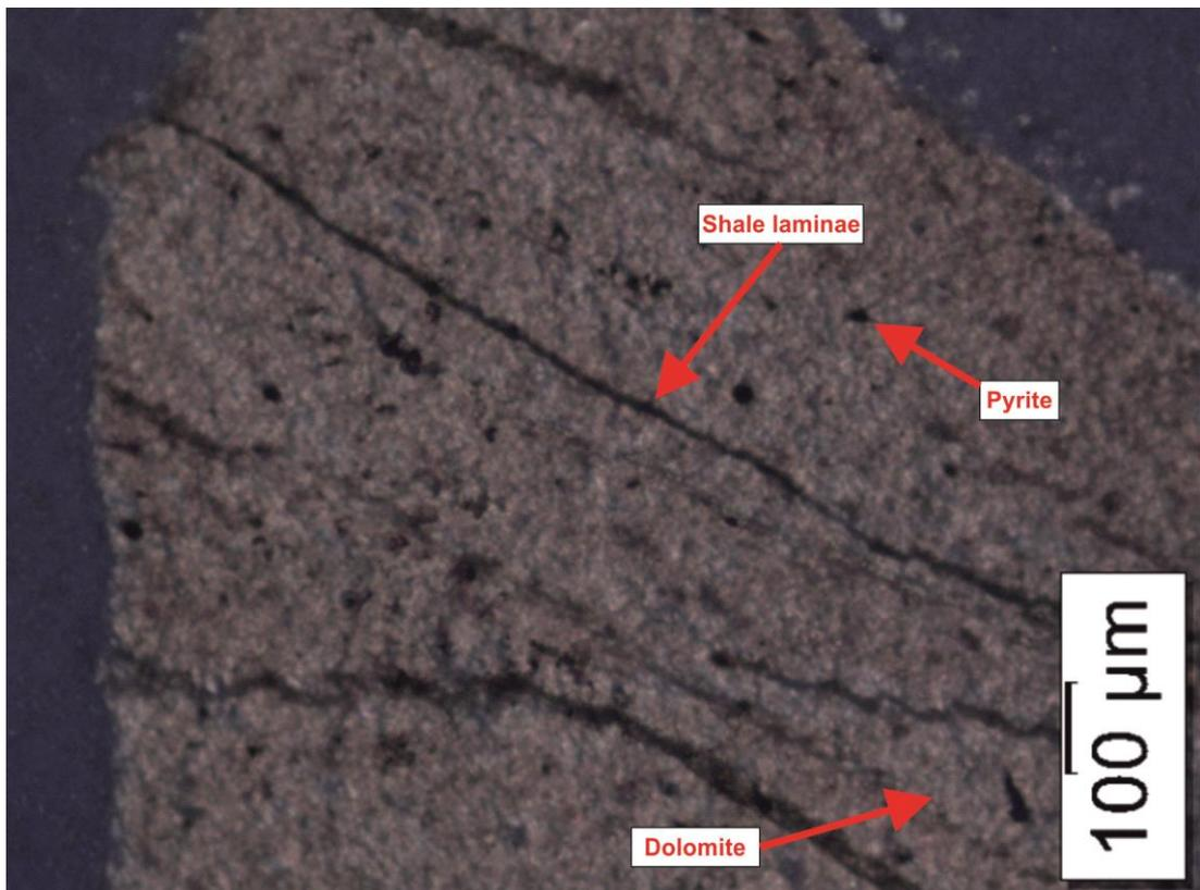
Figure 35: The photomicrograph of the marl lithofacies, the cutting sample-1 of the 2<sup>nd</sup> sandstone level of the uppermost Bedinan Formation, F well.
