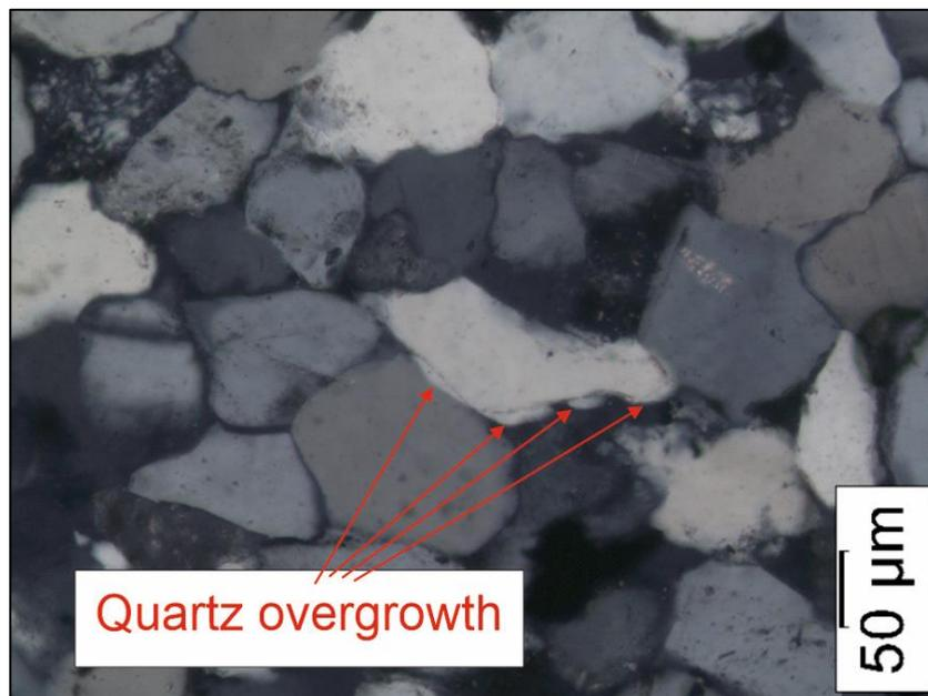
Figure 79: Photomicrograph of the quartz overgrowth developed around tightly packed fine grained quartz of the 1<sup>st</sup> sandstone level (Core-2) of the uppermost Bedinan Formation in F well.
