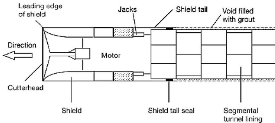
Figure 2.3. Typical Longitudinal Section of Tunnel Shield (Chapman et al., 2010)
