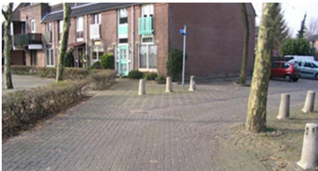
*Figure 4.22. Use of textured pavement, trees and bollards to guide traffic*
