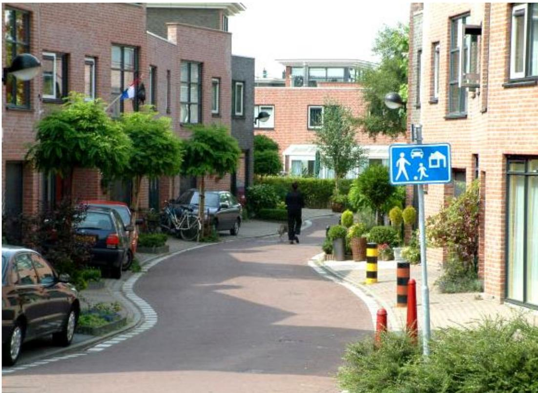
Figure 2.10. Name unknown Woonerf street; entrance sign, uneven street line, street trees, bollards, on-street parking (resource: <https://i.pinimg.com/originals/55/1e/13/551e13ed58f28832fd3bb424c0878396.jpg> )
