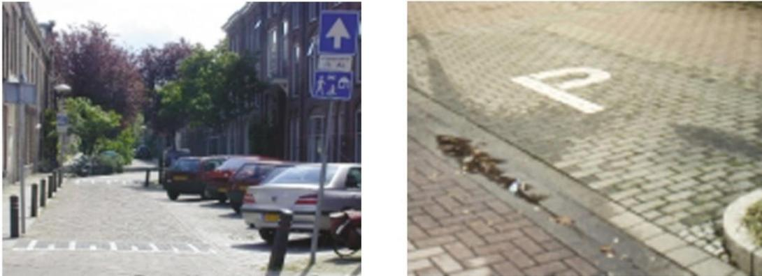
Figure 2.19. Planters and street furniture help prevent indiscriminate parking. & The Dutch “P” for a parking space. (Institute of Highway Incorporated Engineers, 2002, 36)
