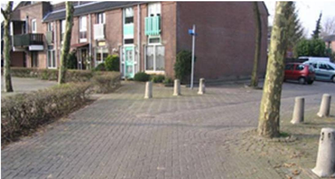
*Figure 4.22. Use of textured pavement, trees and bollards to guide traffic*
