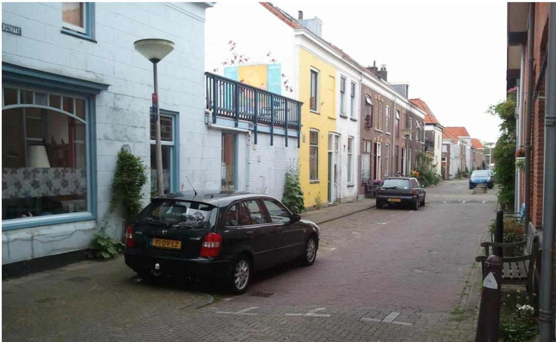
Figure 2.6. First Woonerf implemented according to web sources; seating element for pedestrians, speed humps, significant paving materials, pedestrian level lighting, uneven street line (<http://portlandtransitauthority.blogspot.com.tr/2012/07/a-visit-to-first-woonerf.html>)
