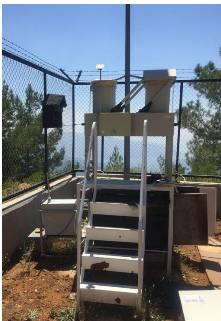
Figure 3.2 Precipitation Sampler of Marmaris Station
