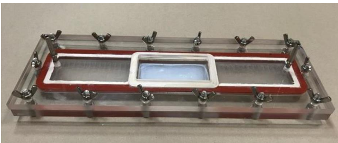
Figure C.1: Plexiglass NO x Photoreactor used in the NO Oxidation Experiment
