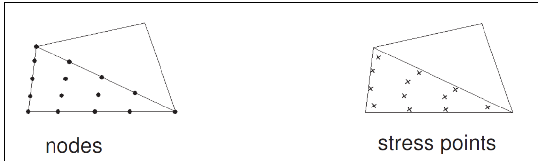
Figure 2.4 Example of nodes and stress points positions in mesh element (PLAXIS 2D Reference Manual, 2016)
