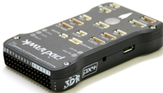
Figure 6.6: A view of Pixhawk autopilot card [2].
