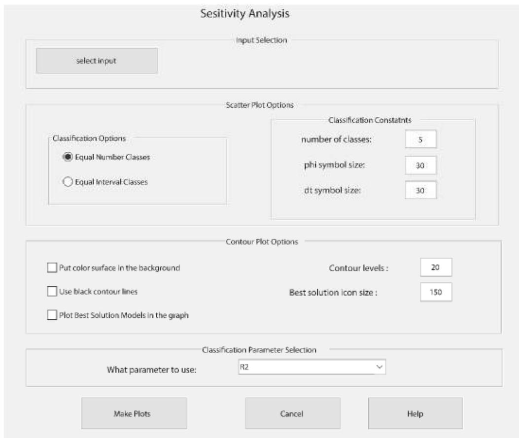
Figure 4-6: Sensitivity analysis interface which generates scatter and contour plots of best solutions in model space using the selected parameter values
