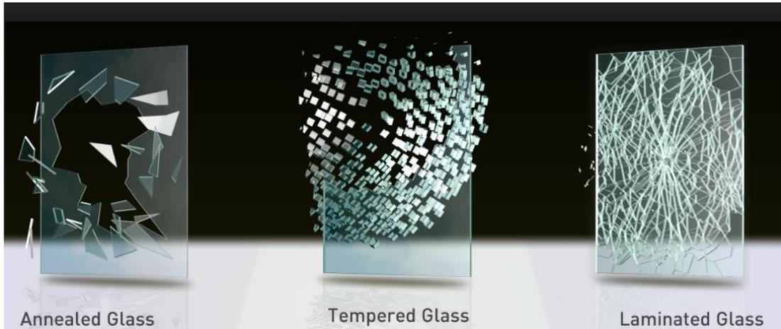
*Figure 6: Typical fracture shape of float, tempered and laminated glass<sup>7</sup>*
