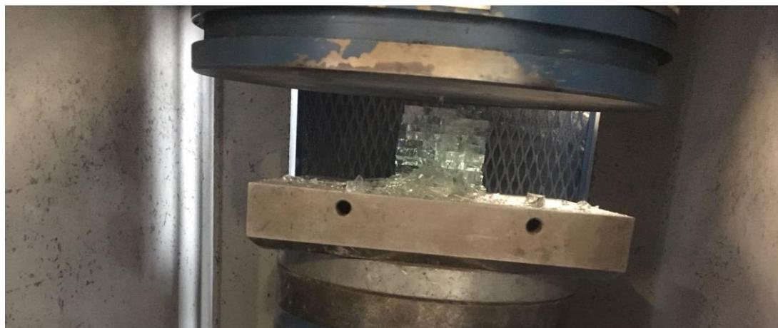
*Figure 13: A glass cube premature failure in the compression test*
