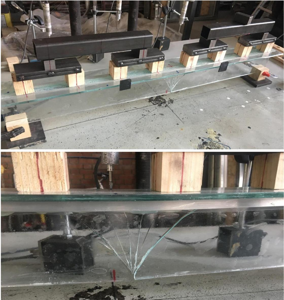
*Figure 37: T-beam float glass exposed to its ultimate load*
