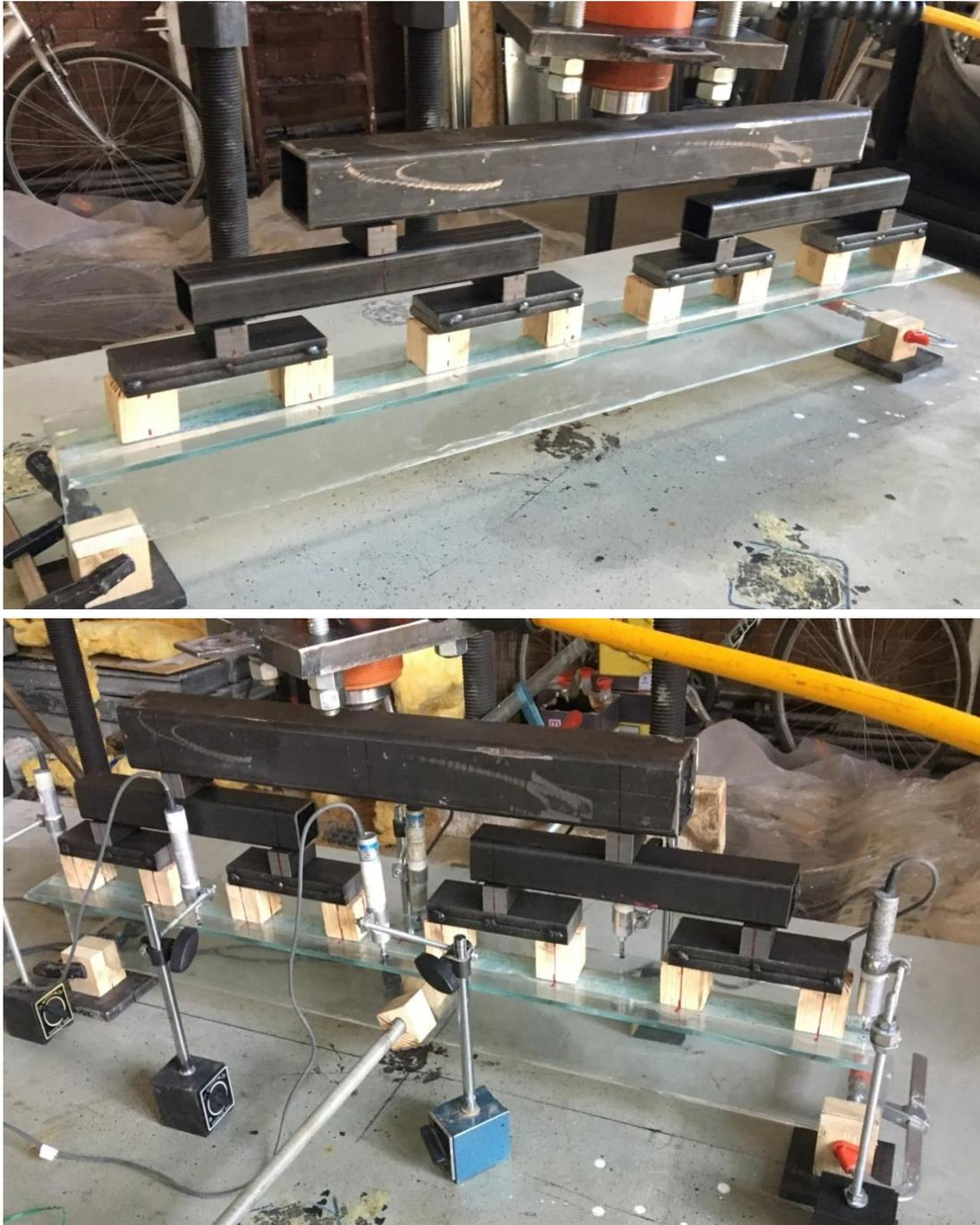
*Figure 35: Test set-up of T-beam without post tensioning*
