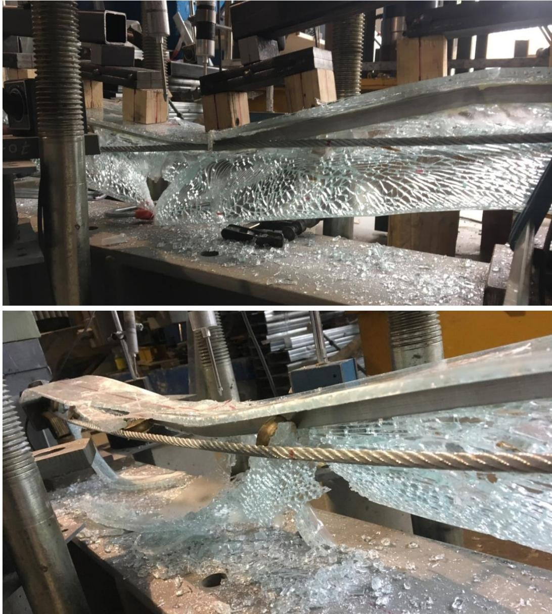
*Figure 43: Tempered glass T-beam with post tensioning after fracture.*
