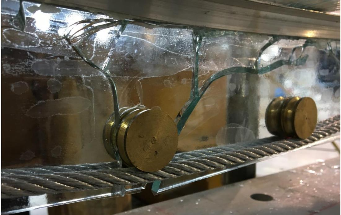
*Figure 41: First cracks of float glass T-beam with post tensioning*
