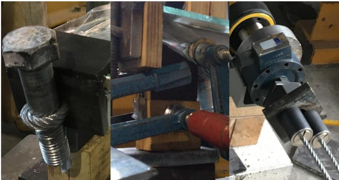
*Figure 33: Anchorages at the ends of the beams (Tensioning at right side).*
