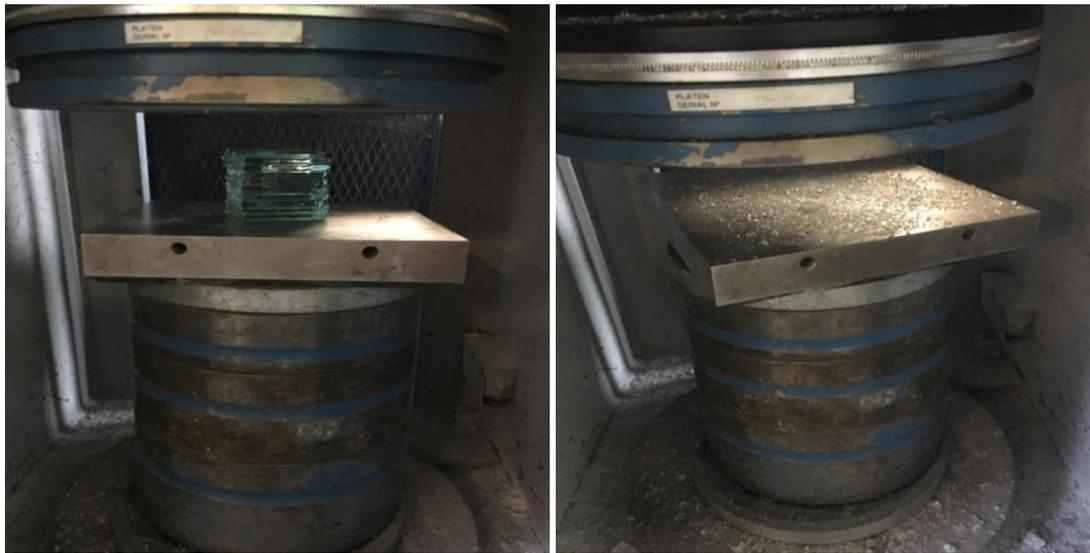
*Figure 12: A glass cube before and after the compression test*
