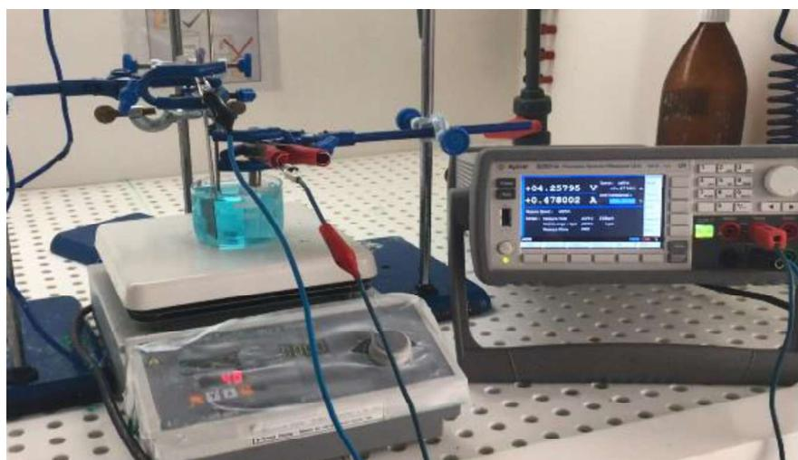
Figure 3.5. A picture of experimental set-up used in the recycling of diamond embedded copper-tin matrix cutting tools
