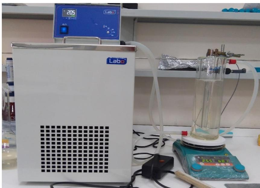
Figure 3.1. Experimental Set-up used for Fenton Oxidation
