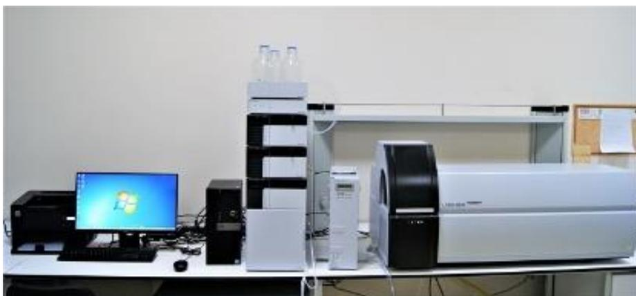
Figure 3.4 LC/MS/MS device
