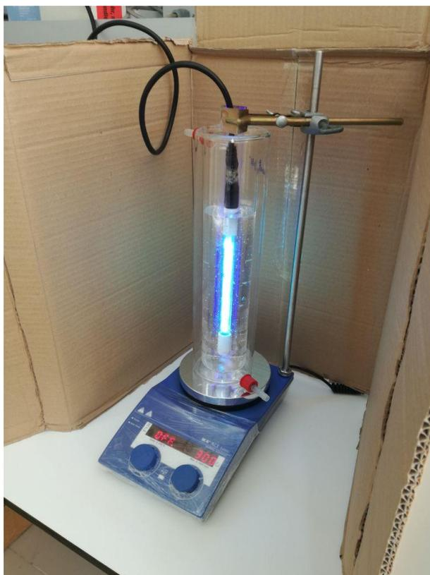
Figure 3.2. Experimental set-up used for Photo-Fenton and UV/ H<sub>2</sub>O<sub>2</sub> Oxidation
