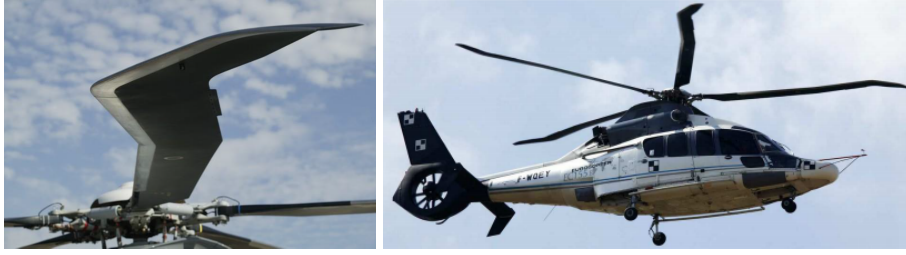
Figure 1.7: EC155 with the Eurocopter Blue-Edge TM blade [3]
