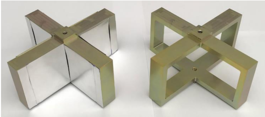
Figure 6-63 T2 test prototypes, with and without damping application
