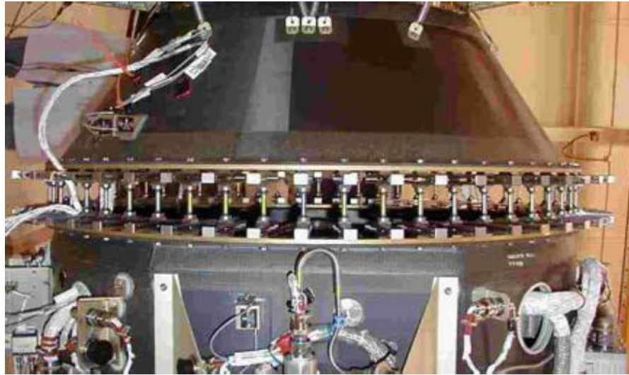
Figure 2-14 SoftRide MultiFlex installation [29]
