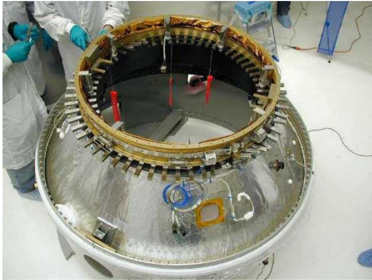
Figure 2-10 SoftRide UniFlex installation [29]
