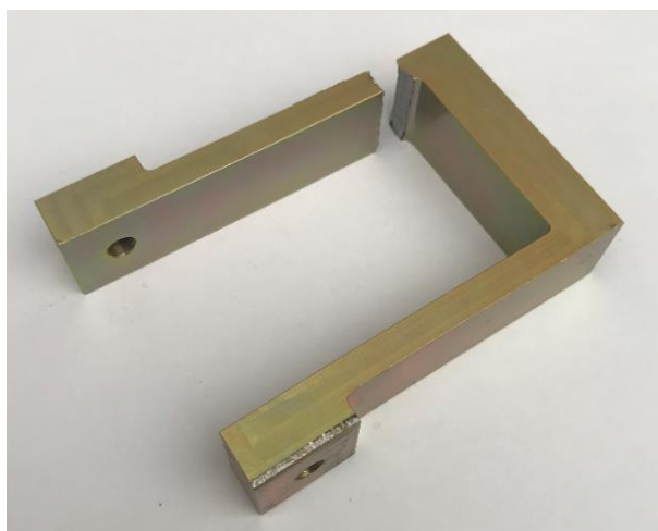
Figure 6-62 Broken T1 vibration isolator
