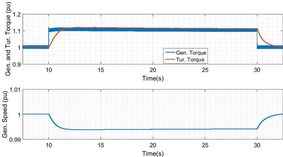
Figure 4.14: Generator and Turbine Torques and Generator Speeds for High Wind Scenario for 20 Seconds Support
