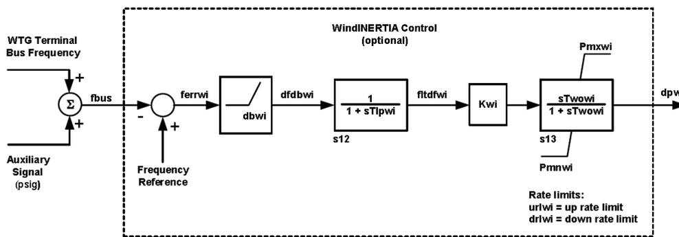
Figure 1.7: GE WindINERTIA Control Diagram in [26]
