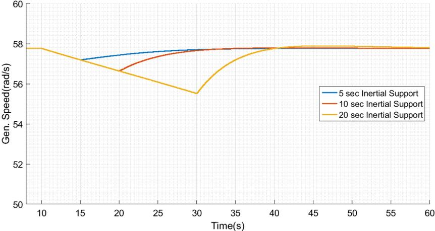
Figure 4.18: Generator Speeds of the Wind Turbine for Low Wind Scenario
