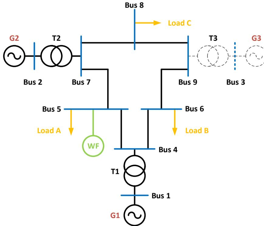
Figure 5.7: Reduced Inertia Case Single Line Diagram
