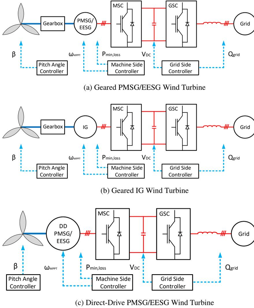
Figure 3.1: Wind Turbine Topologies with Full-Scale Power Converter
