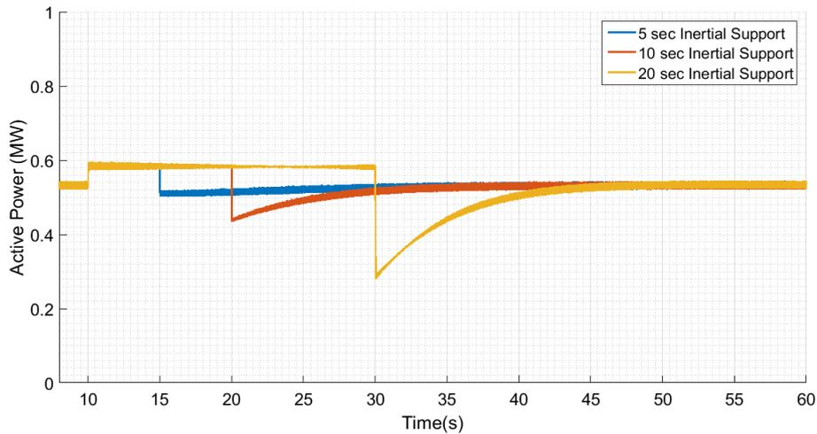
Figure 4.22: Active Power Output of the Wind Turbine for Medium Wind Scenario
