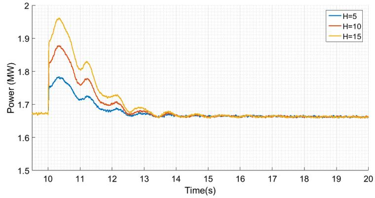
(a) Active Power Generations of the Wind Farms (wind speed=9m/s and n=1490rpm)
