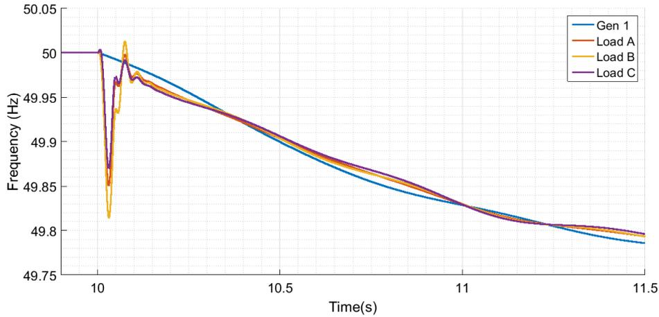
Figure 5.4: Frequencies in Generator 1 and Load Buses
