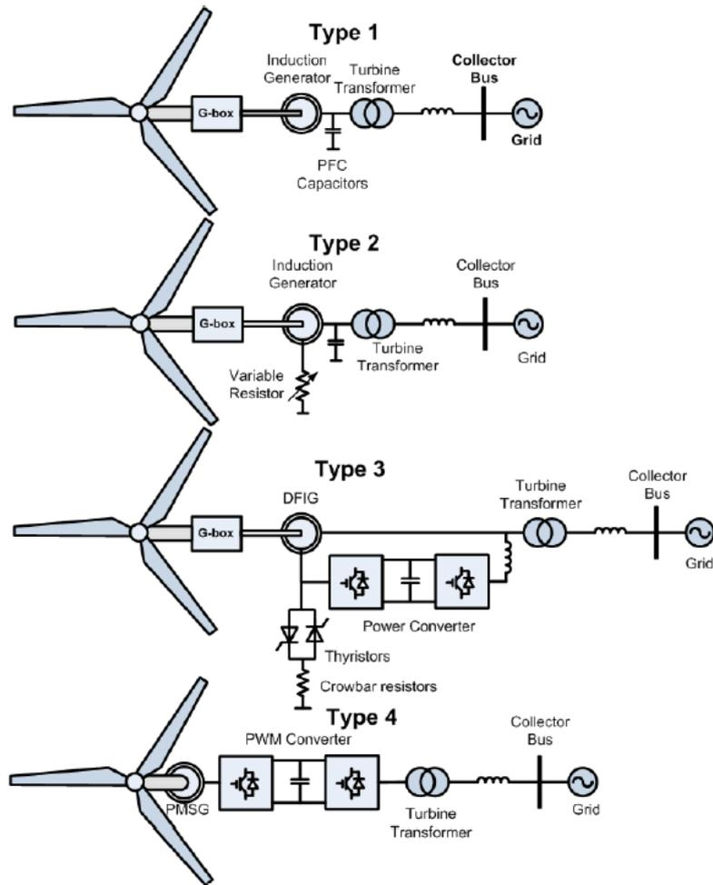
Figure 1.4: Wind Turbine Generator Configurations [12]
