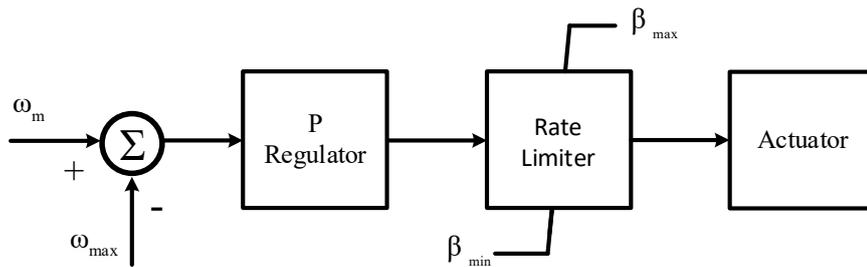
Figure 3.4: Pitch Angle Control Diagram
