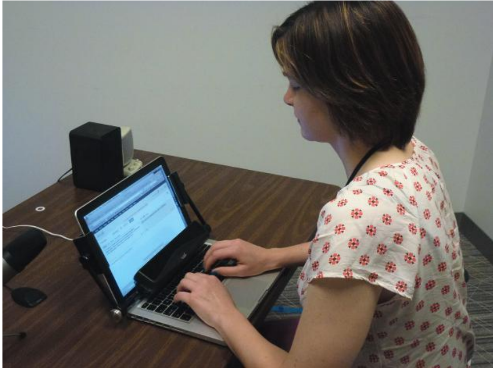
Figure 2. A participant using a mobile eye tracker mounted on a laptop. (Bergstrom & Schall, 2014)
