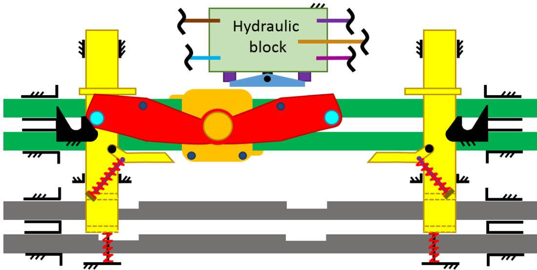
**Figure 100** Contact position of rocker roller with the locking recess
