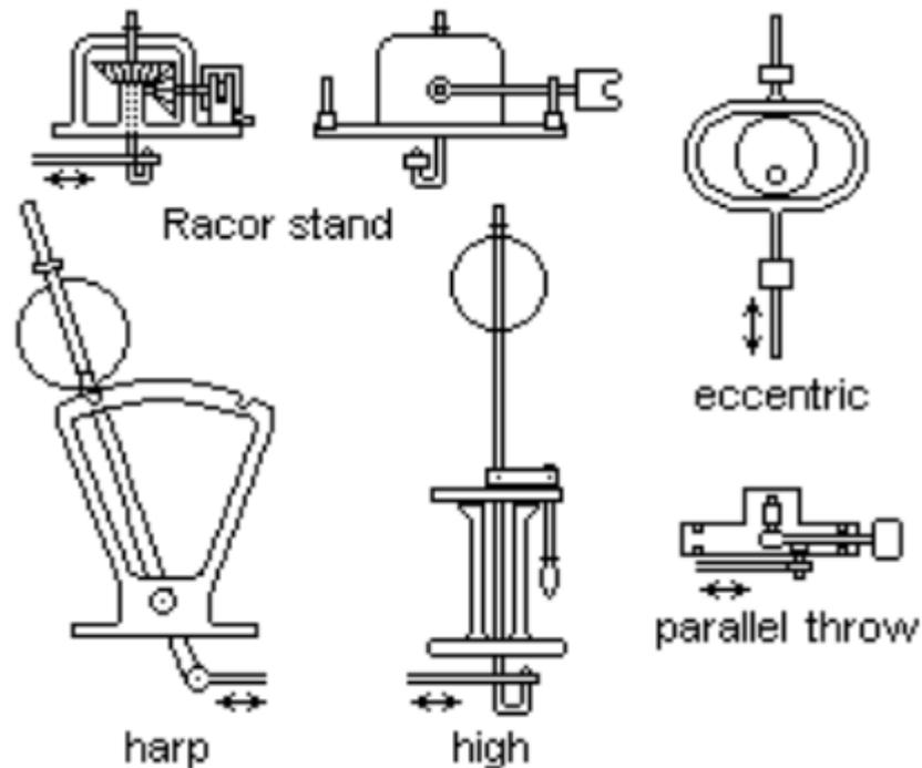
**Figure 5** Schematic views of different switch stand designs [3]
