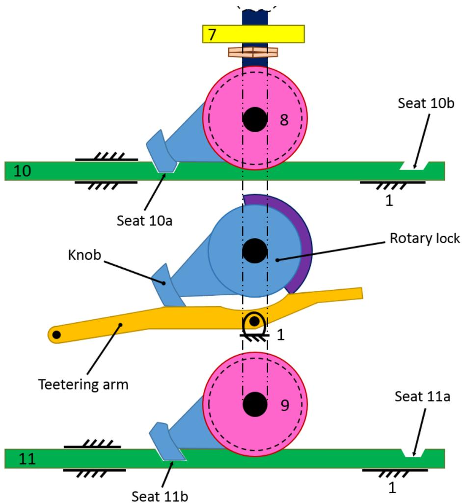
**Figure 130** Representative schematic model of locking mechanism together with the driving mechanism from side view
