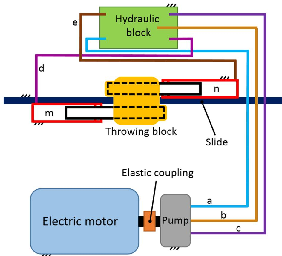
**Figure 84** Schematic representation of electro-hydraulic driving unit from top view
