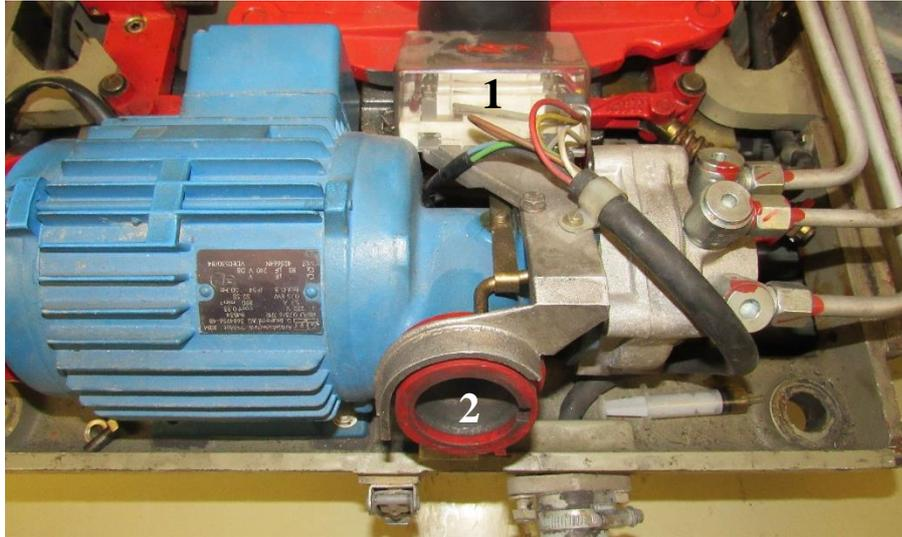
**Figure 107** Energy cut-off switches (1) and access hole (2) for the manual operation
