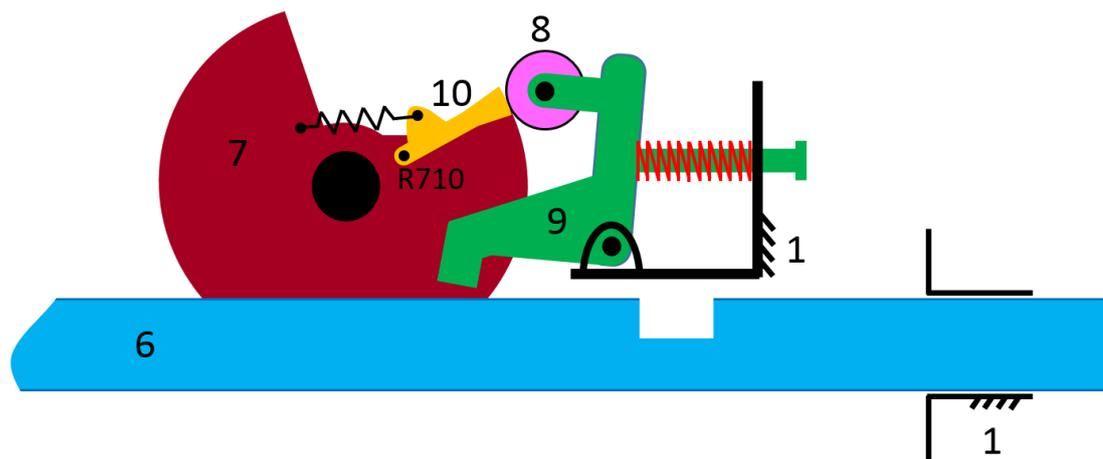
**Figure 79** Schematic representation of locking delay
