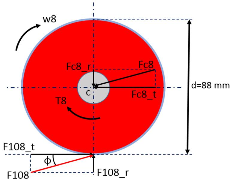
**Figure 120** Free body diagram of the gear 8
