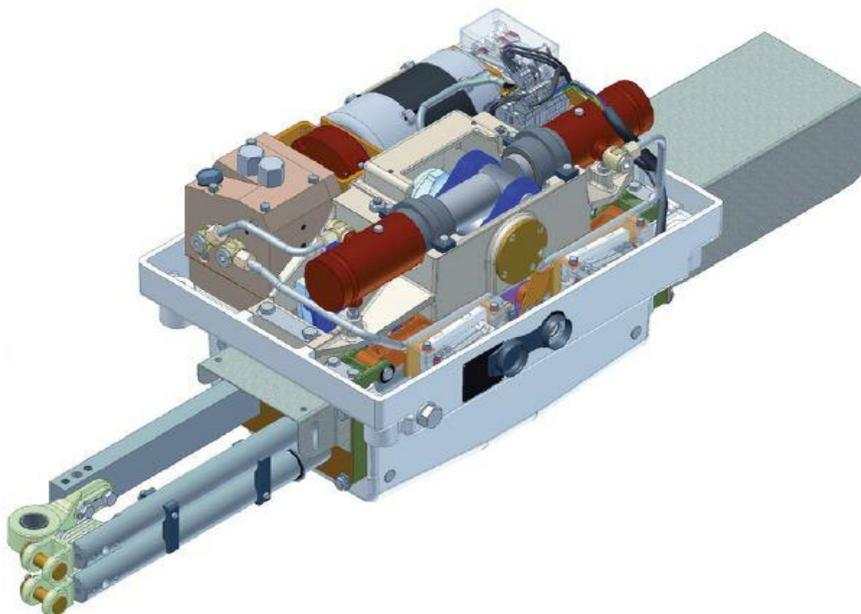
**Figure 32** Inside view of the FieldTrac 6343 L826H point machine [22]
