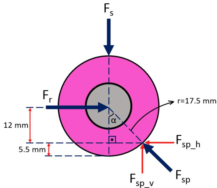
**Figure 114** Free body diagram of trailing cylinder at the beginning of trailing
