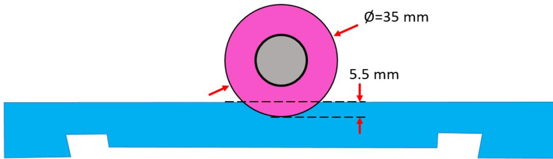
**Figure 113** Mating of trailing cylinder into shutter plate seat
