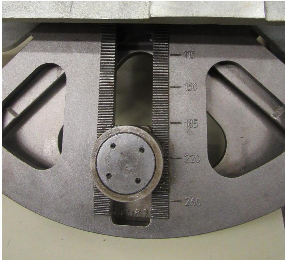
**Figure 39** Photograph of scaling numbers on the rotating disc to adjust the stroke
