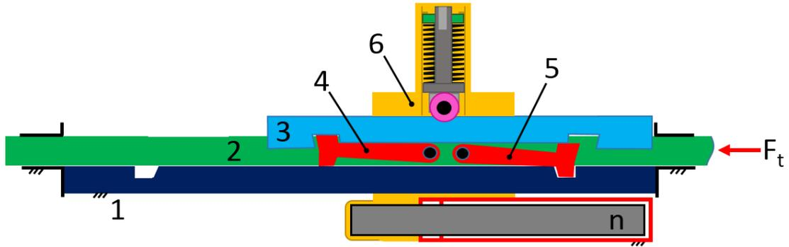
**Figure 112** Trailing force acting on the driving rods
