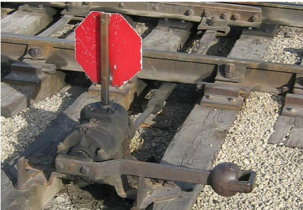
**Figure 4** Photograph of an old switch stand with a reflector target on top [2]
