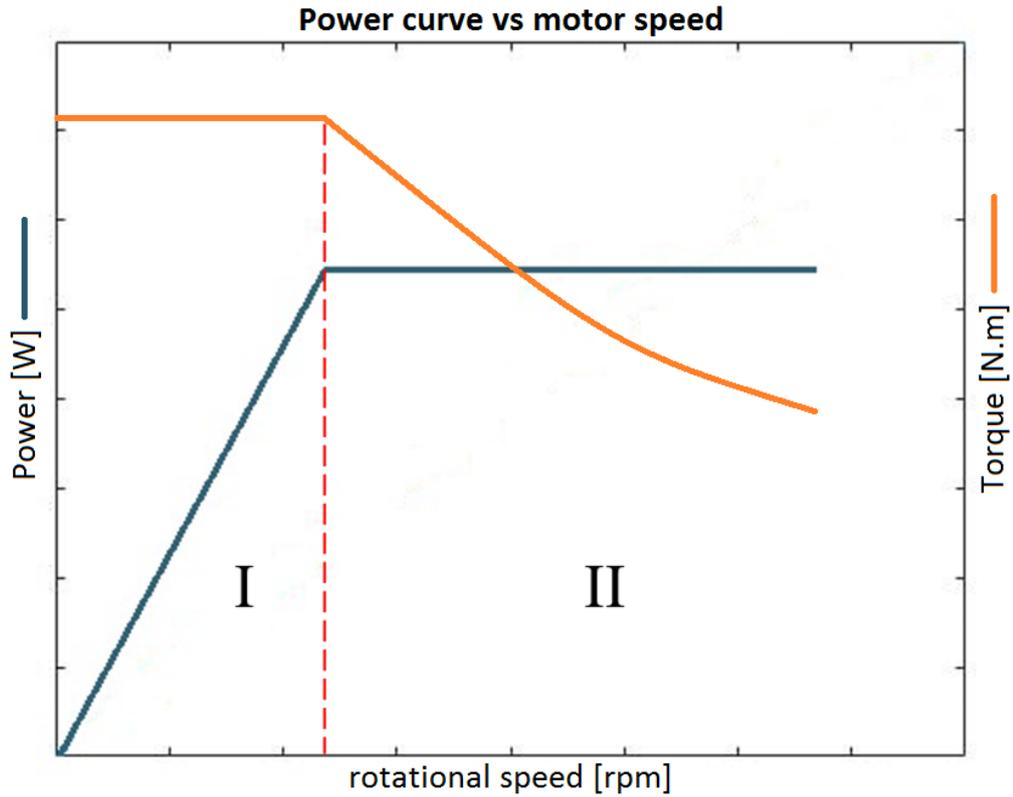
**Figure 68** Typical power and torque curve of a DC electric motor
