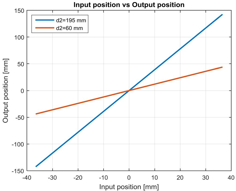
**Figure 48** Output position of driving rod with respect to input position
