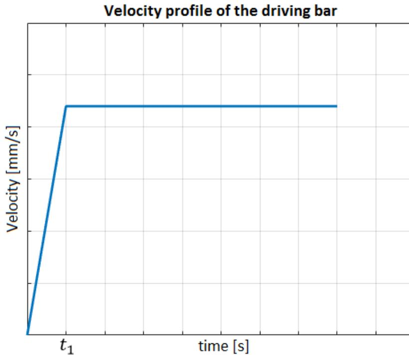
**Figure 69** Assumed velocity profile of the driving bar during its throwing motion
