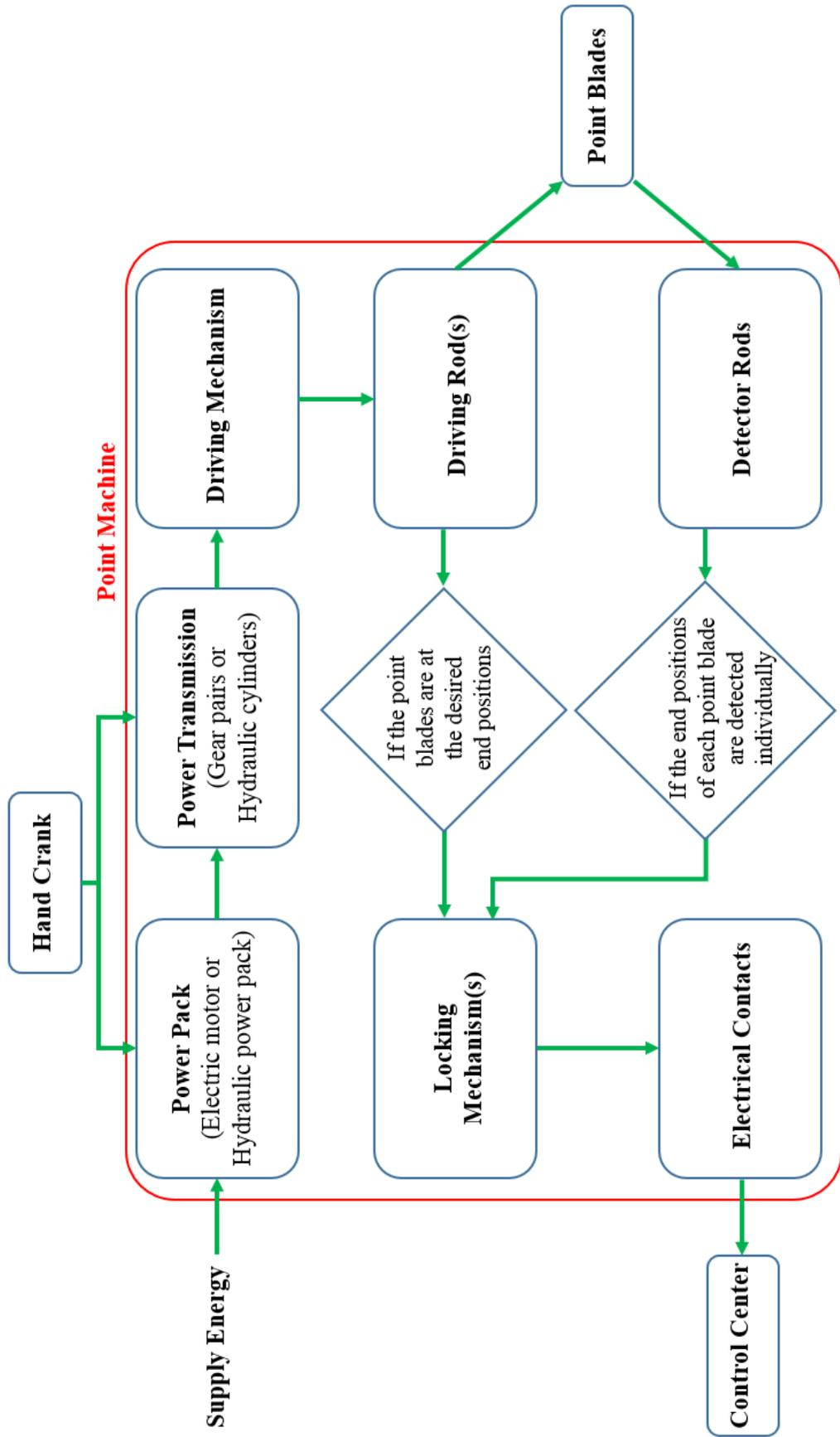
Figure 11 Fundamental structure of a modern point machine
