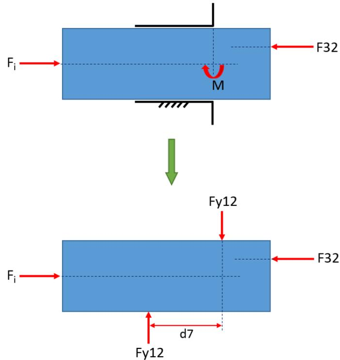
**Figure 44** Free body diagram of link 2
