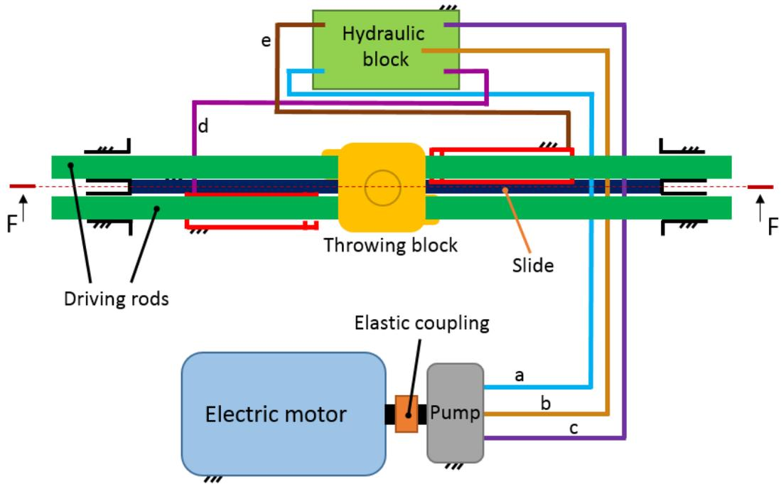
**Figure 85** Schematic representation of installation of driving rods from top view
