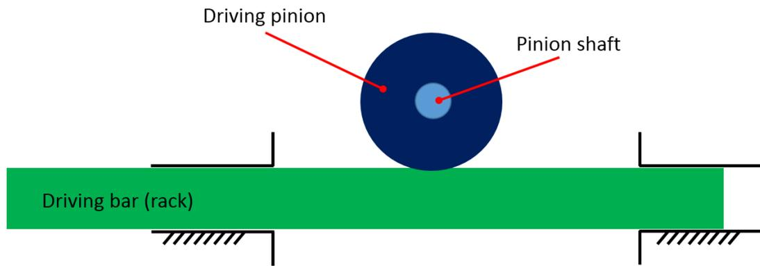
**Figure 64** Rack and pinion gear mate in front view
