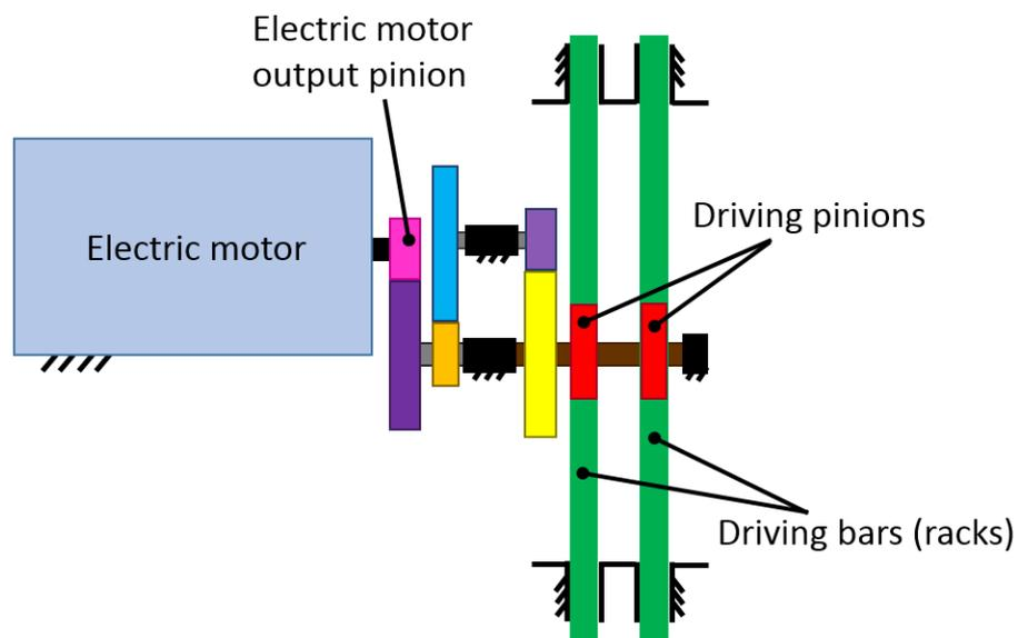
**Figure 116** Representative schematic model of driving mechanism from top view
