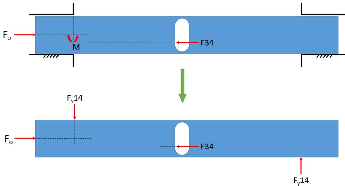
**Figure 46** Free body diagram of link 4
