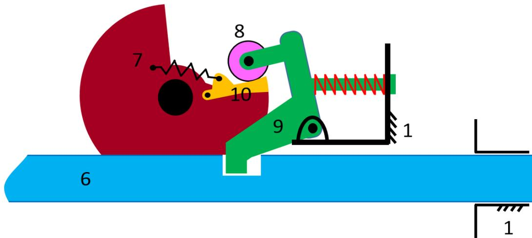
**Figure 80** Schematic representation of locked position with a tight engagement
