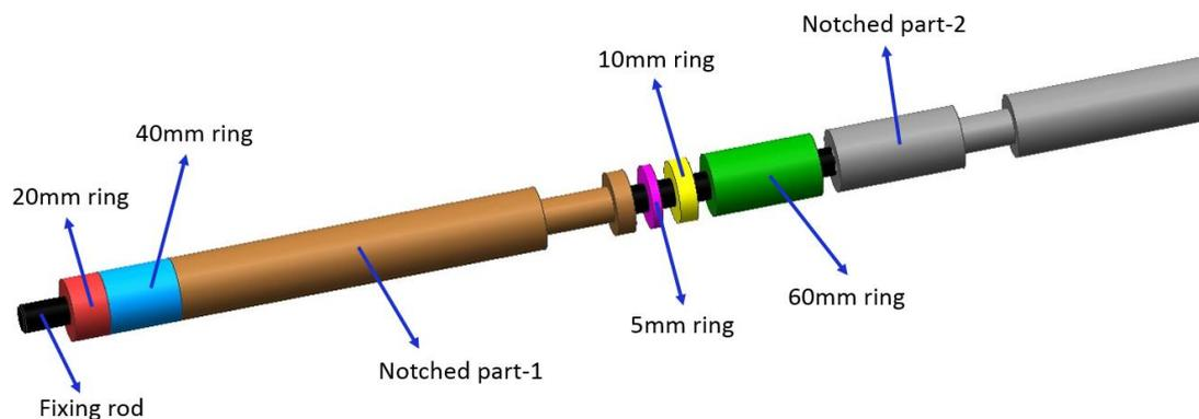
**Figure 54** The detector rod adjusted for the 115 mm motion of point blades
