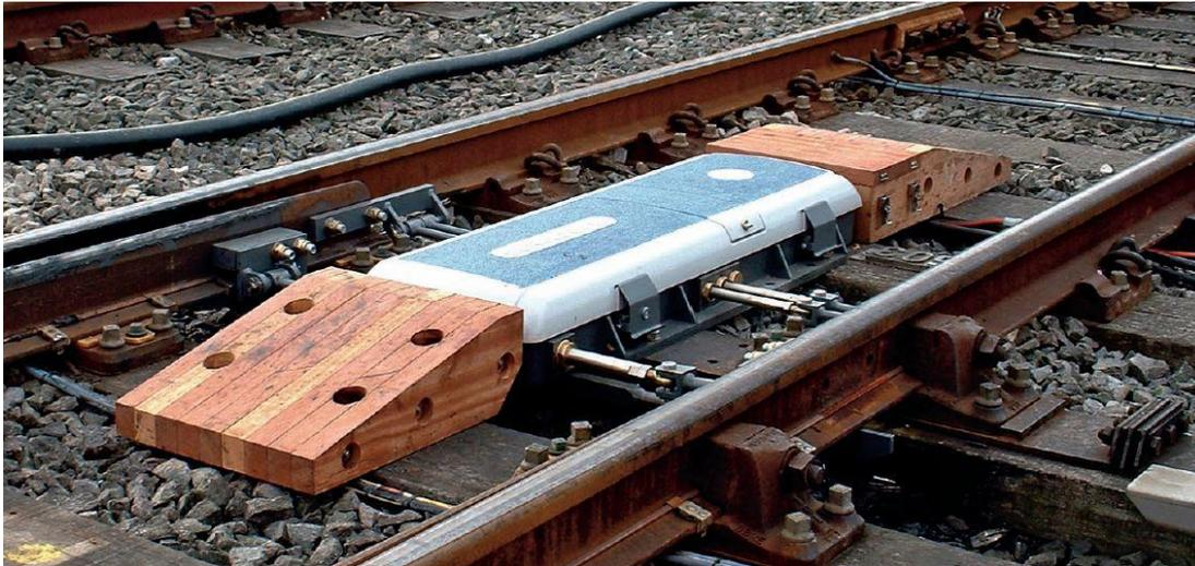
**Figure 16** Switchguard Surelock point machine mounted between the rails (the wooden wedges protect the machine from a derailed wheel) [14]
