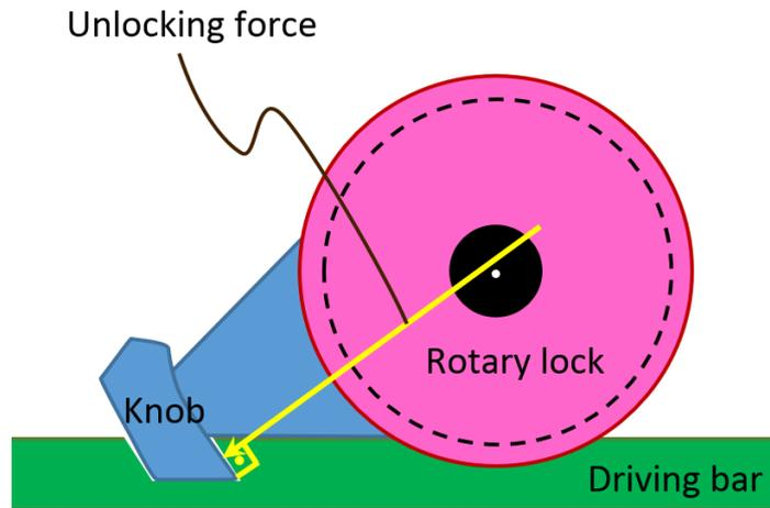
**Figure 131** Geometrical constraint for the locking of driving bars
