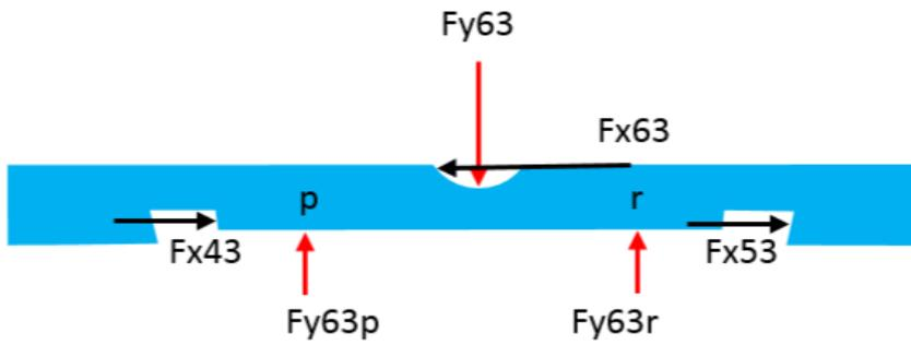
**Figure 88** Free body diagram of shutter plate
