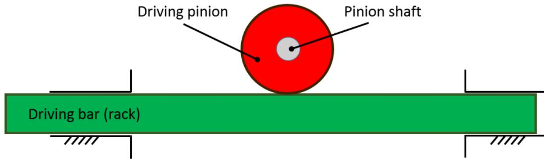
**Figure 119** One of the rack and pinion gear mates from side view
