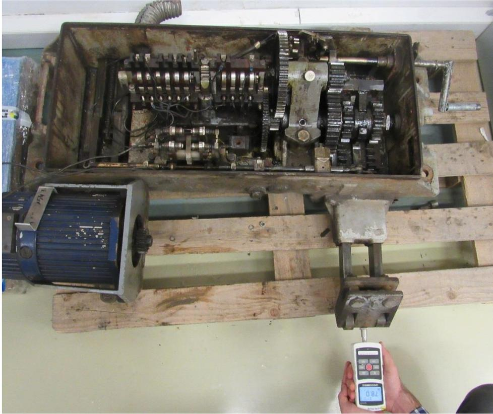
**Figure 128** Force measurement at the linear slide of point machine D
