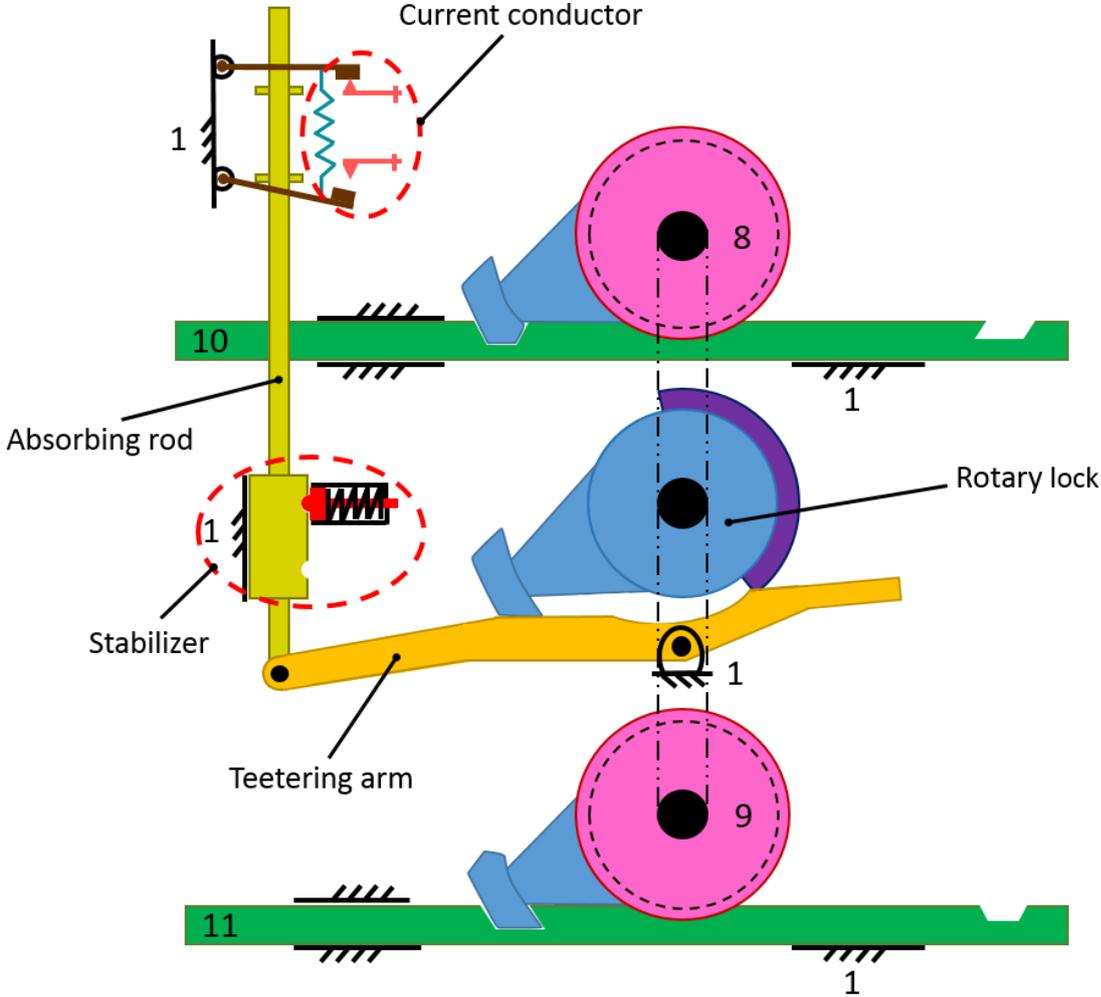
**Figure 132** Schematic representation of current conductor and stabilizer
