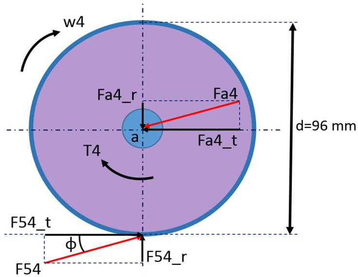
**Figure 65** Free body diagram of link 4
