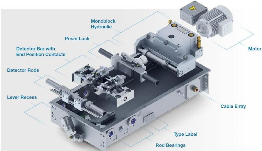
**Figure 19** Modular design structure of the Unistar CSV 24 [16]
