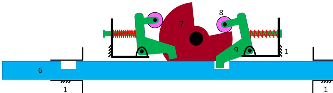
**Figure 78** Schematic representation of locked position of the machine
