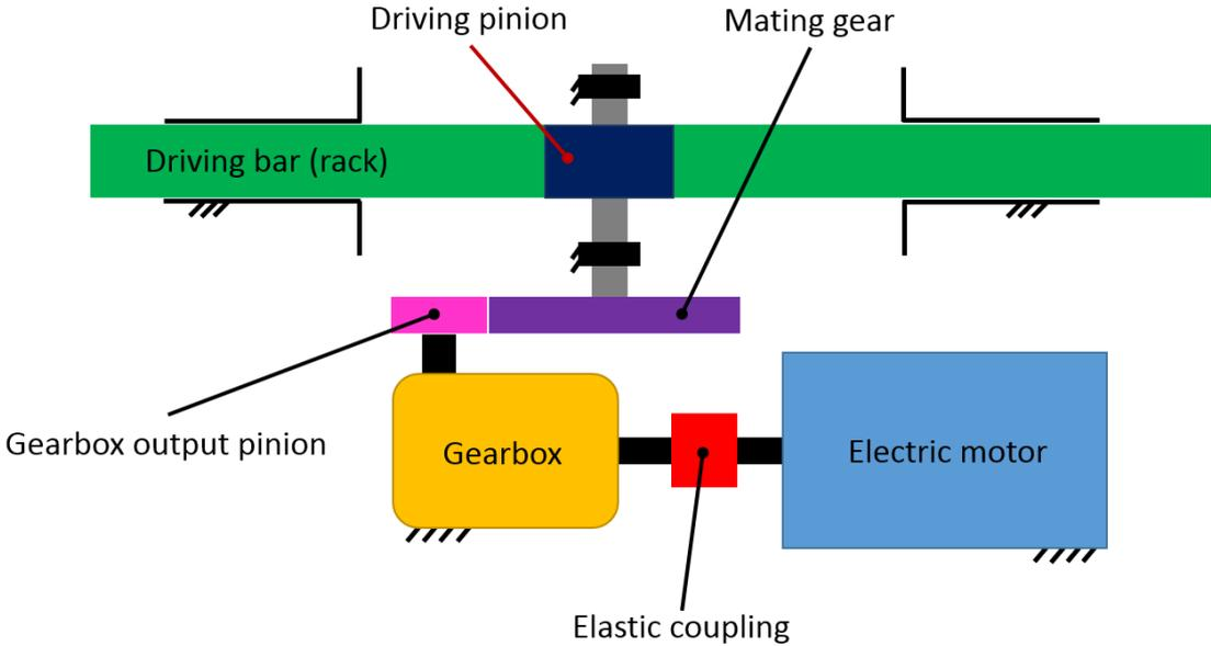
**Figure 61** Representative schematic model of driving mechanism from top view
