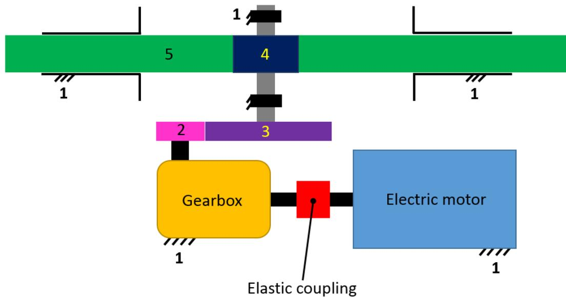
**Figure 62** Representative schematic model showing the links of driving mechanism
