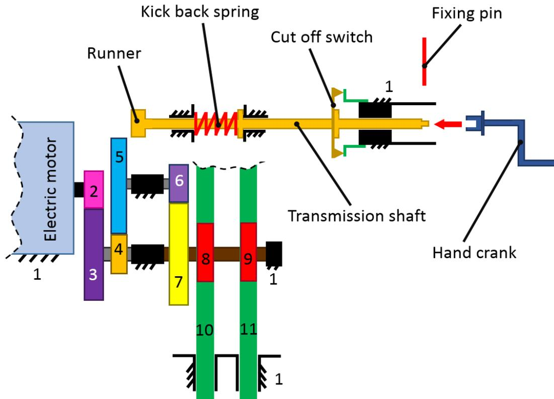
**Figure 138** Schematic representation of manual operation assembly
