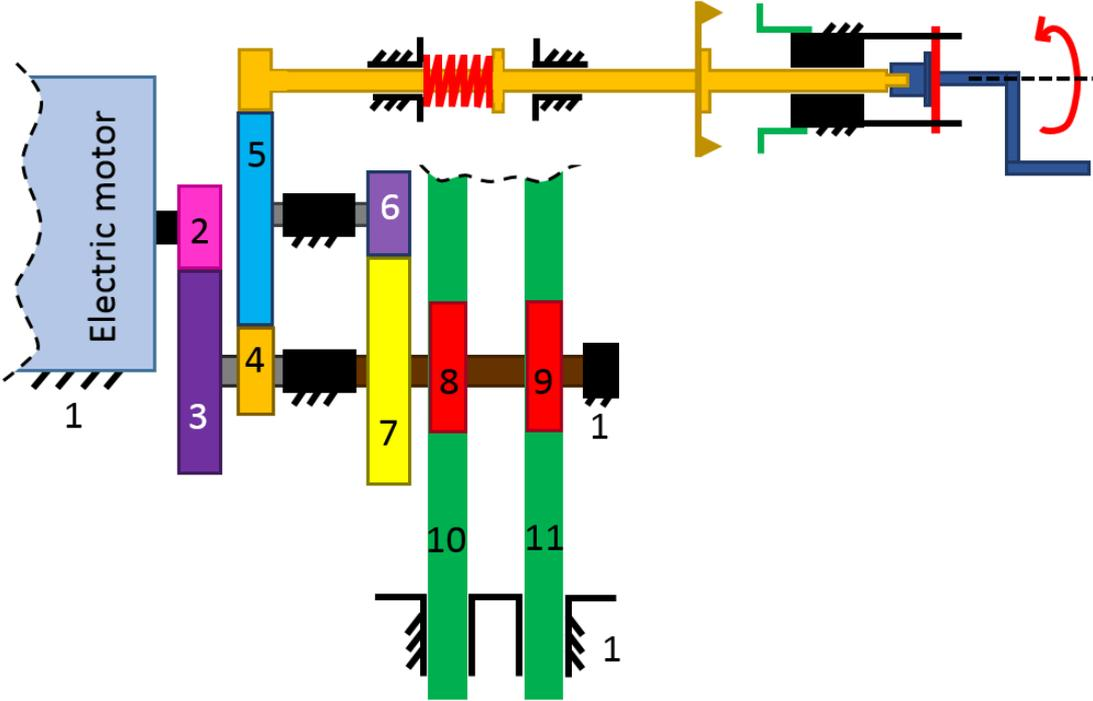
**Figure 139** Schematic representation of use of hand crank
