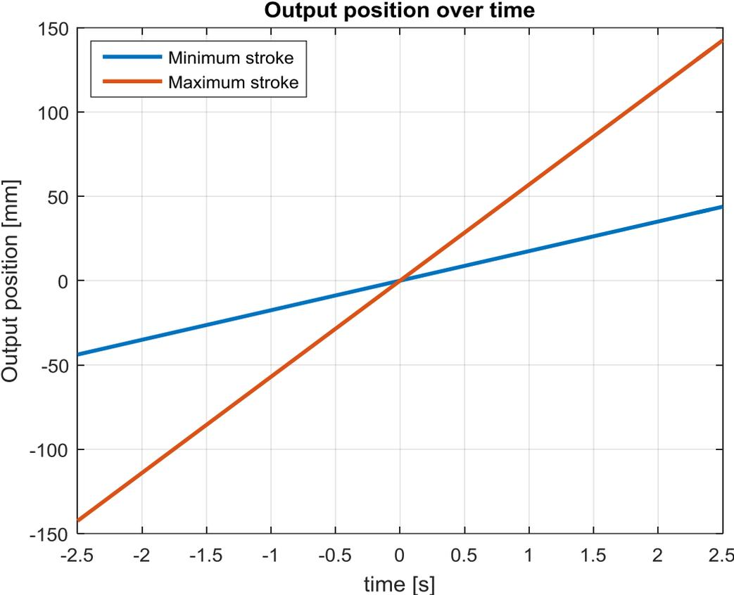
**Figure 47** Maximum and minimum throwing strokes of Point Machine A
