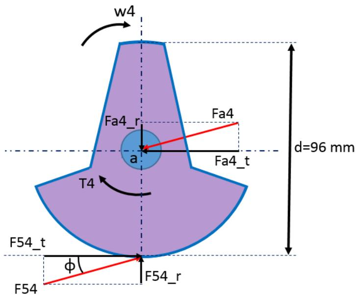
**Figure 66** Free body diagram of actual shape of link 4
