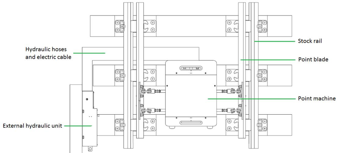
**Figure 25** Schematic view of Easydrive-i installation [18]
