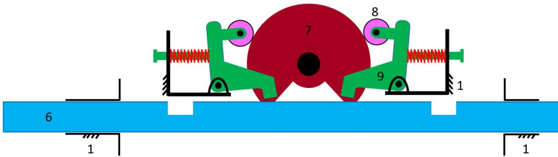
**Figure 77** Schematic representation of the locking mechanism in front view
