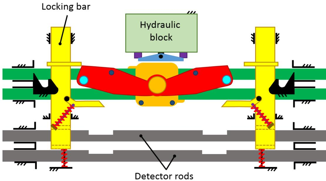
**Figure 97** Schematic representation of whole locking mechanism
