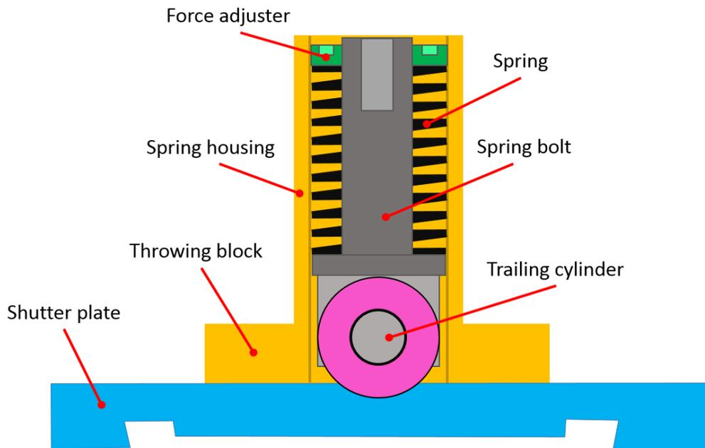
**Figure 111** Components of retaining assembly
