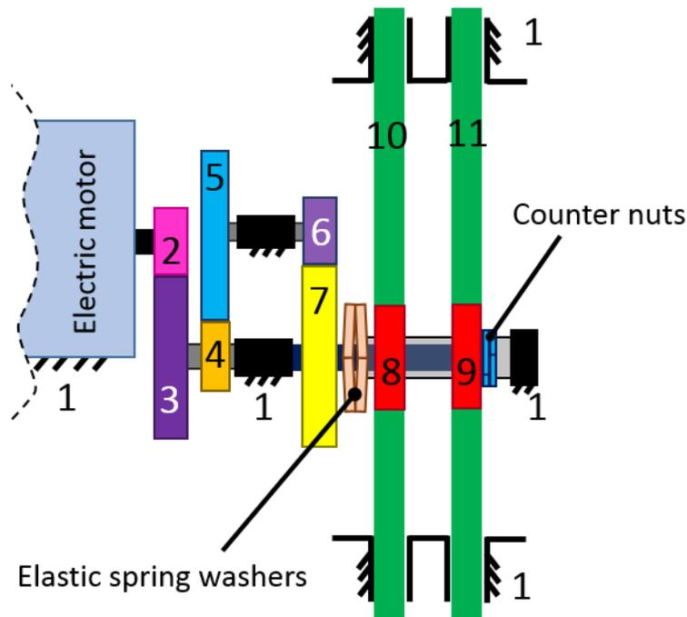
**Figure 129** Schematic representation of elastic spring washers (clutch)
