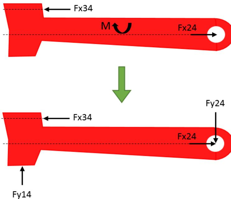
**Figure 89** Free body diagram of left locking clamp
