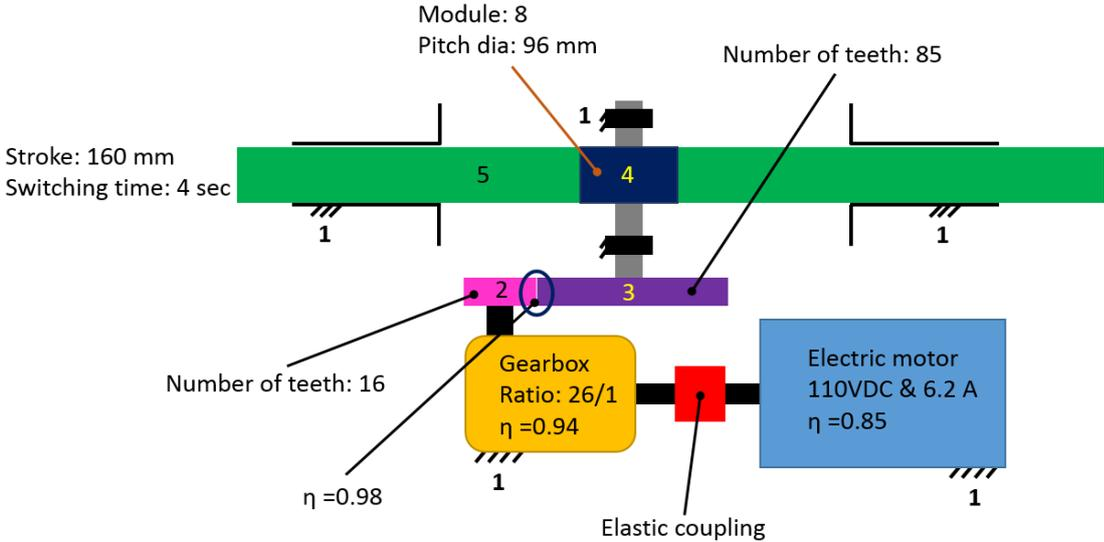
**Figure 63** Known and measured parameters of the driving mechanism
