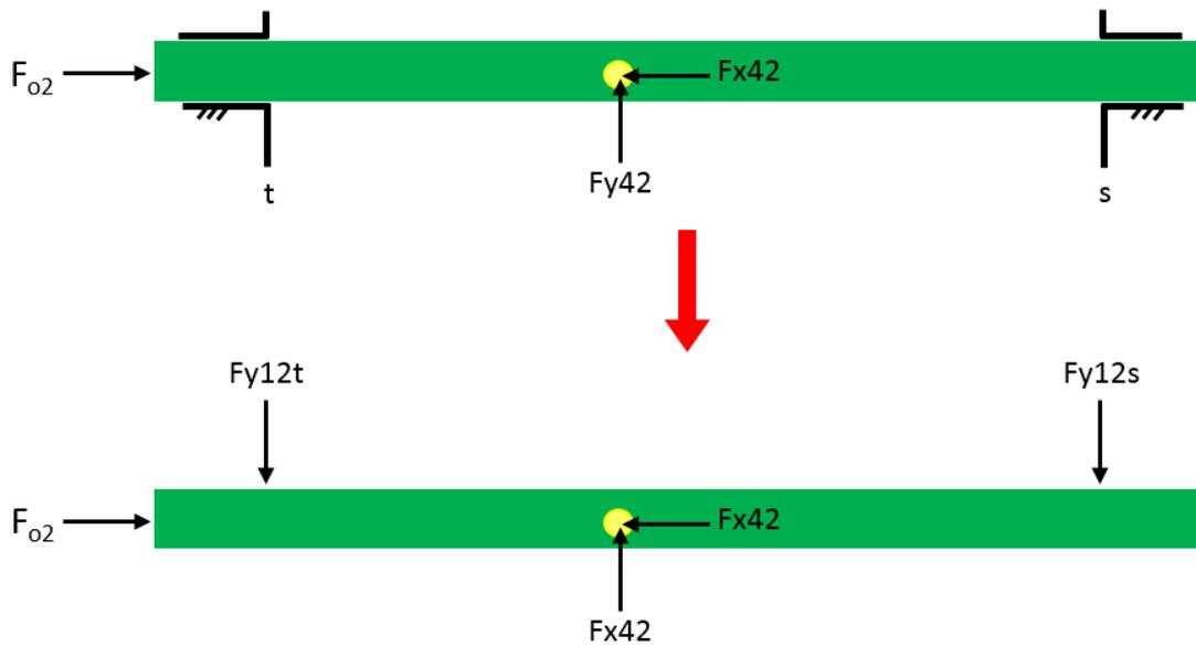
**Figure 91** Free body diagram of driving rod (link 2)
