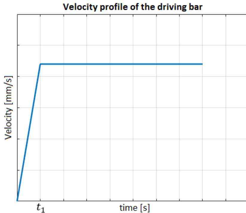
**Figure 123** Assumed velocity profile of the driving bar during its throwing motion
