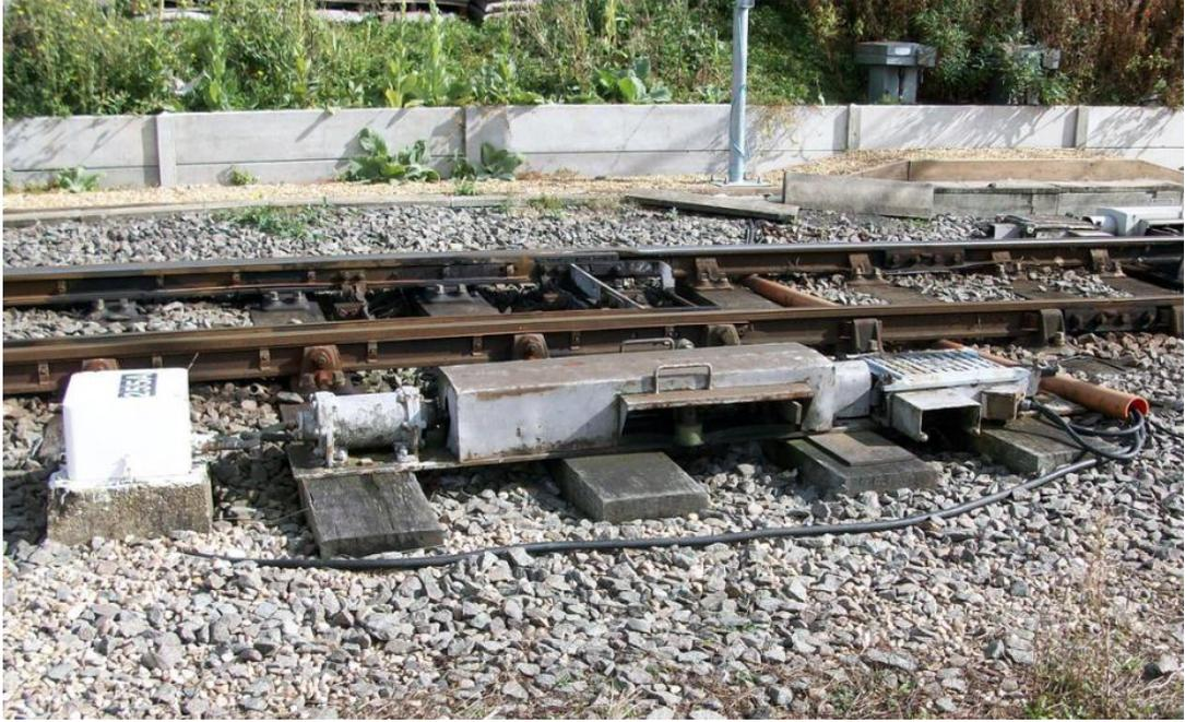
**Figure 10** An electro-pneumatic point machine fitted to 225A points, north of Bletchley Station in England, 27.09.2012. [10]
