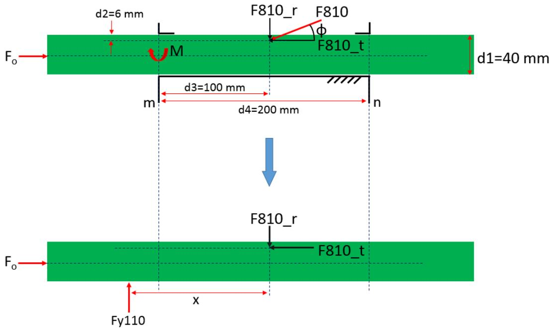
**Figure 121** Free body diagram of component 10
