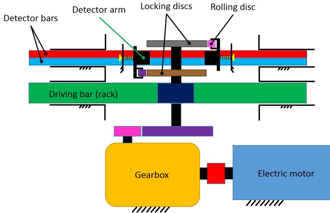
**Figure 76** Representative schematic model of locking mechanism together with the driving mechanism from top view
