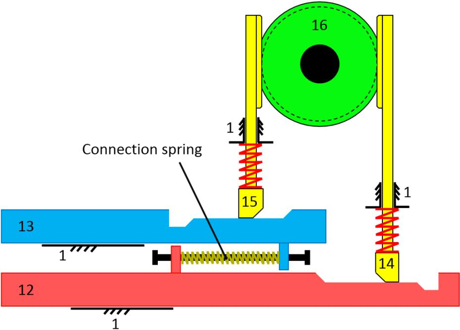
**Figure 134** Schematic representation of the detection mechanism
