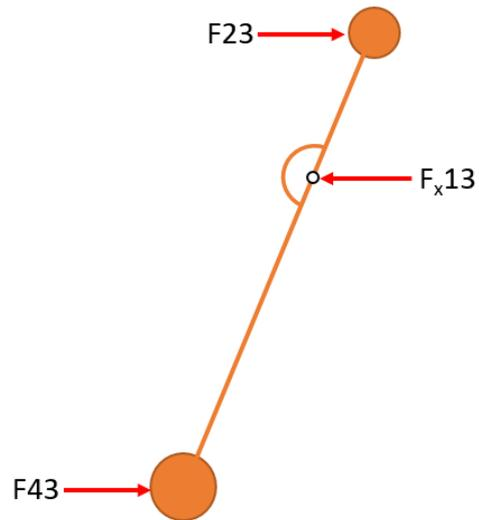
**Figure 45** Free body diagram of link 3
