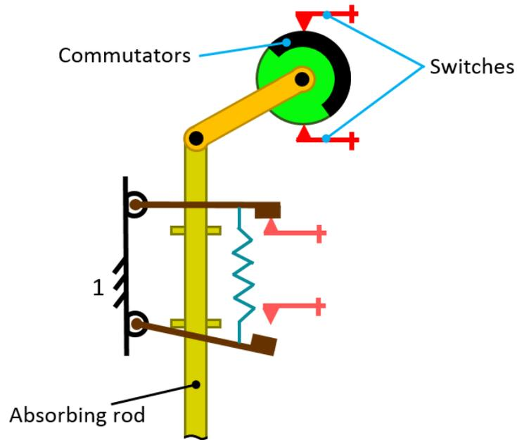
**Figure 136** Schematic representation of position commutators operated by the absorbing rod
