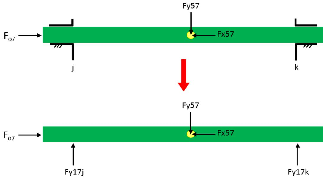
**Figure 92** Free body diagram of driving rod (link 7)
