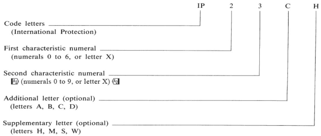
**Figure 141** Arrangement of the IP Code (Section 4.1 in [31])
