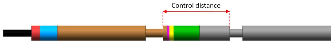
**Figure 55** The control distance on the detector rod for the adjustment of different point blade motions
