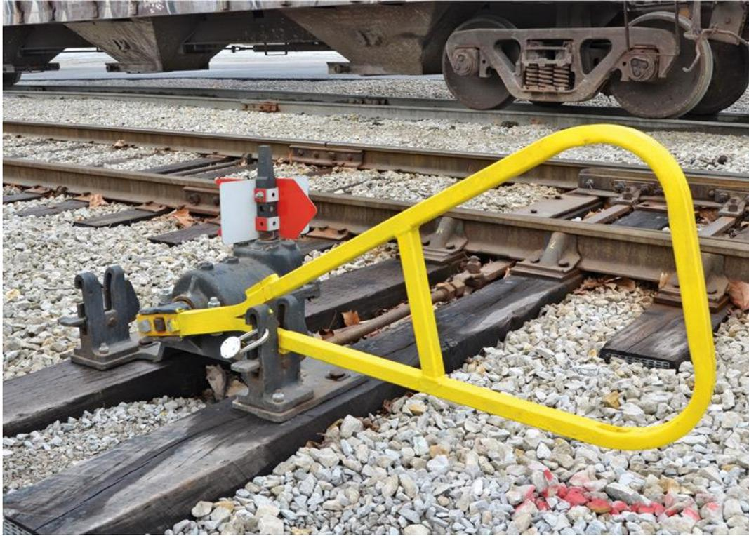
**Figure 7** An example of racor type point lever and padlocked latch in a position [5]
