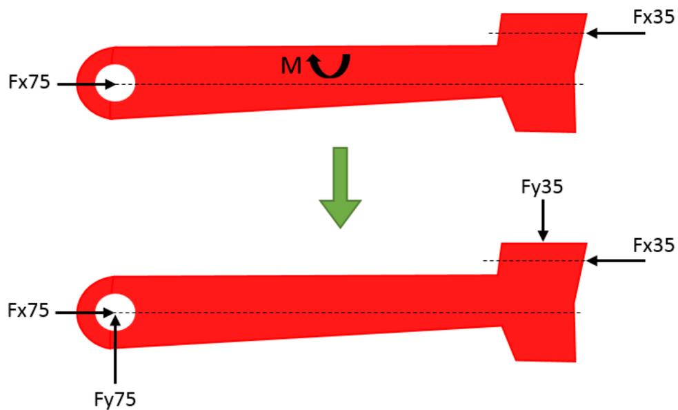
**Figure 90** Free body diagram of right locking clamp
