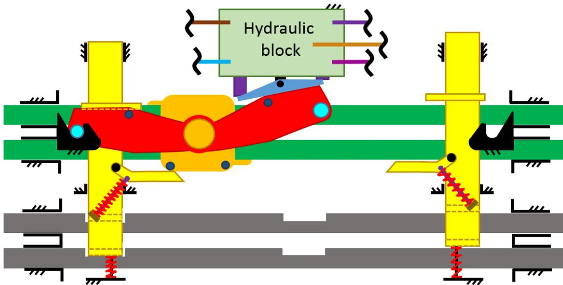
**Figure 102** Locked position of the machine at the left position
