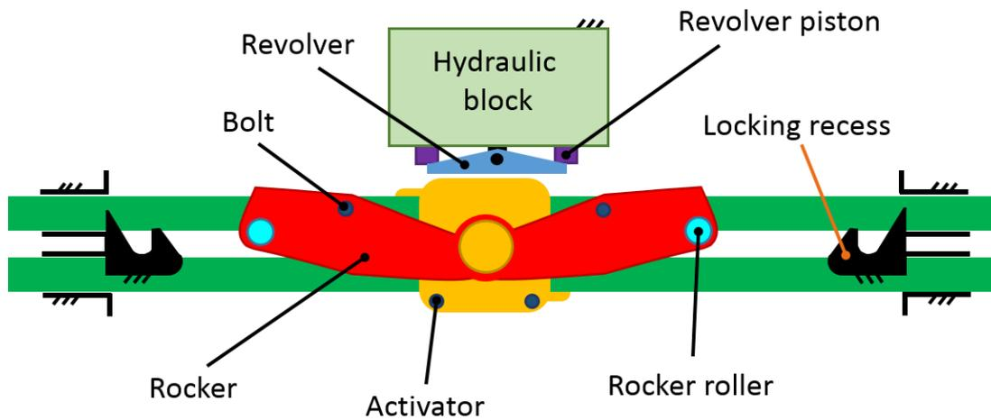
**Figure 98** Schematic representation of locking mechanism for driving rods
