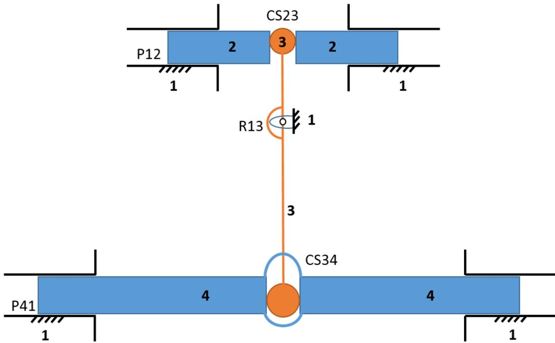
**Figure 41** Kinematic joint types between the links
