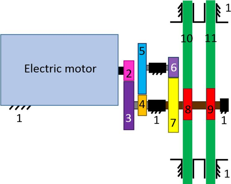
**Figure 117** Representative schematic model showing the machine elements of driving mechanism
