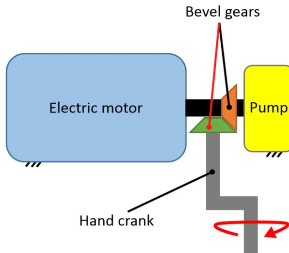
**Figure 108** Schematic representation of the use of hand crank
