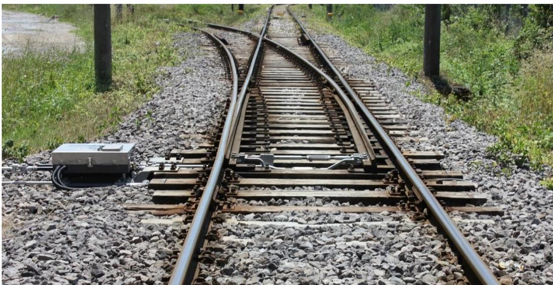
**Figure 1** Photograph of a railway point (switch) at Arifiye train station in Turkey, 12.09.2017.
