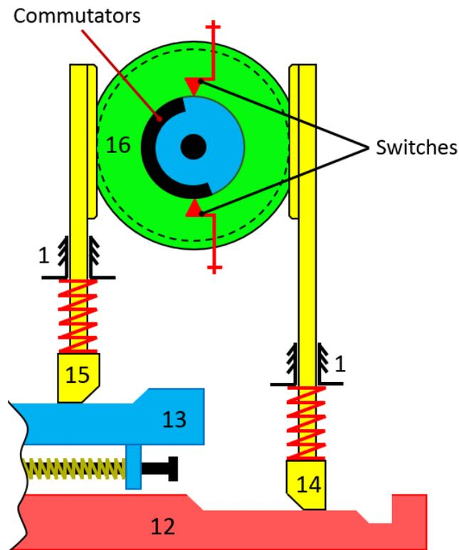
**Figure 137** Schematic representation of commutators controlling the tips of point blades
