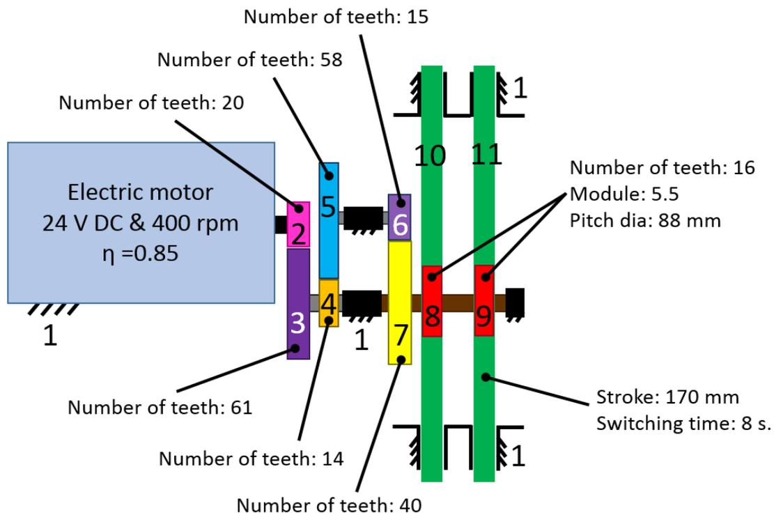
**Figure 118** Known and measured parameters of the driving mechanism
