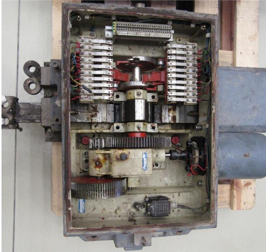
**Figure 60** Photograph of inside view of point machine B
