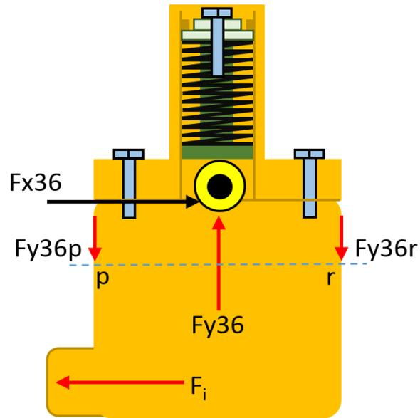
**Figure 87** Free body diagram of throwing block
