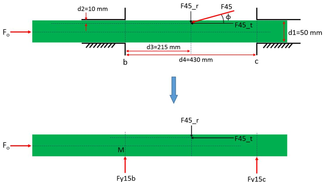
**Figure 67** Free body diagram of link 5
