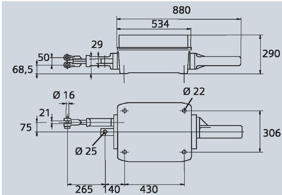
**Figure 14** Some important dimensions of S 700 K in mm [13]
