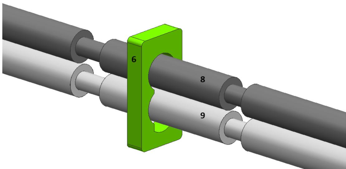
**Figure 52** Two detector rods passing through link 6 while the machine is operating
