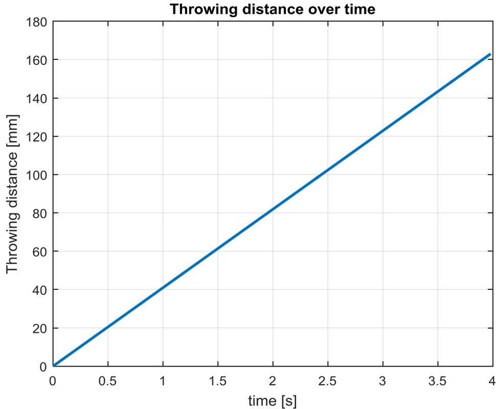
**Figure 93** Throwing distance during the operation time of Point Machine C
