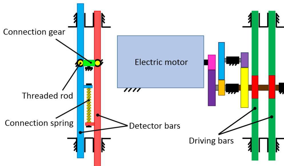
**Figure 133** Representative schematic model of detection mechanism together with the driving mechanism from top view
