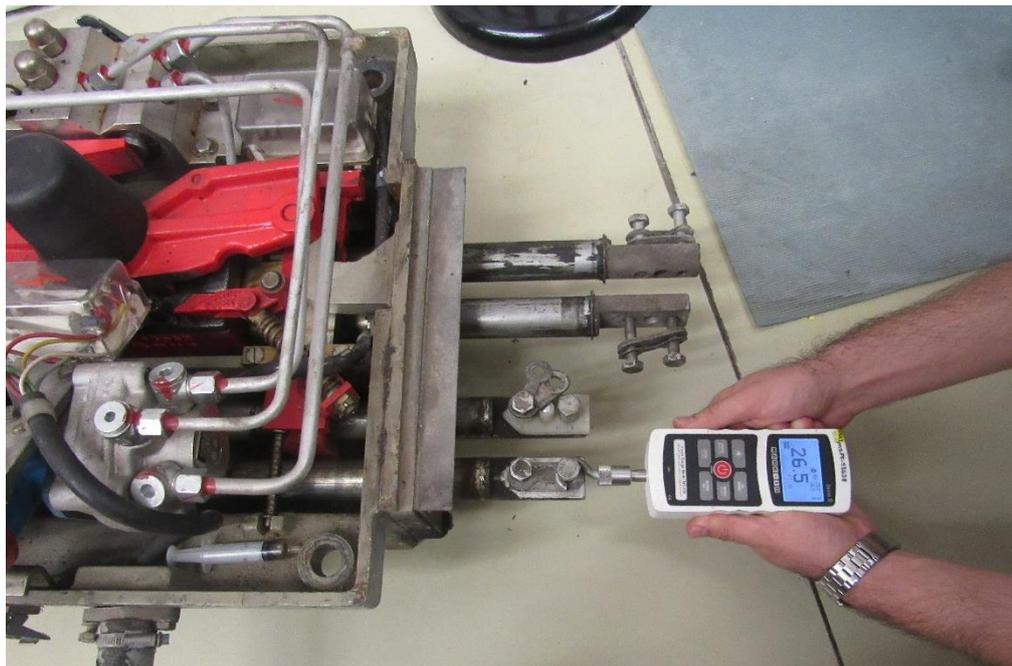
**Figure 96** Force measurement at the linear slides
