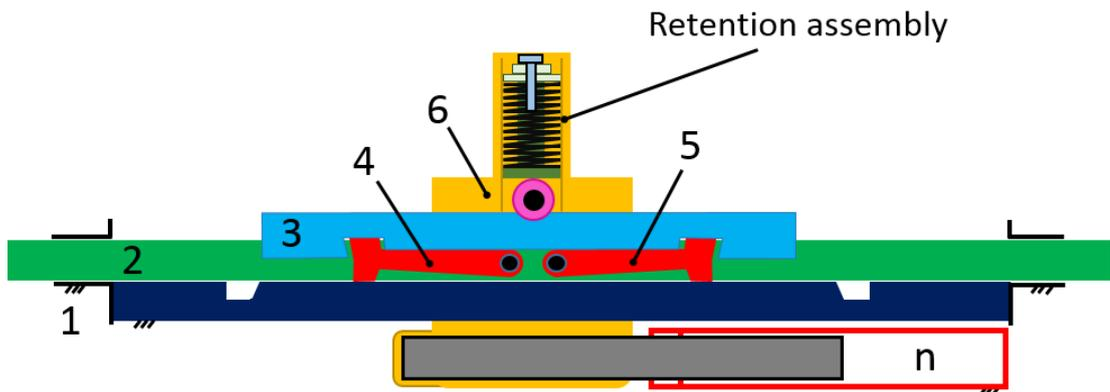
**Figure 86** Schematic representation of driving rods' integration with the throwing block in front view
