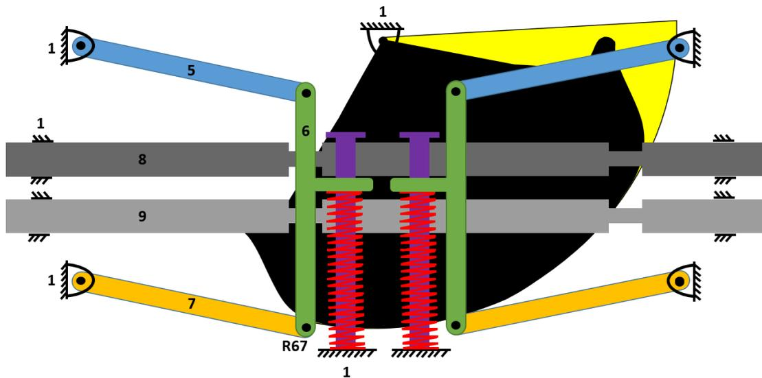
**Figure 57** Unlocking and rotating discs at the just unlocked position of the machine
