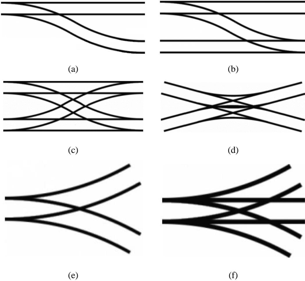
**Figure 2** Schematic representation of simple turnout (a), single crossover (b), double crossover (c), double slip switch (d), equilateral turnout (e) and three-way turnout (f)
