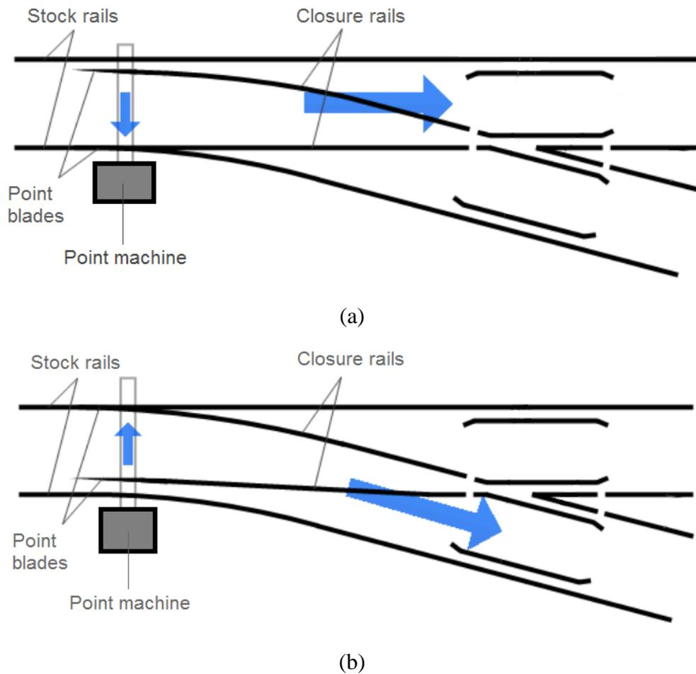
**Figure 3** Schematic representation of a point allowing the train to straight track (a) and to diverging track (b) (adopted from [1])
