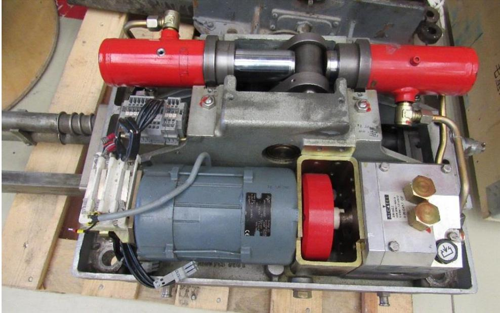
**Figure 36** Photograph of inside view of point machine A
