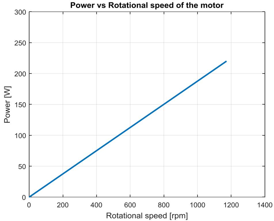
**Figure 71** Power curve of the electric motor with respect to rotational speed
