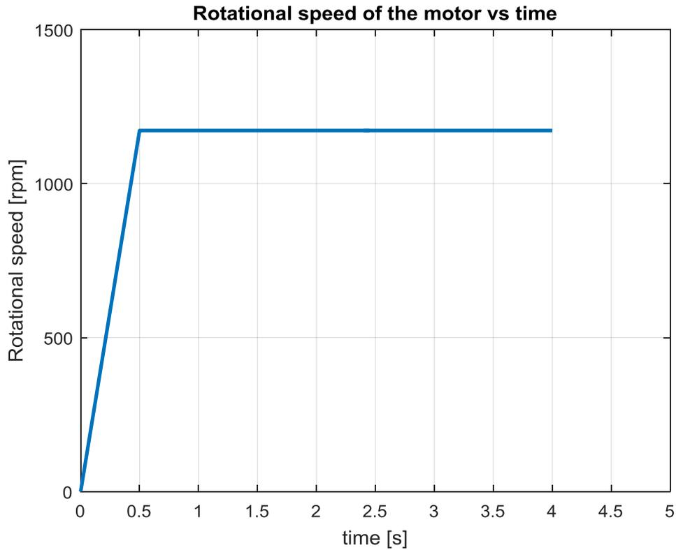
**Figure 72** Motor speed during the operation of the machine
