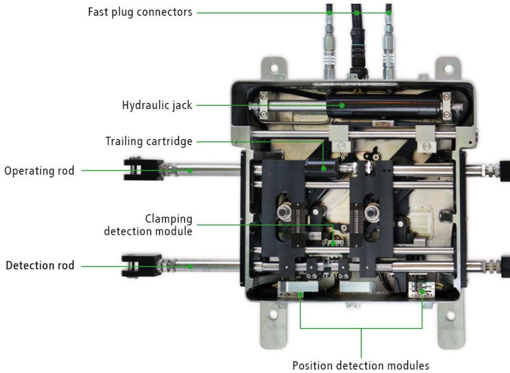
**Figure 26** Inside view and components of Easydrive-i point machine [18]
