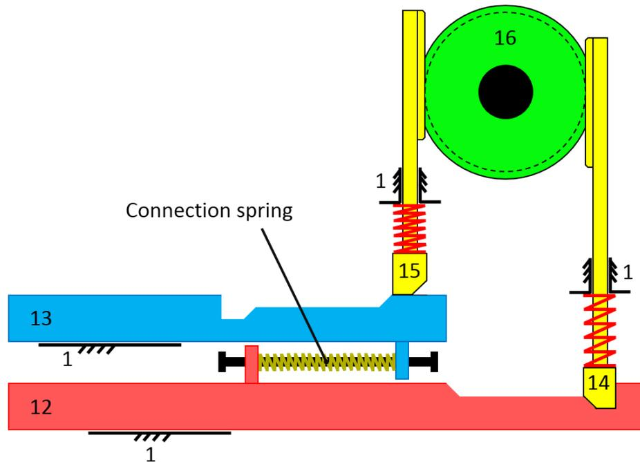
**Figure 135** Schematic representation of locked position of the detection mechanism
