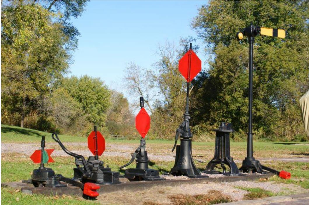
**Figure 6** Some examples of different switch stands with different heights [4]
