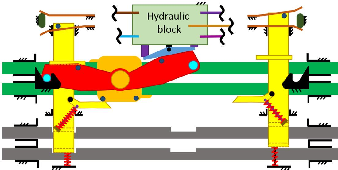
**Figure 106** Locked position of the contact switches at the left hand side
