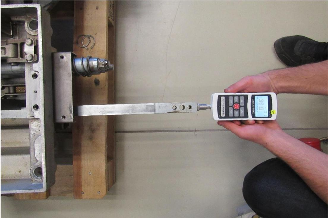
**Figure 49** Force measurement at the linear bearing
