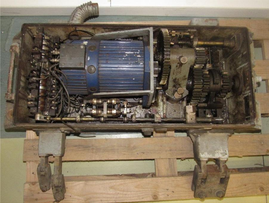
**Figure 115** Photograph of inside view of point machine D
