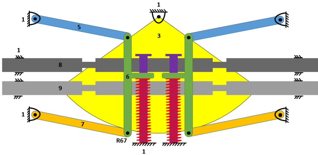
**Figure 51** Schematic representation of locking mechanism together with rotating disc
