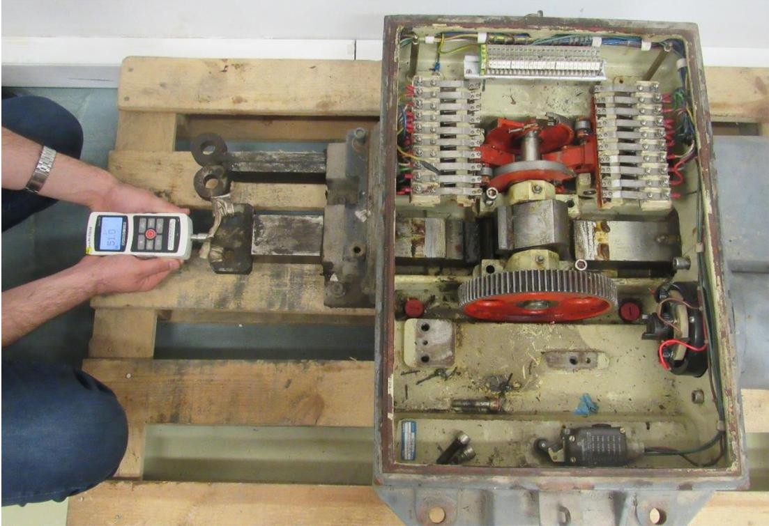
**Figure 74** Force measurement at the linear slides
