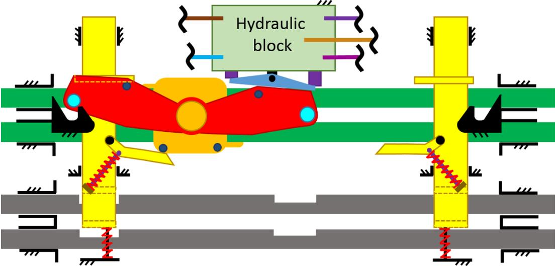
**Figure 104** Schematic representation of the machine at the just unlocked position
