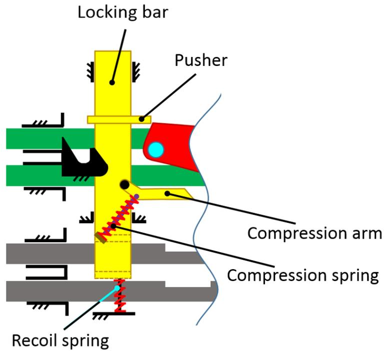
**Figure 99** Schematic representation of locking mechanism for detector rods
