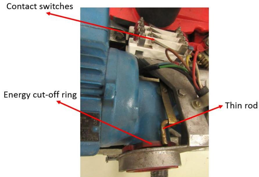
**Figure 110** Energy cut-off mechanism
