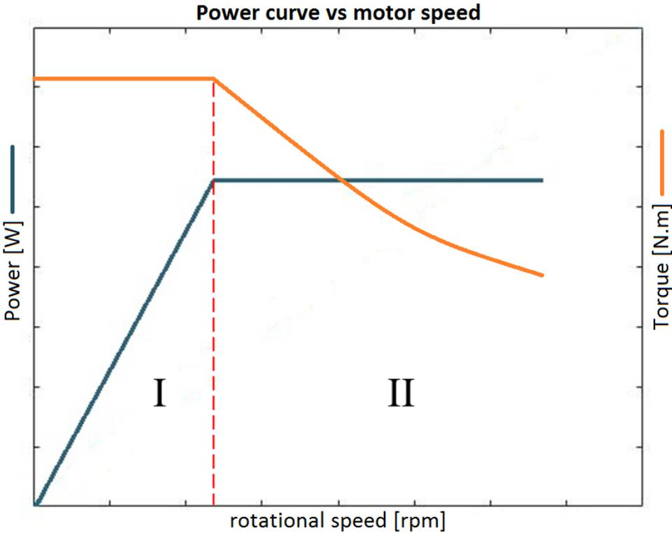
**Figure 122** Typical power curve of a DC electric motor
