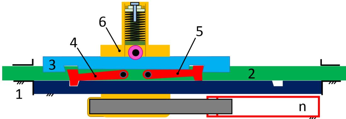
**Figure 95** Schematic representation of falling of locking clamp into a seat
