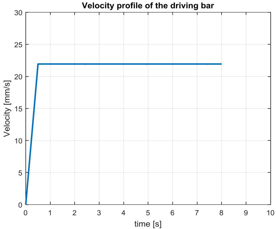
**Figure 124** Velocity profile of the driving bar
