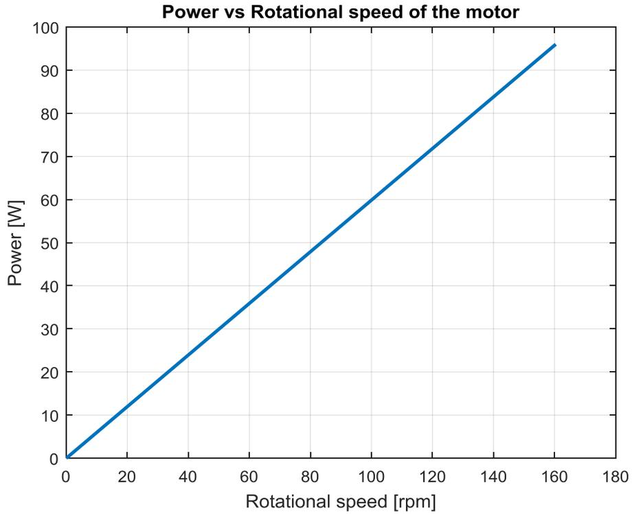
**Figure 126** Power curve of the electric motor with respect to rotational speed
