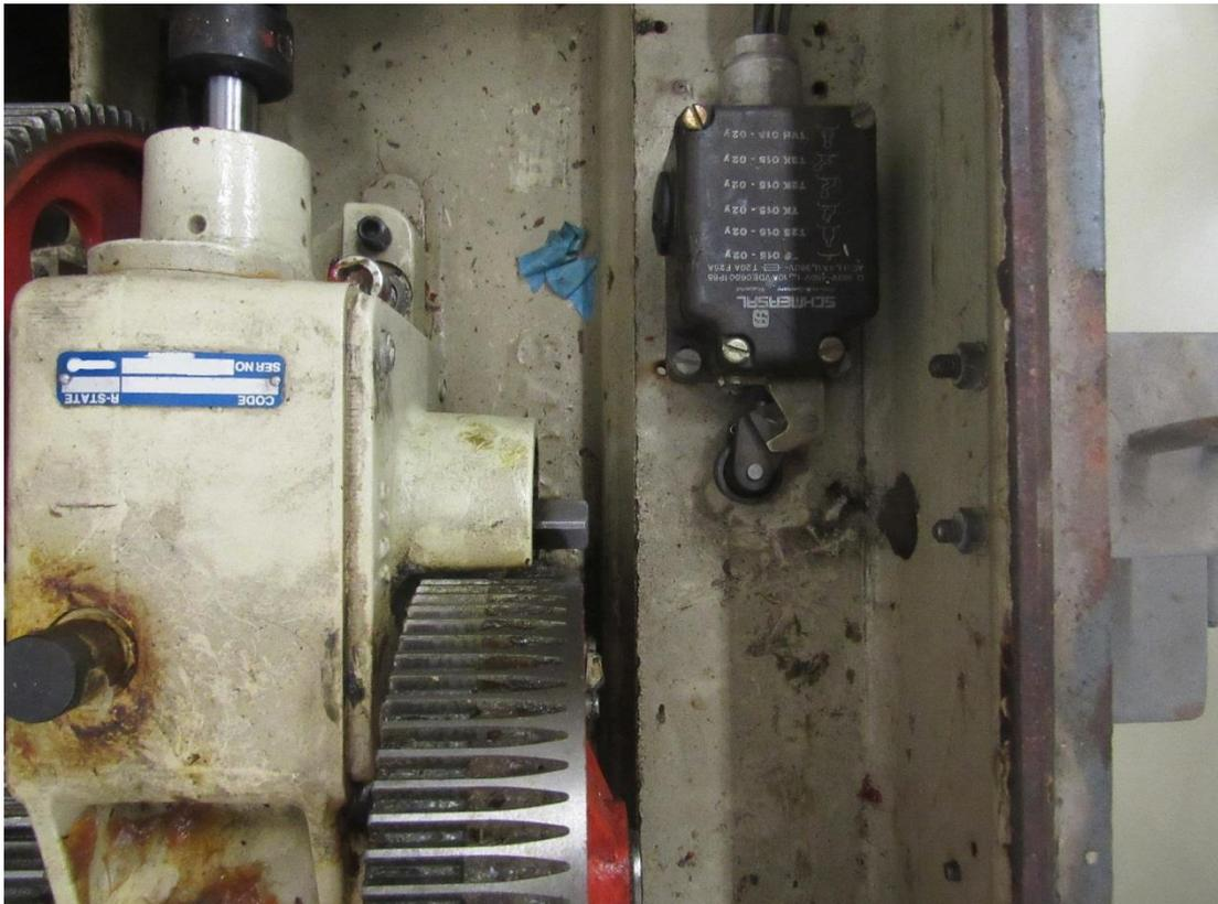
**Figure 82** Safety cut out switch for manual operation
