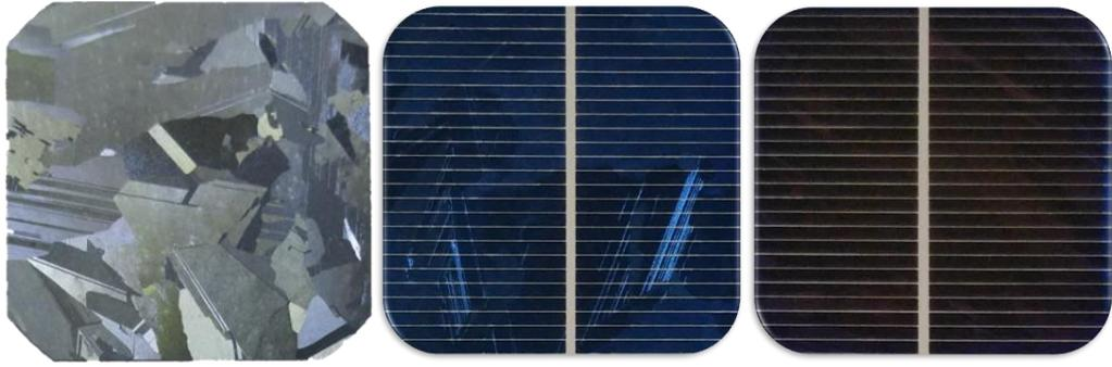
Figure 4.42. Saw damage etched sample (left), Un-textured reference (middle), and laser textured sample (right)
