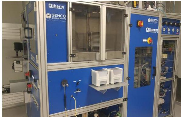
Figure 3.6. Picture of Semco Qtherm PECVD / solid state diffusion system
