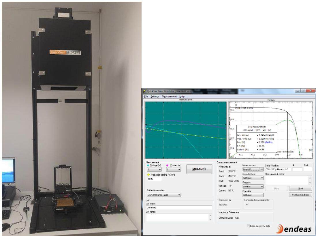
Figure 3.12. QuickSun 120CA-XL for measuring I-V curve (left) and corresponding software (right)
