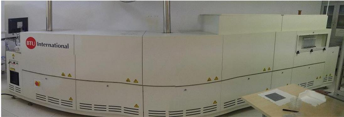
*Figure 3.8. Picture of BTU International firing system*
