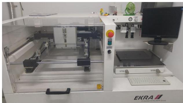
Figure 3.7. Picture of EKRA screen printing system
