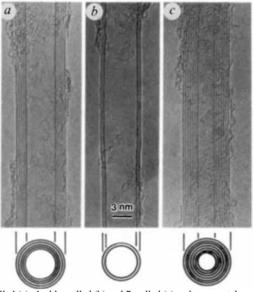
Figure 3. 5 walled (a), double walled (b) and 7 walled (c) carbon nanotubes as observed by Iijima [1].
