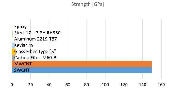
Figure 5. Ultimate strength of various high-performance engineering materials as compared to carbon nanotubes.
