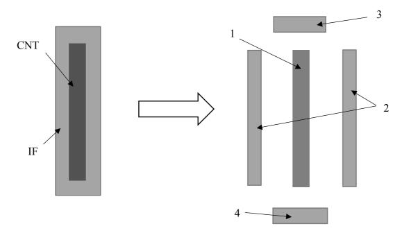
Figure 15. Partitioning of the CNT and interface model into four regions.
