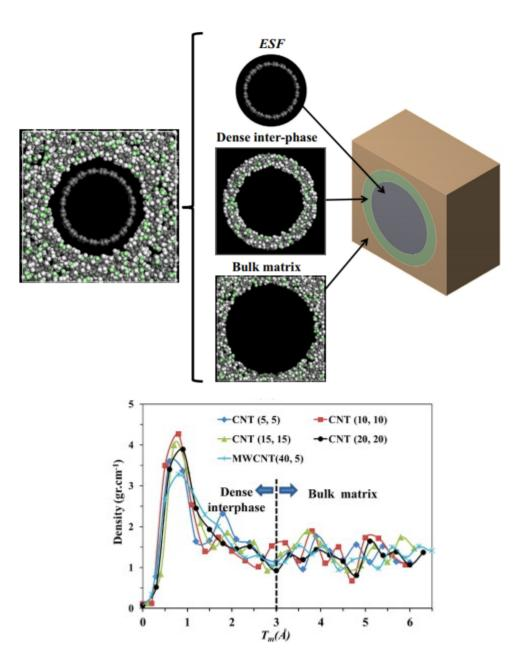
Figure 18. Atomistic images of the interphase region in a Poly Vinyl Chloride (PVC) – CNT Composite (top) and density distribution of Poly Vinyl Chloride (PVC) in the radial direction from surface of the CNT (bottom). Image obtained from [37].
