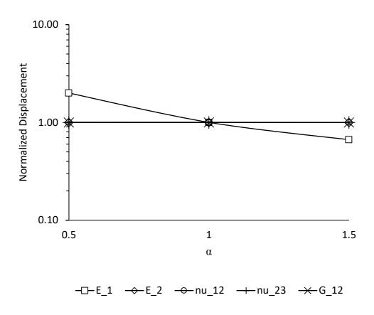
Figure 34. Variation of axial displacement in axial loading as a function of effective fiber moduli.
