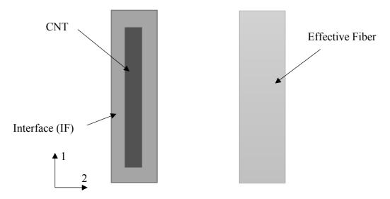
Figure 10. Side views of finite element models consisting of CNT and the interface (left), and effective fiber (right).
