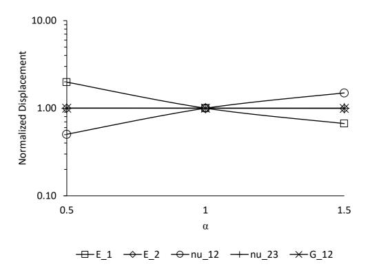
Figure 36. Variation of axial displacement in radial loading as a function of effective fiber moduli.
