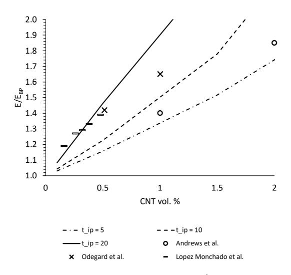
Figure 26. Results of the current model using a CNT radius of 3.9 Å, interphase thickness of 3 Å, and a = 5 compared to experimental and numerical findings in the literature [14,41,42].
