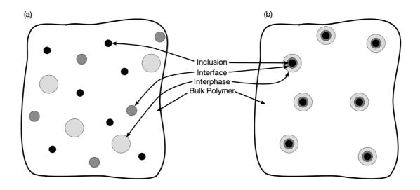
Figure 8. Mori-Tanaka distribution of micromechanical inclusions (a), and the distribution in an actual carbon nanotube composite (b).
