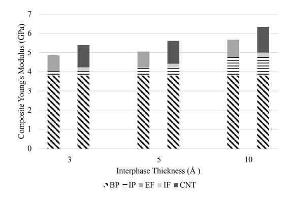
Figure 24. Contribution of each phase to the modulus of the nanocomposite when using a stiff interface model.
