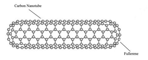
Figure 1. An illustration of a carbon nanotube.
