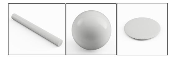
Figure 30. Cylindrical (left), spherical (center) and plate-like (right) inclusion shapes.
