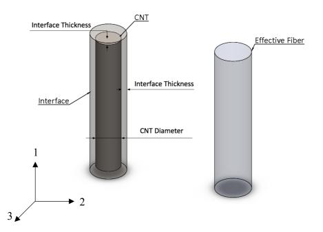
Figure 9: Isometric views of finite element models consisting of CNT and the interface (left), and effective fiber (right).
