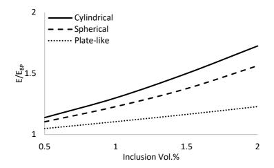
Figure 31. Variation of normalized composite Young's modulus, E/E<sub>BP</sub> as a function of inclusion volume fraction for cylindrical, spherical ad plate-like inclusions.
