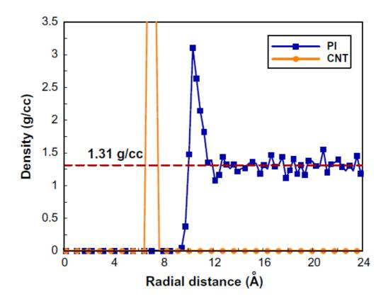
Figure 17. Density distribution of a PI-CNT composite in the radial direction originating in the center of the CNT. Image courtesy of [24].
