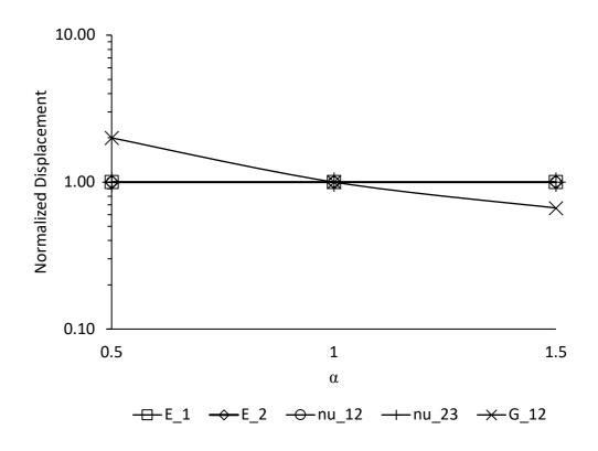
Figure 37. Variation of hoop displacement in torsional loading as a function of effective fiber moduli.
