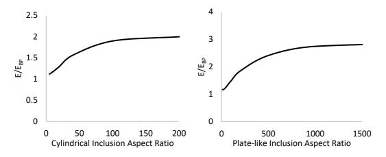
Figure 32. Variation of normalized composite Young's modulus as a function of cylindrical inclusion aspect ratio (left) and plate-like inclusion aspect ratio (right).
