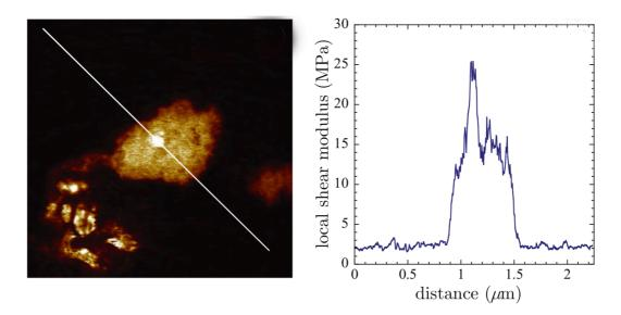
Figure 20. Illustrated AFM measurement of the local shear modulus around a TiO<sub>2</sub>-Elastomer nanocomposite. Note that the abscissa of the plot on the right side corresponds to the white line crossing the nanoparticle on the left side. Image obtained from [39].
