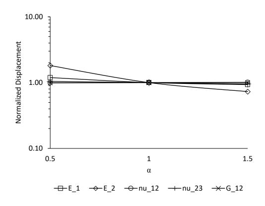
Figure 35. Variation of radial displacement in radial loading as a function of effective fiber moduli.
