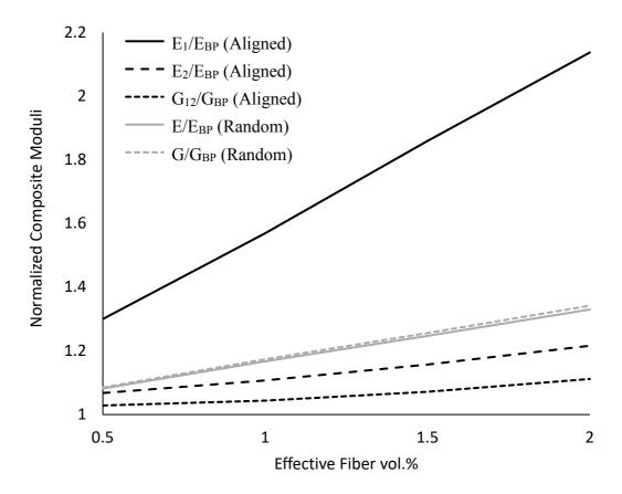
Figure 27: Composite moduli vs effective fiber vol.% for aligned and random inclusion distributions.
