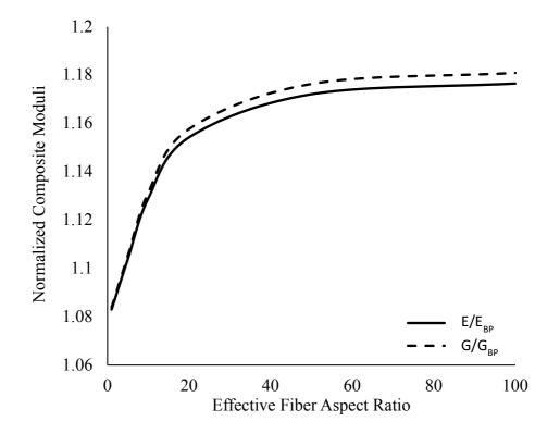
Figure 28: Composite Young's and shear moduli vs effective fiber aspect ratio
