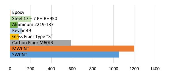
Figure 4. Young's modulus of various high-performance engineering materials as compared to carbon nanotubes.
