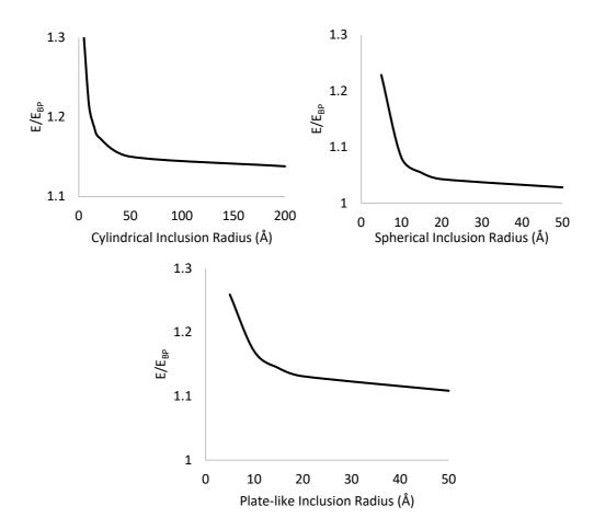
Figure 33. Variation of normalized composite stiffness with respect to cylindrical inclusion radius (top left), spherical inclusion radius (top right), and plate-like inclusion radius (bottom).
