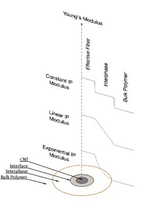
Figure 19: Representative Young's modulus distribution across the micromechanical model. This representation of the interphase is in line with the observations made in experiments of nanoparticulate composites as shown in Figure 20 and Figure 21.
