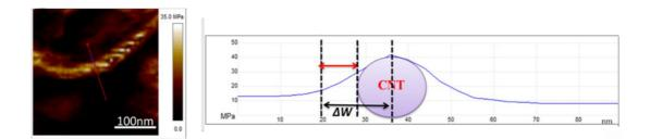
Figure 21. Representative Young's modulus of CNT-Natural Rubber nanocomposite and its corresponding modulus-length curve to represent the interphase thickness. Image obtained from [40].
