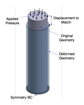
Figure 12: Loading conditions used to obtain the longitudinal modulus of the effective fiber.
