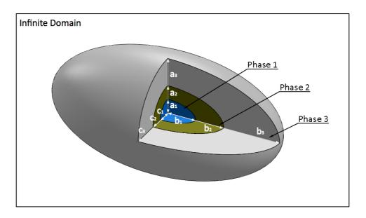
Figure 6. Graphical representation of the phases in the micromechanical model used in this study.
