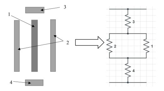
Figure 16. Simplification of the 4 regions in the CNT + interface model with linear springs.
