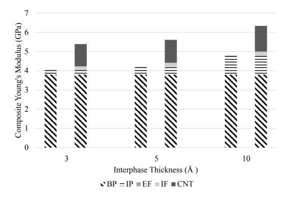
Figure 25. Contribution of each phase to the modulus of the nanocomposite when using a soft interface model.
