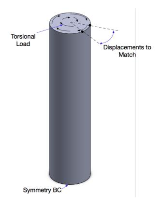
Figure 14: Loading conditions used to obtain G<sub>12</sub>.
