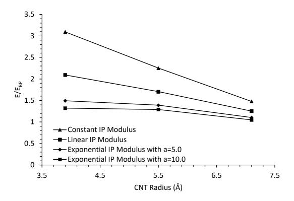
Figure 23. Normalized composite moduli vs CNT radius for various interphase moduli distributions.
