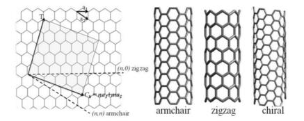
Figure 2. Carbon nanotube chirality vector.
