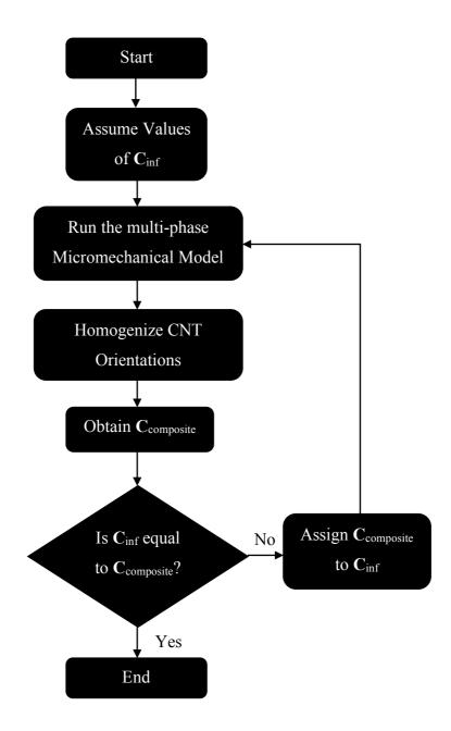
Figure 7. Sequence of operations in the current micromechanical model.
