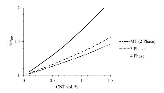
Figure 22. Comparison of 2-phase, 3-phase and 4-phase micromechanical models.
