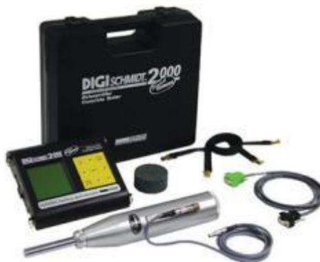
**Figure 4.2** Schmidt hammer test device
