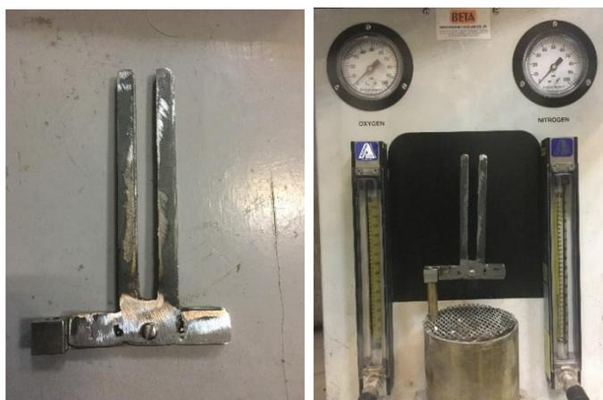
**Figure 9.** Frame with a width of 1 cm and test setup for the LOI test.
