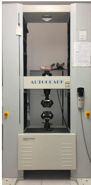
**Figure 7.** Shimadzu Autograph AG-IS 100kN universal tensile test machine.
