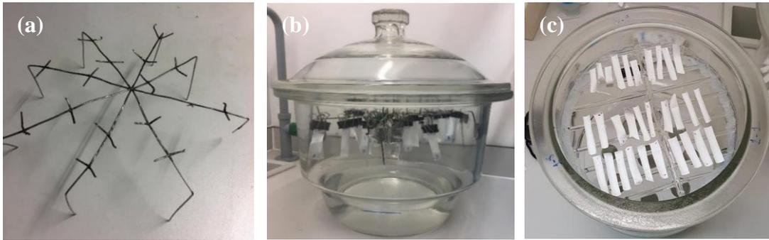
**Figure 10.** (a) Sample holder of the old setup (b) desiccator where the experiments are carried out with the first setup (c) new setup with glass grid.
