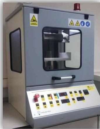
**Figure 6.** Inovenso Ne 300 electrospinning device.
