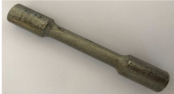
Figure 4.6: A sample of X and Y specimens after grinding operation
