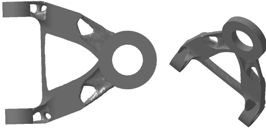
Figure 5.22: Last optimized model for vertical part with smooth surfaces
