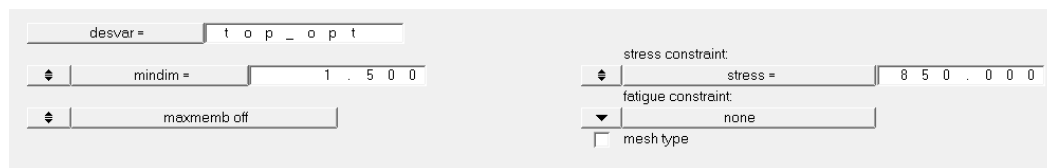
Figure 5.14: Design variable parameters screen for minimum member size control and stress constraint
