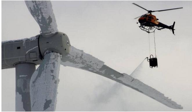
Figure 1.3: De-icing of turbine blades [7].
