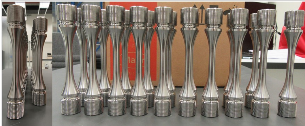
Figure 42 Fatigue test specimens after machining.
