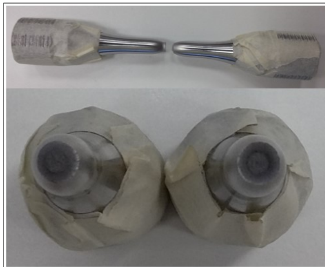
Figure 66 Cup-and-cone type fracture surface for tensile tested specimen (SP-21)
