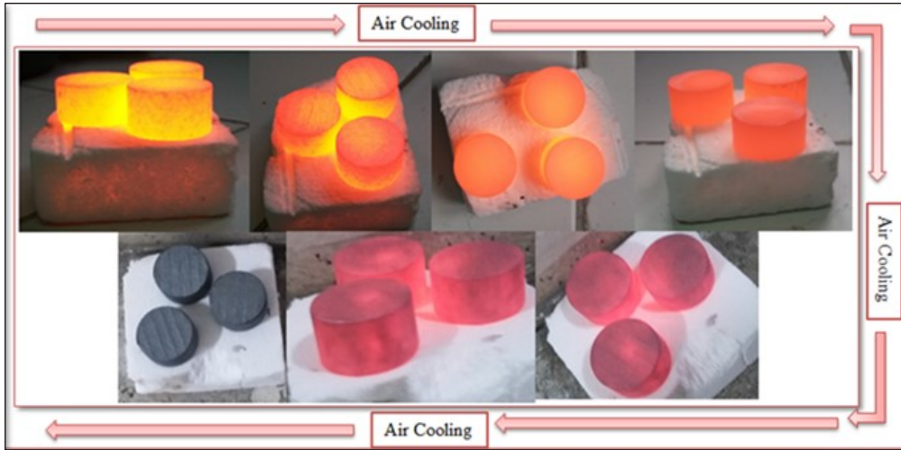
Figure 44 Heat treated specimens during air cooling.
