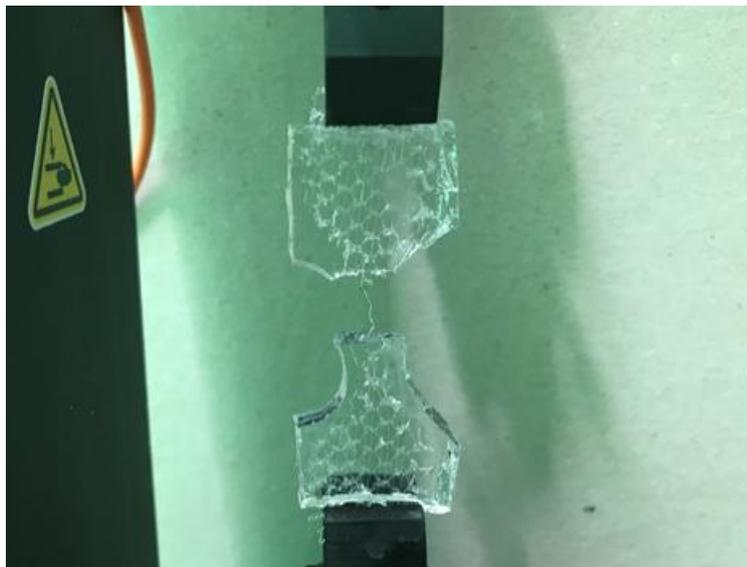
**Figure 3. 12** Image of a PUL25-PP sample breaking after tensile test.
