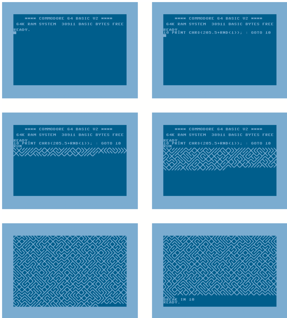
Figure 9 One-lined code “10 PRINT program” is typed into the Commodore 64 and run: repeat infinitely until it is interrupted. Source: Nick Montford, Patsy Baudoin et al. 10 PRINT CHR$(205.5+RND(1)); : GOTO 10 . USA: The MIT Press, 2013: 2.
