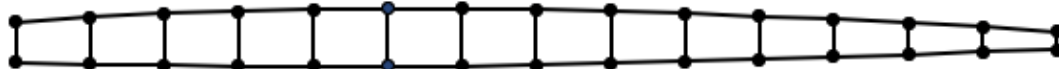
Figure 4-13 Panels and Booms at the Cross-Section of the Wingbox for the Supersonic Fighter Wing
