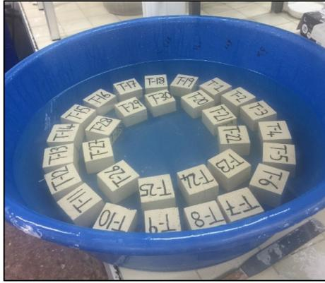
Figure 15: Cubic travertine stone samples (numbered from 1 to 30) in sodium sulfate solution
