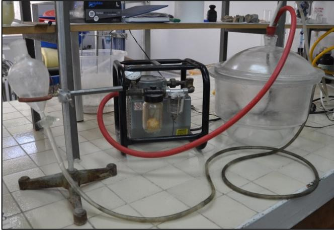
Figure 17: Vacuum chamber used in porosity measurement experiment
