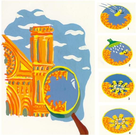
Figure 5: Biomineralisation illustration (1) Spraying of bacteria onto the surface, (2) Spraying of the nutritional medium, (3) Bacterial multiplication, (4) Formation of calcite crystals
