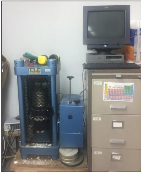
Figure 21: Uniaxial Compressive Strength (UCS) test device
