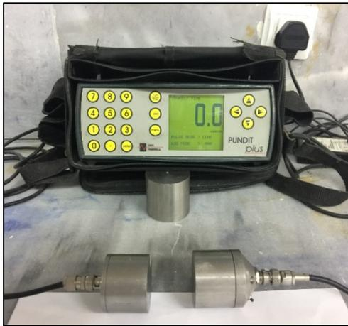
Figure 20: UPV measurement instrument
