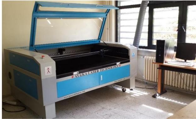
Figure 2-5 Laser cutting machine.
