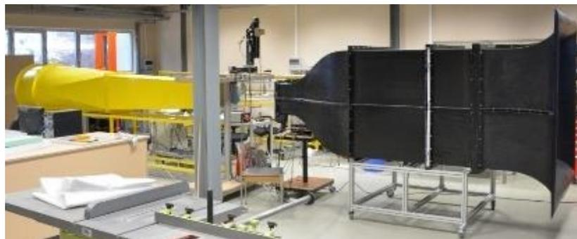
Figure 2-4 Open loop suction type wind tunnel and traversing unit at the top of the test section to measure the incoming flow using HWA.
