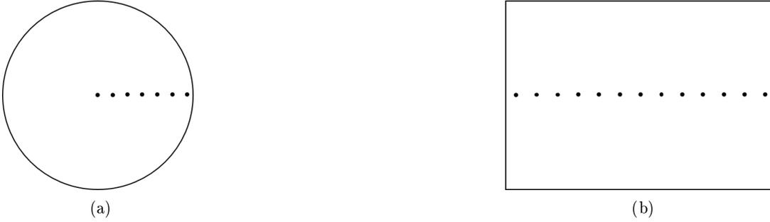
Figure 3.14: Magic field measurement points for mode analysis in (a)cylindrical waveguide (b)rectangular waveguide
