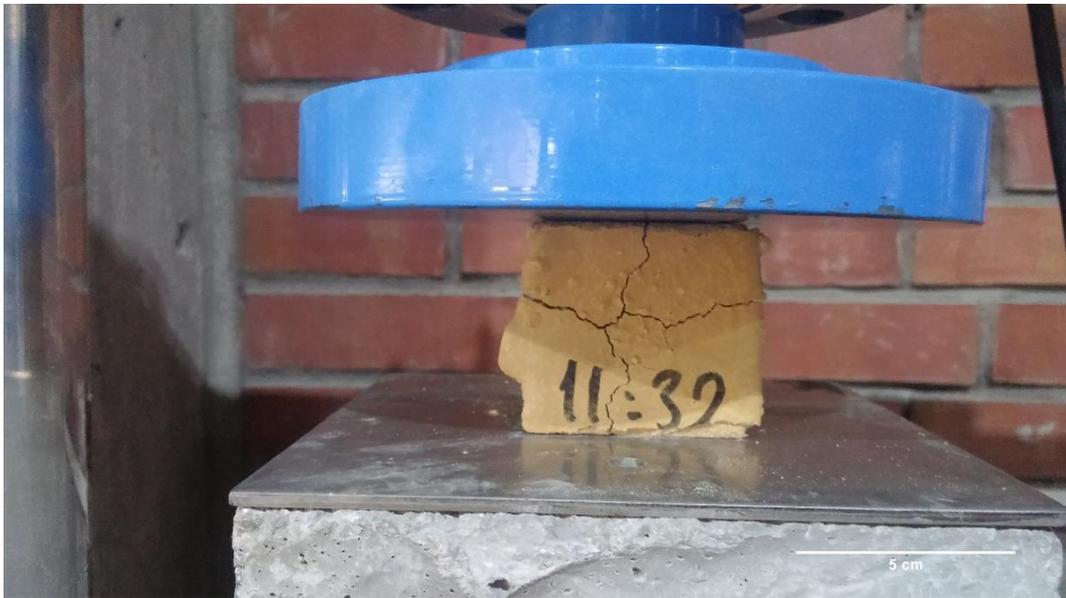
Figure C.1 Cracks on the 5-cm cube sample with  $M/P = 6$  and  $W/B = 0.20$  at 24 h (before testing)
