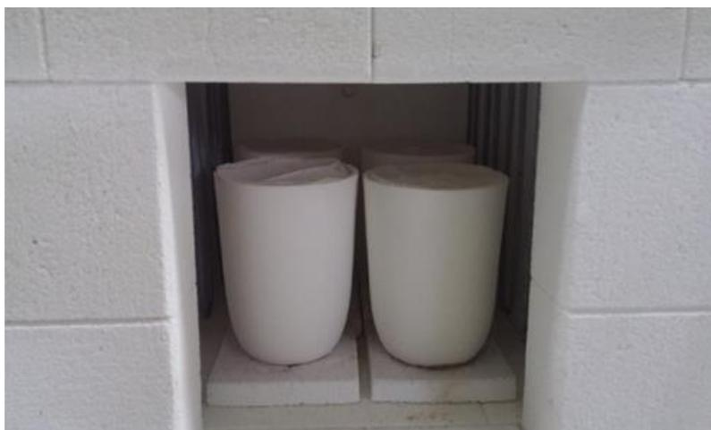
Figure 3.1 The crucibles placed in the furnace (the top diameter of the crucible is almost 10 cm)
