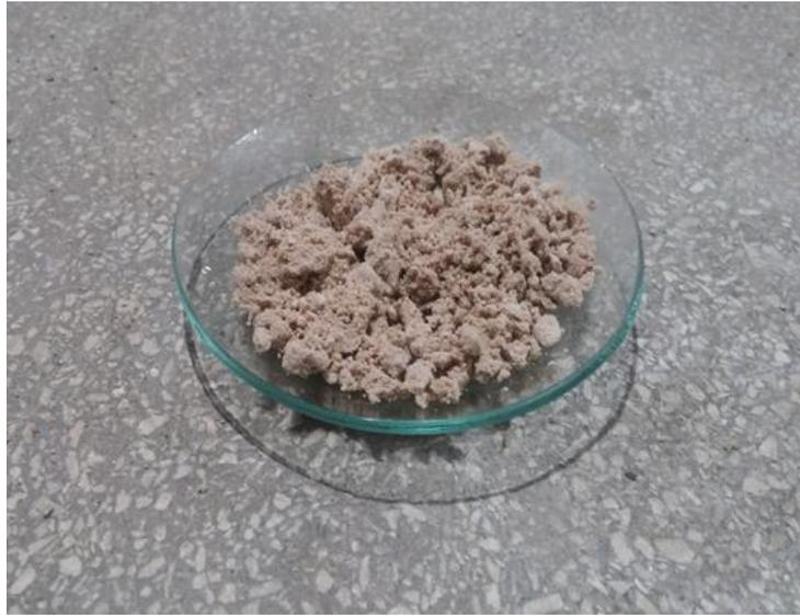
Figure 3.3 A MKPC paste made with a low-temperature calcined MgO, dry and crumbly (image width is approximately 10 cm)
