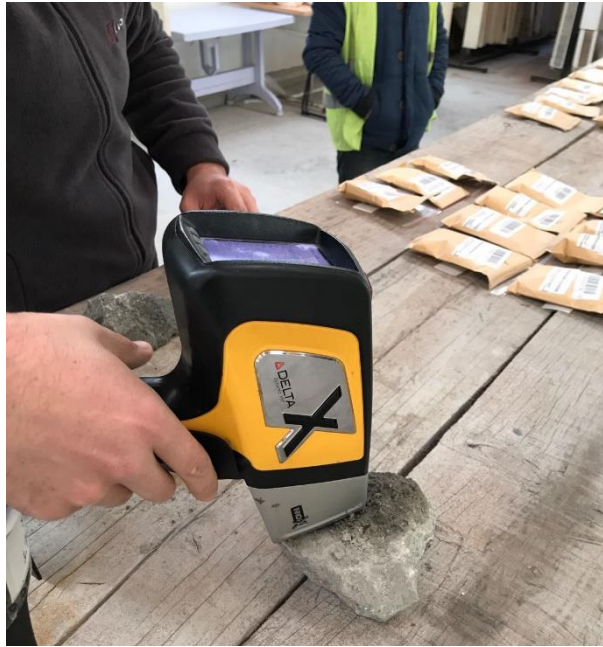
Figure 4.3 XRF Gun Test at Kışladağ Gold Mine, in Uşak. November 23, 2017.
