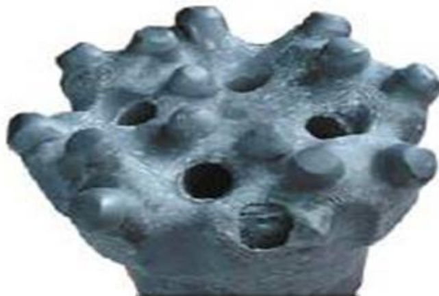
Figure 2.24 Excessive Button Protrusion, Purdy, 2014
