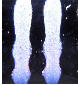
Figure 5.7: Color of LC processed PECVD deposited a-Si layer
