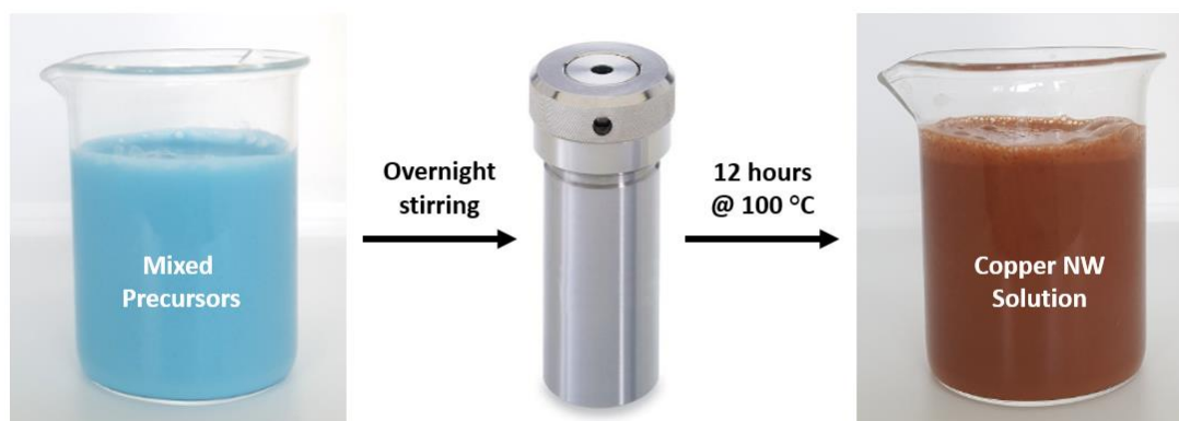
Figure 2. 7 Cu NW synthesis route via hydrothermal method used in this work.
