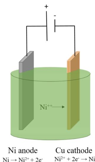
Figure 5 Schematical representation of a typical nickel plating cell
