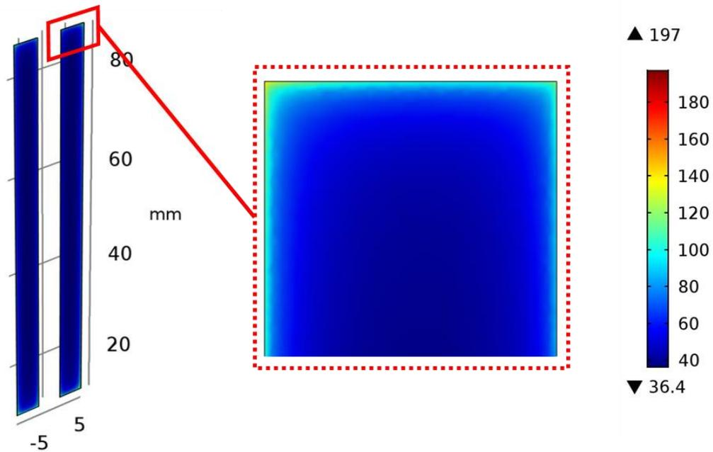
Figure 10 Calculated thickness distribution of electrodeposited nickel on copper strips used to measurements residual stress
