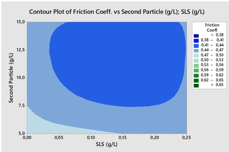
Figure B.15 The counter plot for COF with respect to amount of SLS and  $Al_2O_3$
