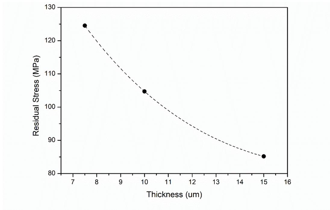
Figure 32 The effect of coating thickness on residual stress at pH of 3, the addition of 0.25 g/l ALS and the current density of 8 A/dm<sup>2</sup>
