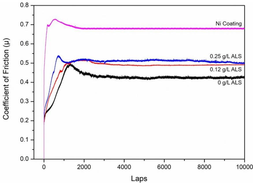
Figure 27 Recorded COF values during measurements at 5 A/dm<sup>2</sup> current density without SLS
