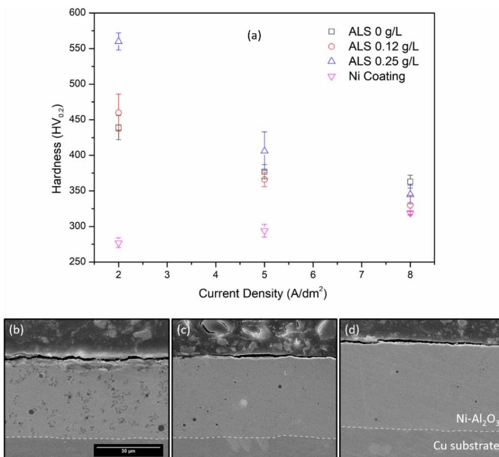
Figure 18 (a) The effect of current density with and without surfactants on hardness. Cross-sectional SEM images of the coatings with 10 g/l Al<sub>2</sub>O<sub>3</sub>, 0 g/l SLS and 0.25 g/l ALS at (b) 2 A/dm<sup>2</sup>, (c) 5 A/dm<sup>2</sup> and (d) 8 A/dm<sup>2</sup>
