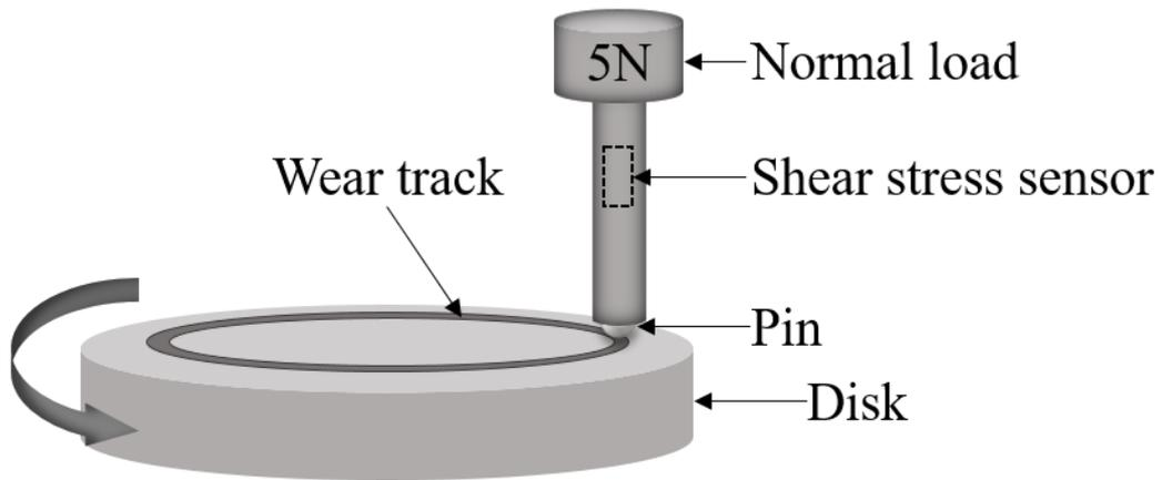
Figure 12 Schematical representation of pin-on-disk test setup
