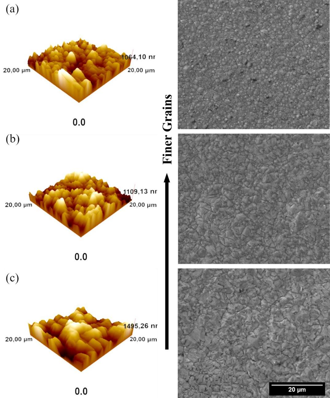
Figure 34 Surface analysis via AFM and SEM images of composite coatings at (a) 2, (b) 5 and (c) 8 A/dm<sup>2</sup> at 0.12 g/l SLS combined with 0.25 g/l ALS and 10 g/l Al<sub>2</sub>O<sub>3</sub> in the electrolyte
