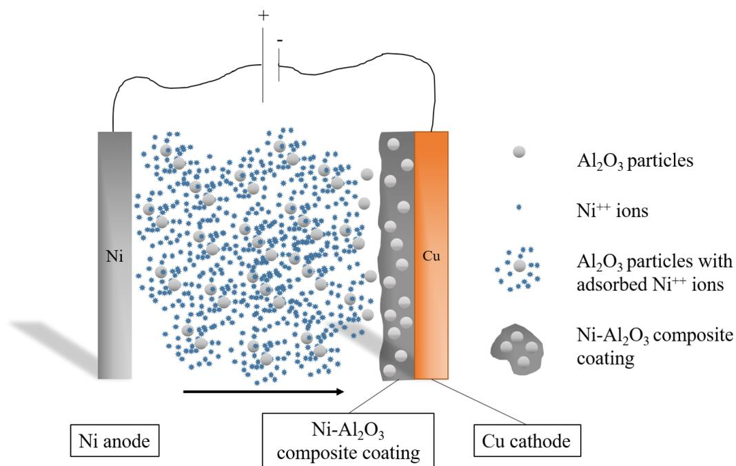
Figure 1 Schematic electrochemical cell for electrocodeposition [9]
