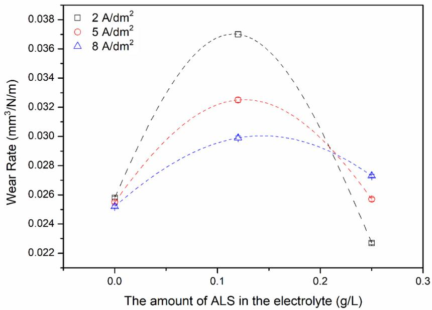
Figure 21 The effect of current density and the amount of ALS on wear rate
