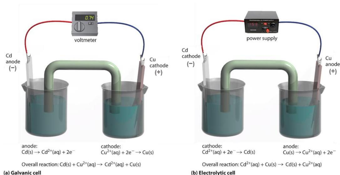
Figure 2 Schematical representation of (a) galvanic and (b) electrolytic cells
