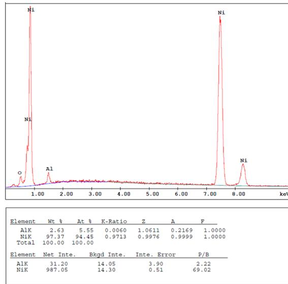
Figure 17 Representative EDS measurement for Ni-9 wt.% Al<sub>2</sub>O<sub>3</sub> composite coating
