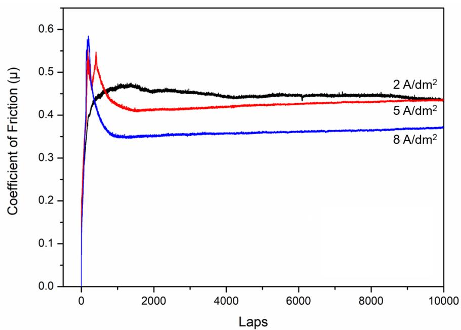
Figure C.4 COF measurements at three different current densities
