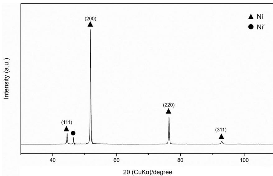
Figure 37 XRD pattern of Ni coating at a current density of 2 A/dm<sup>2</sup> without surfactant
