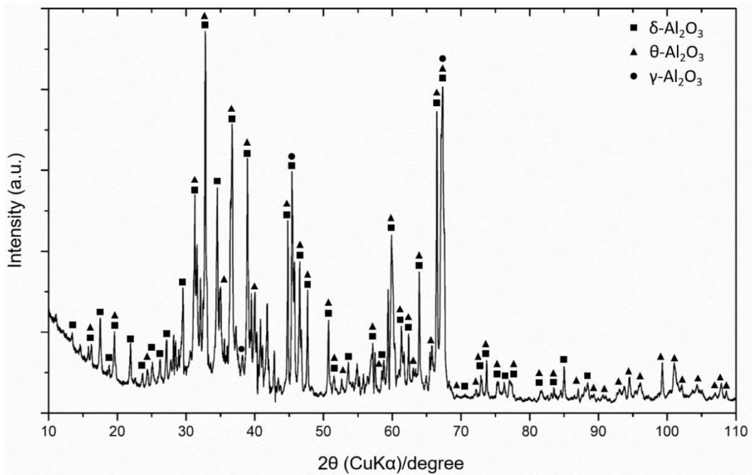
Figure 8 Xray diffraction pattern of alumina powder
