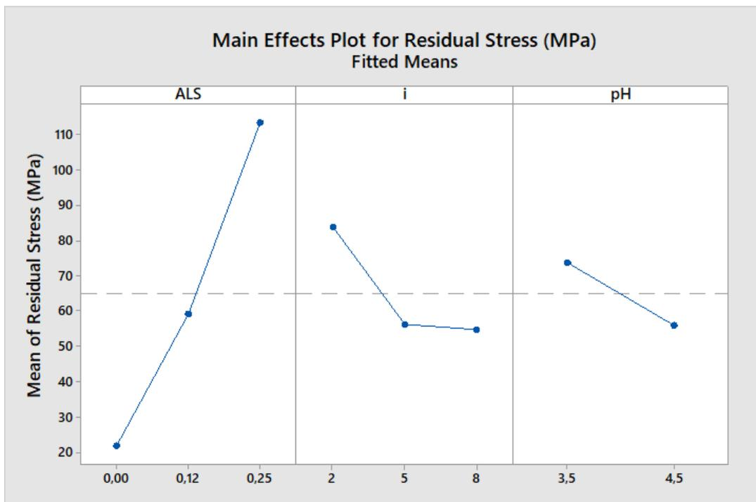
Figure 31 The mean effects plot for residual stress
