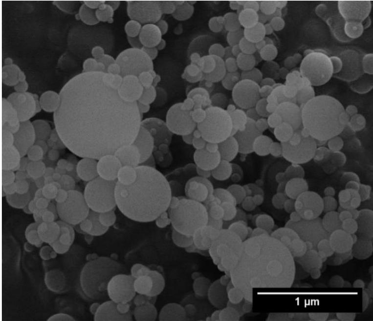
Figure 7 SEM image of submicron spherical alumina powder
