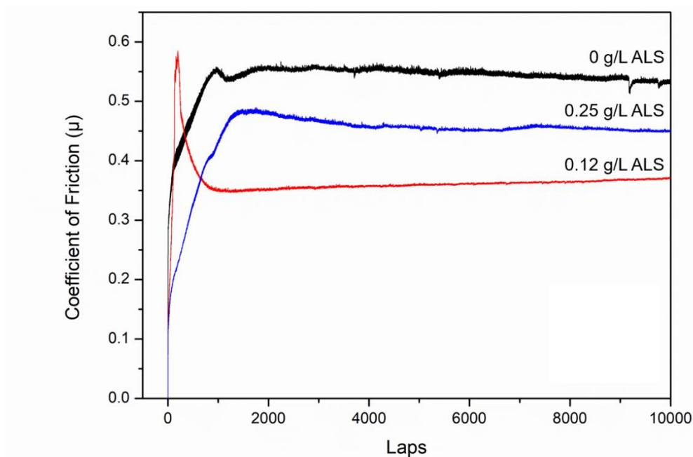
Figure C.3 COF measurements at three different ALS amount
