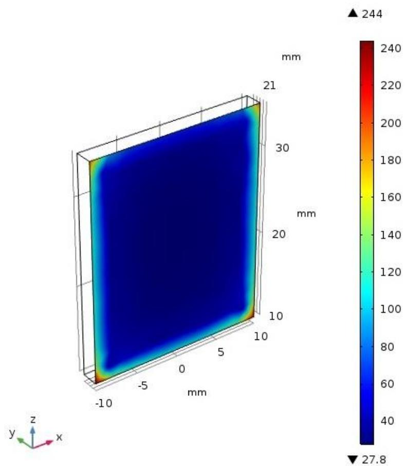
Figure 9 Thickness distribution of electroplated nickel on copper substrate determined by Comsol Multiphysics 5.2 software package
