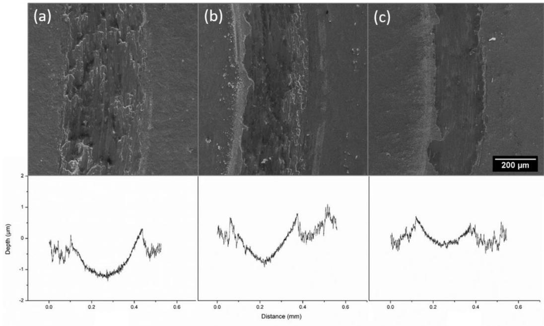
Figure 24 SEM images and surface profiles of the wear track of the composite coatings at current densities of (a) 8 (b) 5 (c) 2 A/dm<sup>2</sup> with 0.12 g/l SLS and 0.25 g/l ALS
