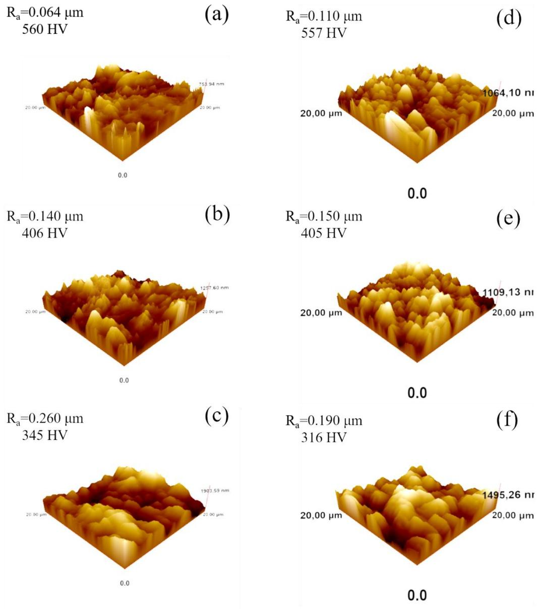
Figure 33 Surface analysis via AFM to understand the effect of current density of (a) 2, (b) 5 and (c) 8  $A/dm^2$  at 0.25 g/l ALS addition, (d) 2, (e) 5 and (f) 8  $A/dm^2$  at 0.12 g/l SLS combined with 0.25 g/l ALS and 10 g/l  $Al_2O_3$  in the electrolyte
