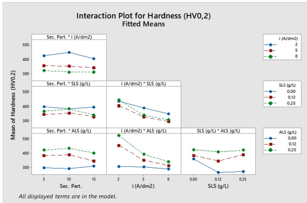
Figure 19 Interaction plot for hardness
