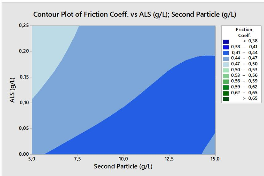
Figure B.11 The counter plot for COF with respect to the amount of ALS and  $Al_2O_3$
