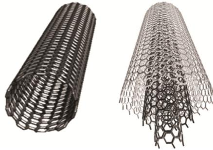
Figure 1.4: Single-walled and multi-walled CNTs. Reprinted from [18]
