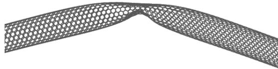
(b) Euler buckling of (10,10) CNT with  $L=30$  nm
