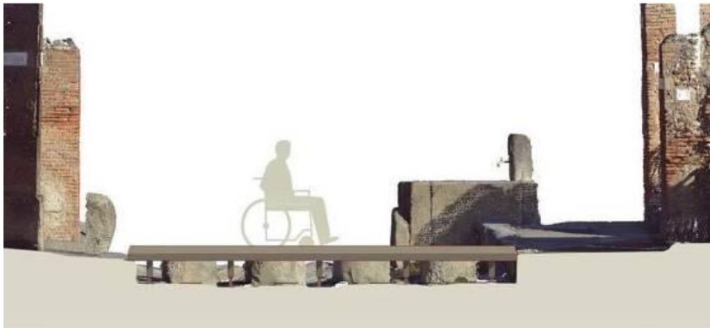
Figure 2-14: The project for the overcoming of the road crossings of Pompeii with the creation of a reversible passage connecting the basalt blocks. Drawing by M.R. Acetoso and B. Rubichi.
