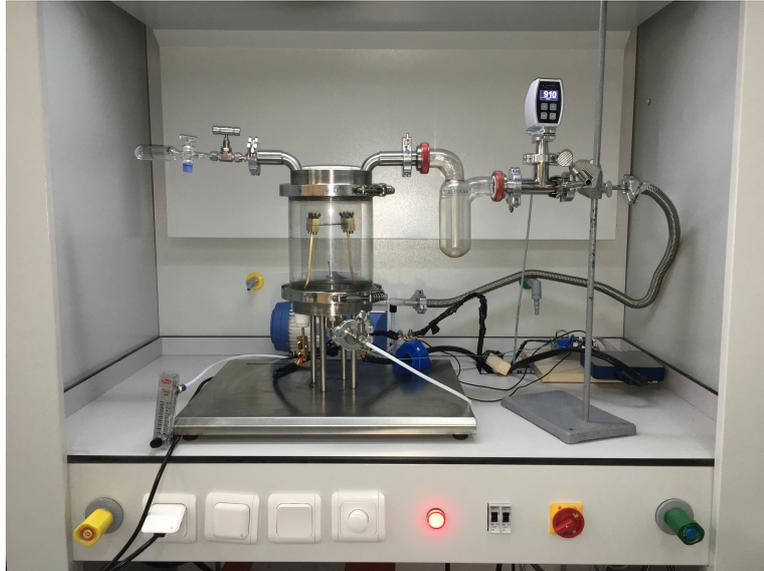
**Figure 3.4** Wire mesh reactor (WMR) in Clean Combustion Technologies Laboratory (CCTL).
