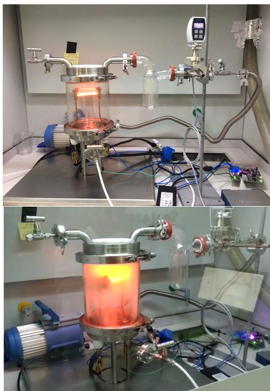
**Figure 3.21** Pyrolysis at 4500 °C/s by using molybdenum wire mesh. In the first image, no sample was placed. In the second image, hazelnut shell (HS) was pyrolyzed at 1550 °C.
