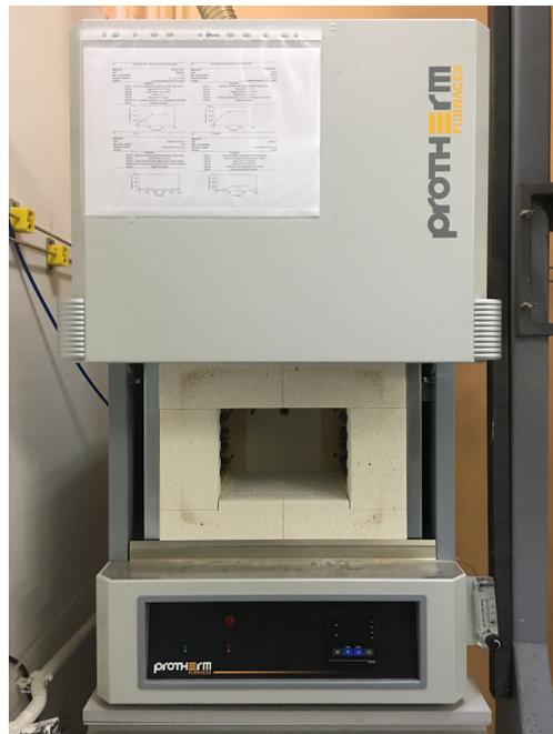
**Figure 3.14** Protherm ashing furnace at Clean Combustion Technologies Laboratory (CCTL)
