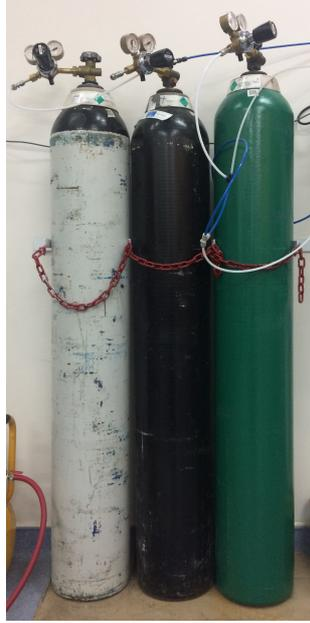
**Figure 3.22** Gas cylinders located at Clean Combustion Laboratory. Green one is nitrogen cylinder used in pyrolysis experiments.
