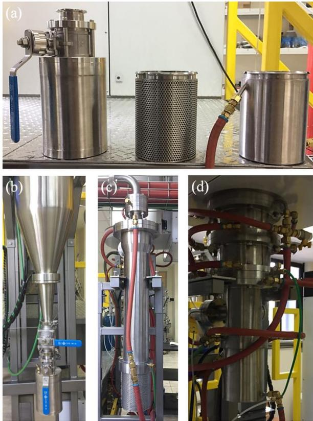
Figure 3. 5 a) Actual design of the bottom collector, cyclone collector, powder collector, respectively. Actual view from the collection unit of the b) bottom collector c) cyclone collector d) powder collector.
