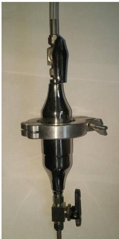
Figure 2. 6 Design of the aerosol filter holder.
