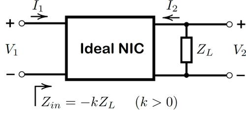
Figure 4.8: An ideal negative impedance converter.
