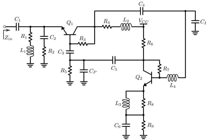
Figure B.1: A grounded negative impedance converter circuit designed to obtain a negative capacitor ( $-47$  pF) in between 10 MHz and 120 MHz.
