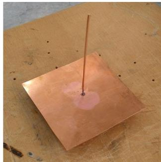
Figure 2.4: The wire monopole antenna with a length of 8 cm and a wire radius of 0.846 mm placed on a copper ground plane.
