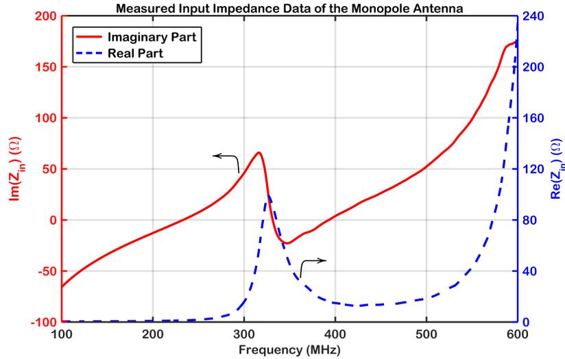
Figure 3.4: Measured input impedance of the unloaded monopole antenna. The solid red line and the blue dashed line represent imaginary and real parts of the input impedance, respectively.
