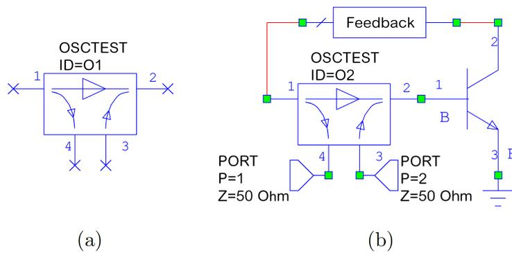
Figure 5.4: Oscillator open-loop test element. (a) OSCTEST component of AWR MWO<sup>®</sup>. (b) Demonstration of the usage.
