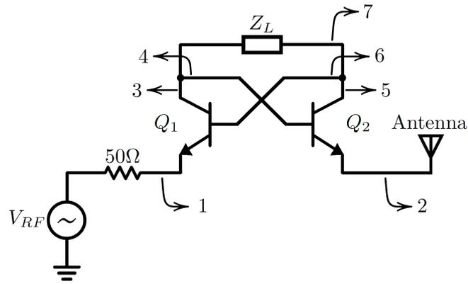
Figure 5.7: A floating OCS NIC circuit connected to an antenna and a  $50\Omega$  input. Branches (1) to (7) for possible stabilization circuits are shown [10].
