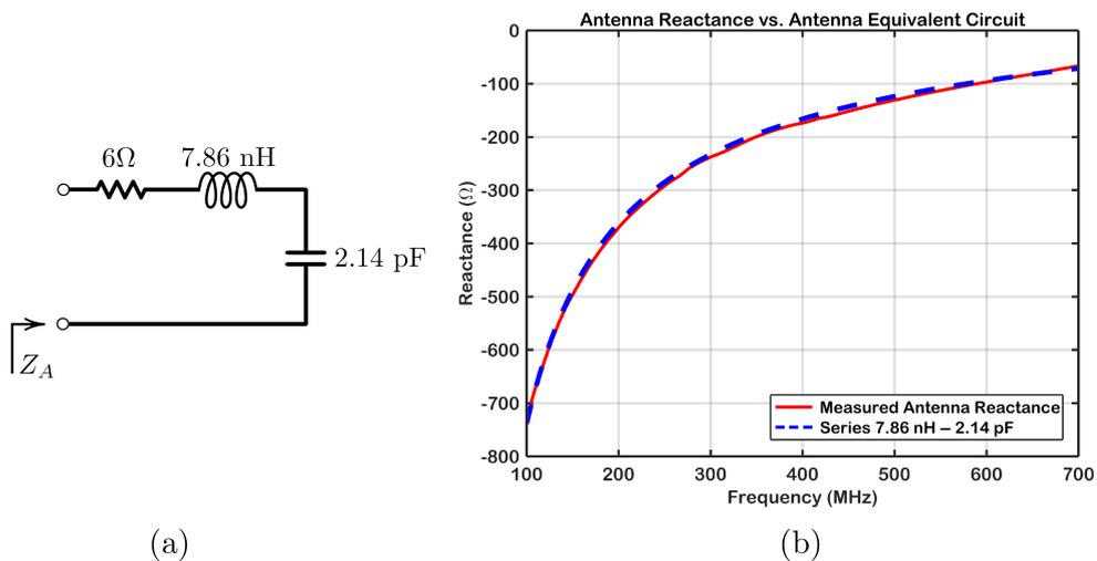
Figure 2.7: Comparison of measured antenna reactance and equivalent circuit that models the antenna reactance in between 100 MHz and 700 MHz.
