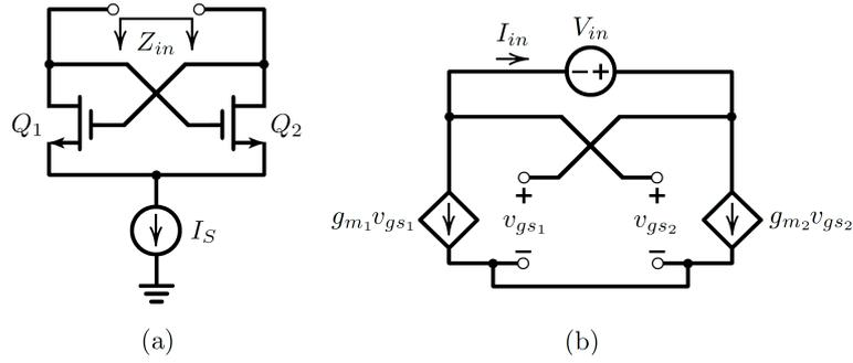
Figure 4.14: (a) Cross-coupled negative resistance circuit. (b) Small-signal equivalent circuit of negative resistance circuit.
