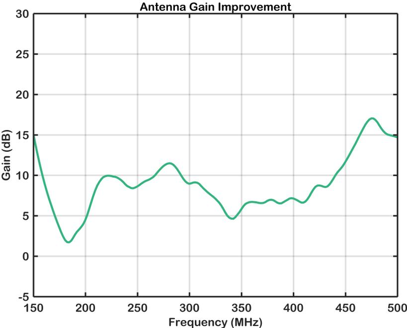
Figure 5.20: Demonstration of the improvement on the antenna gain with the use of non-Foster matching network between 150 MHz and 500 MHz.
