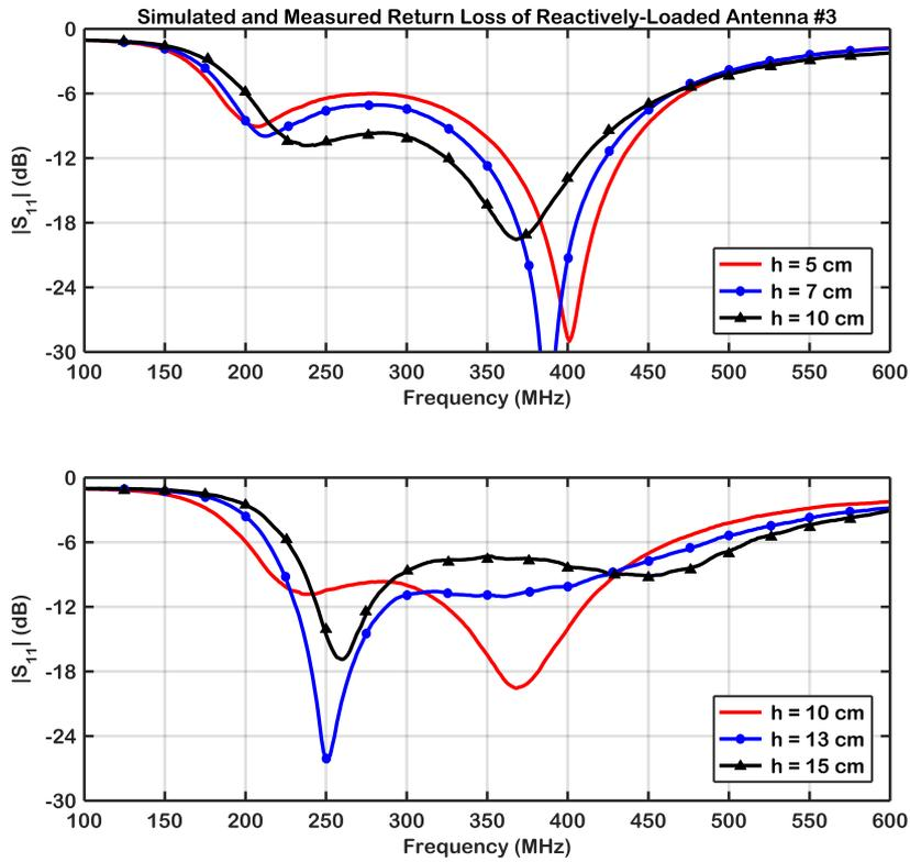
Figure 3.7: Measured return loss data for Design #3 with different load positions: 5 cm, 7 cm, 10 cm, 13 cm and 15 cm.
