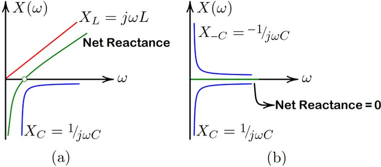
Figure 4.7: Comparison of passive and active matching approaches [1, 7]. (a) Passive matching. (b) Active matching.
