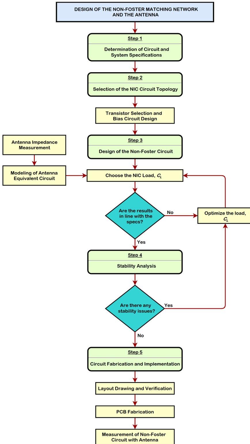
Figure 5.2: Systematical design and implementation procedure of the non-Foster matching network for the electrically-small monopole antenna.
