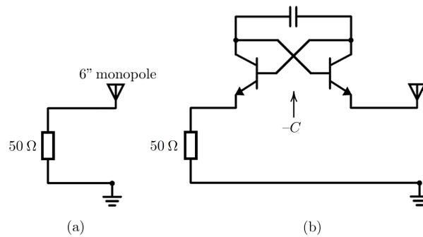
Figure 4.23: The measurement setup presented in Sussman-Fort's paper [7]. (a) 6" monopole antenna connected to 50Ω line. (b) 6" monopole antenna connected to a floating NIC.
