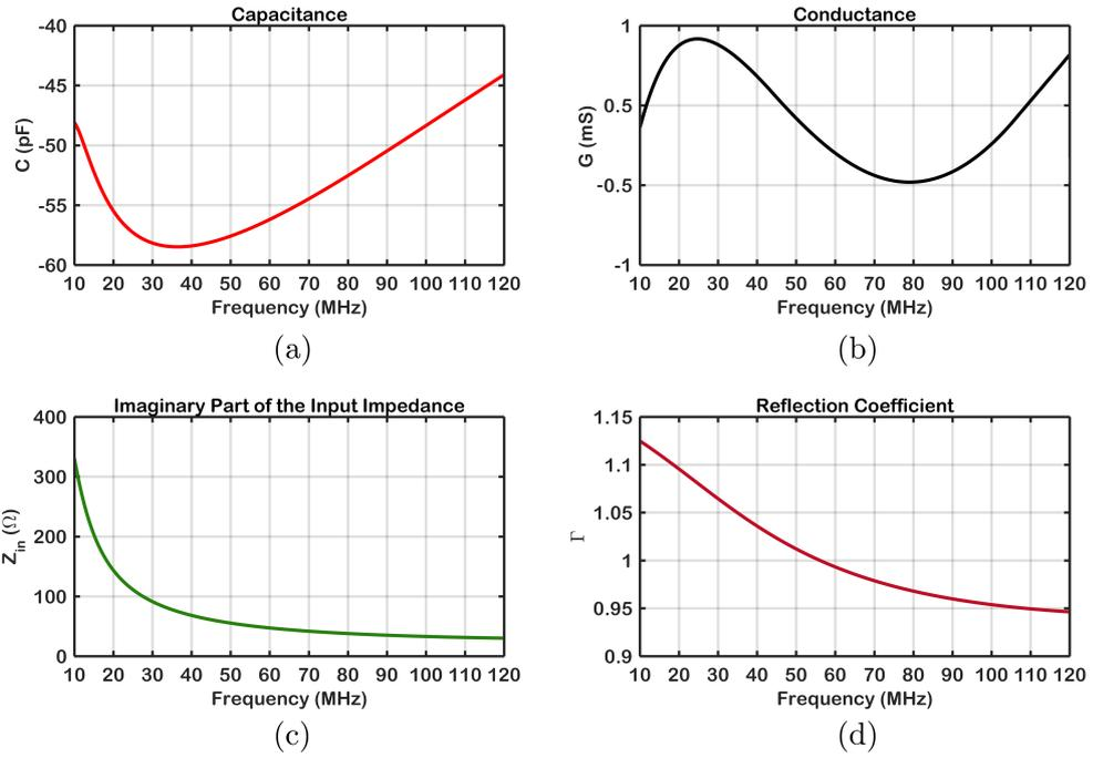
Figure B.2: Simulated results of the grounded NIC circuit presented in Figure B.1 in between 10 MHz and 120 MHz.
