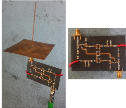
Figure 5.10: Photograph of the fabricated non-Foster matching network containing a negative capacitor ( $-2.4$  pF) for an 8 cm-long wire-type monopole antenna placed on an 8 cm by 8 cm copper ground plane.
