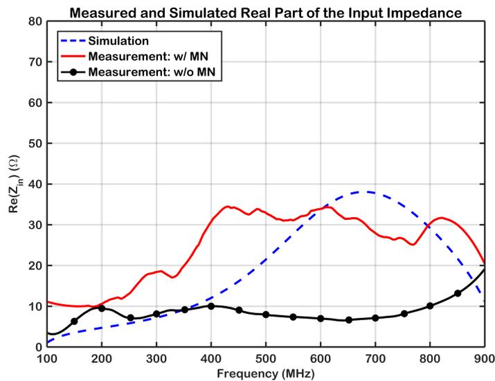
Figure 5.14: Demonstration of the simulation and measurement results for the real part of the input impedance of the overall network with and without the non-Foster matching circuit.
