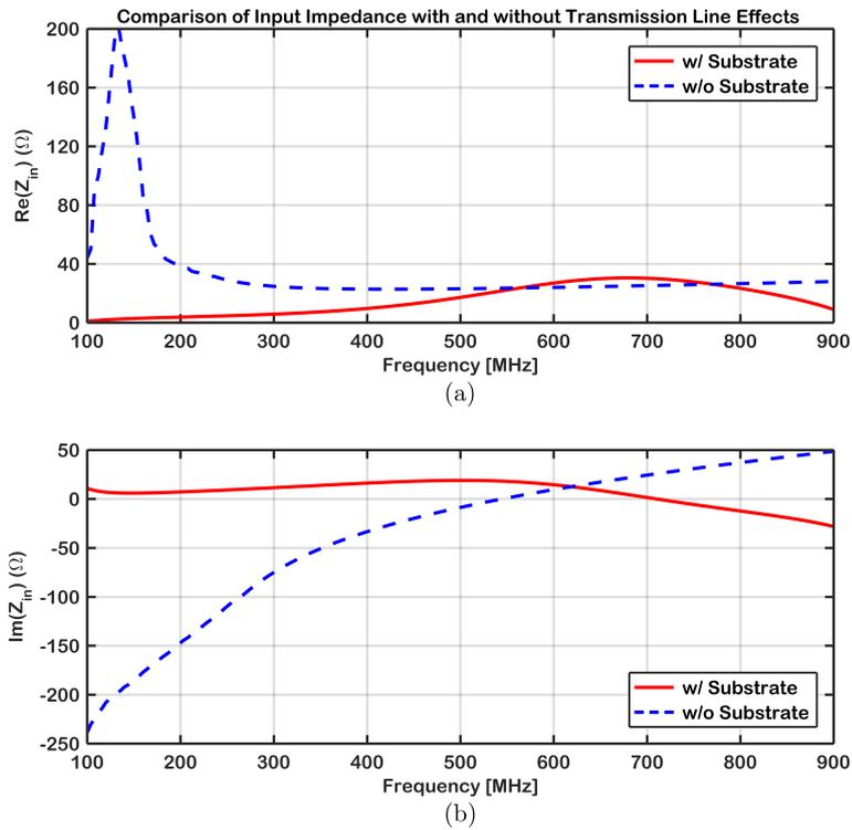
Figure 5.13: Comparison of simulation results of input impedance for the designed non-Foster matching network and the antenna with and without taking transmission line effects into consideration.
