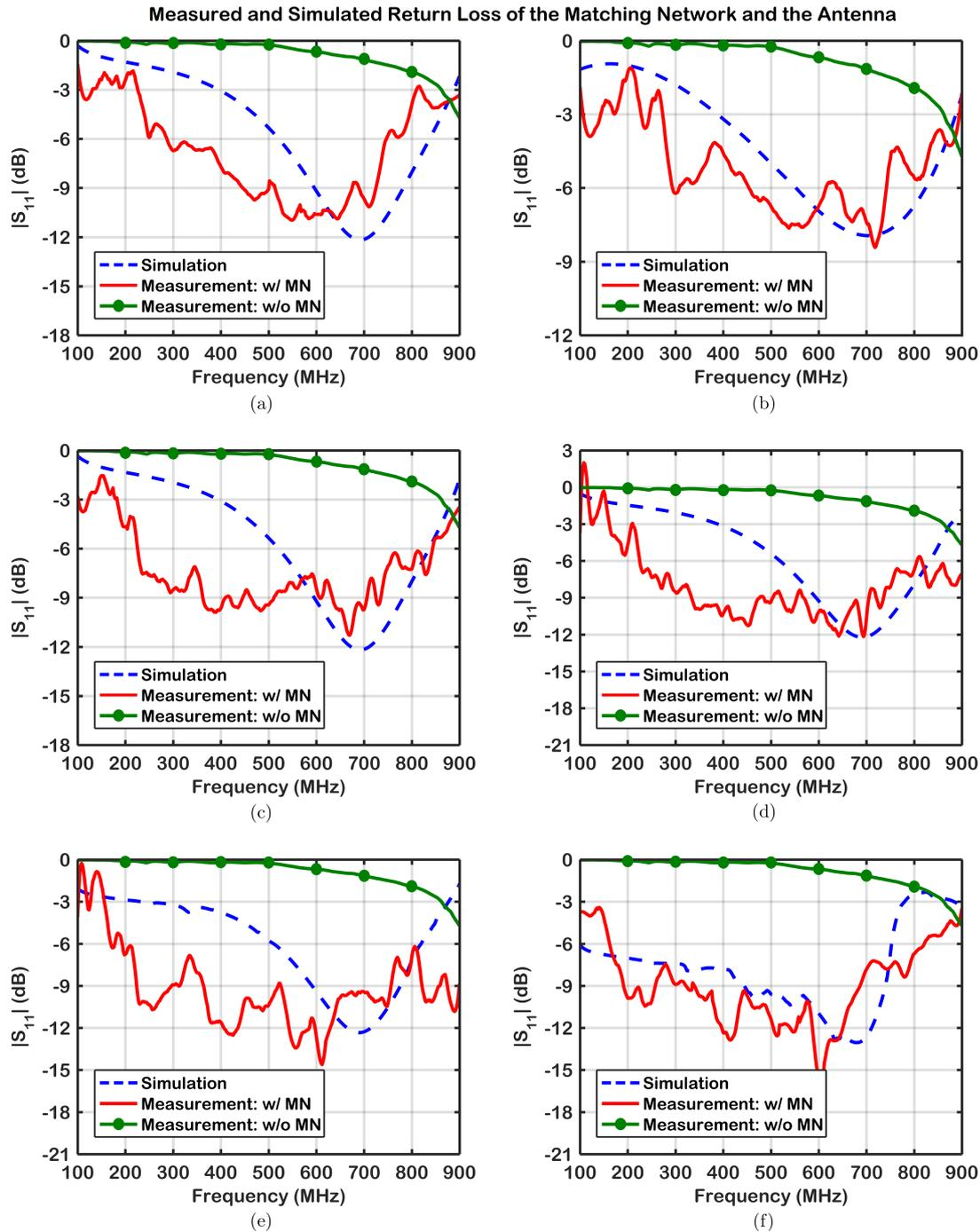
Figure 5.12: Demonstration of the simulated and measured return loss of the overall non-Foster matching network and the antenna for various input power levels. (a)  $P_{in} = -6$  dBm. (b)  $P_{in} = -3$  dBm. (c)  $P_{in} = 0$  dBm. (d)  $P_{in} = 3$  dBm. (e)  $P_{in} = 6$  dBm. (f)  $P_{in} = 9$  dBm.
