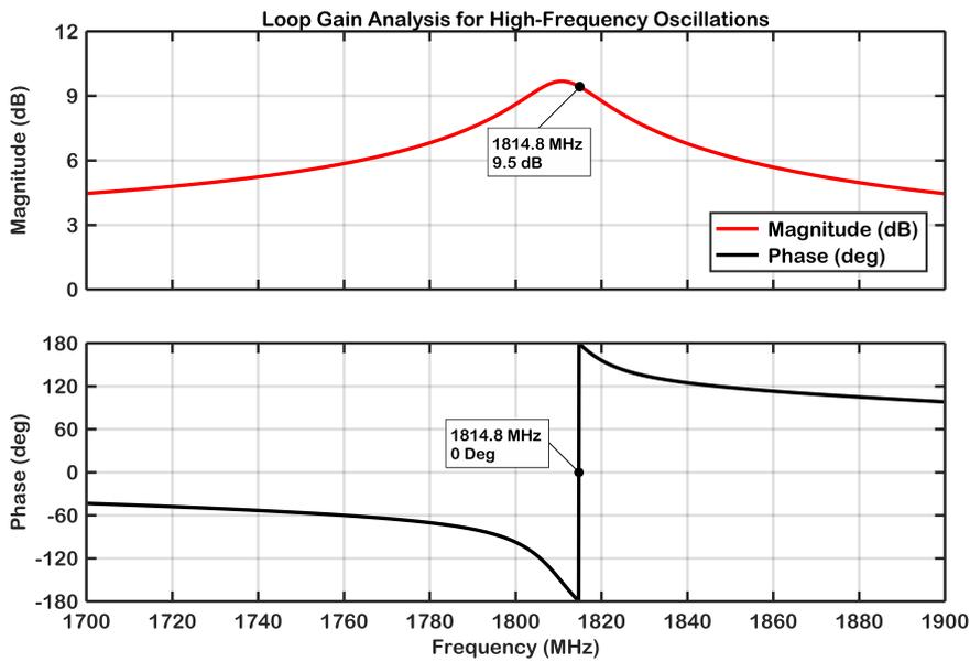
Figure 5.6: Loop gain analysis for the non-Foster matching network at high frequencies. A potentially unstable point at 1.815 GHz is shown using the magnitude-phase plot.
