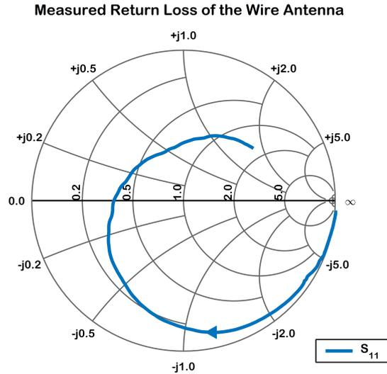
Figure 5.1: Measured return loss for the monopole wire antenna depicted in Figure 2.4. S-parameter data for the monopole antenna is taken in between 50 MHz–1050 MHz range with 1 MHz increments. The return loss line on the Smith chart traces the plot in the clockwise direction.
