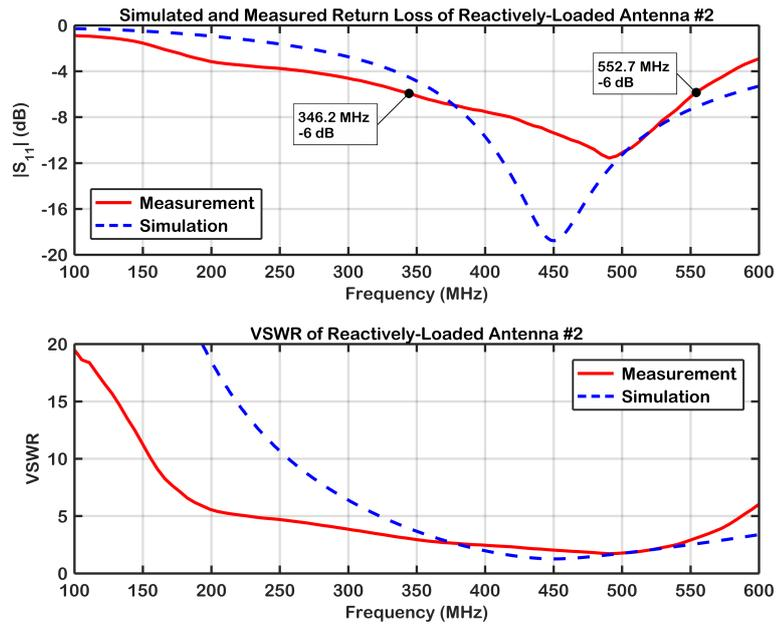
Figure 3.6: Simulated and measured return loss ( $S_{11}$ ) and VSWR data for Design #2. The solid red and blue dashed lines correspond to measured and simulated data.
