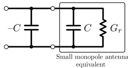
Figure 4.22: Small monopole antenna model given by Harris and Myers [9].
