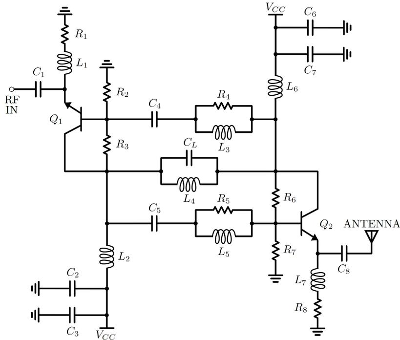
Figure 5.8: Schematic of the stabilized non-Foster matching network with the monopole antenna.
