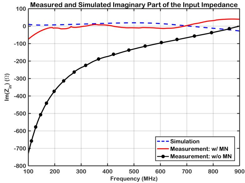
Figure 5.15: Demonstration of the simulation and measurement results for the imaginary part of the input impedance of the overall network with and without the non-Foster matching circuit.
