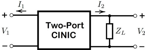
Figure 4.11: The current–inversion negative impedance converter (CINIC).
