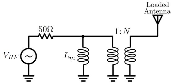
Figure 3.2: An external matching network comprised of a transformer and a shunt inductor is connected to the input terminals of the loaded monopole antenna.
