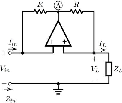
Figure 4.19: An operational amplifier-based grounded negative impedance converter.
