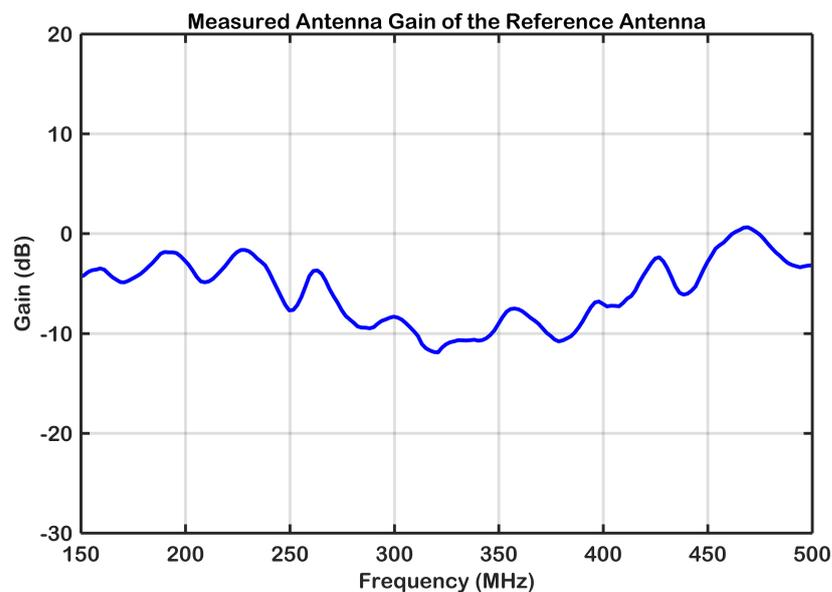
Figure 5.18: Measured antenna gain data of the reference monopole whip with a length of 38 cm for the frequencies in between 150 MHz and 500 MHz.
