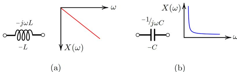
Figure 4.5: Reactance curves for non-Foster elements: (a) A negative inductor. (b) A negative capacitor.
