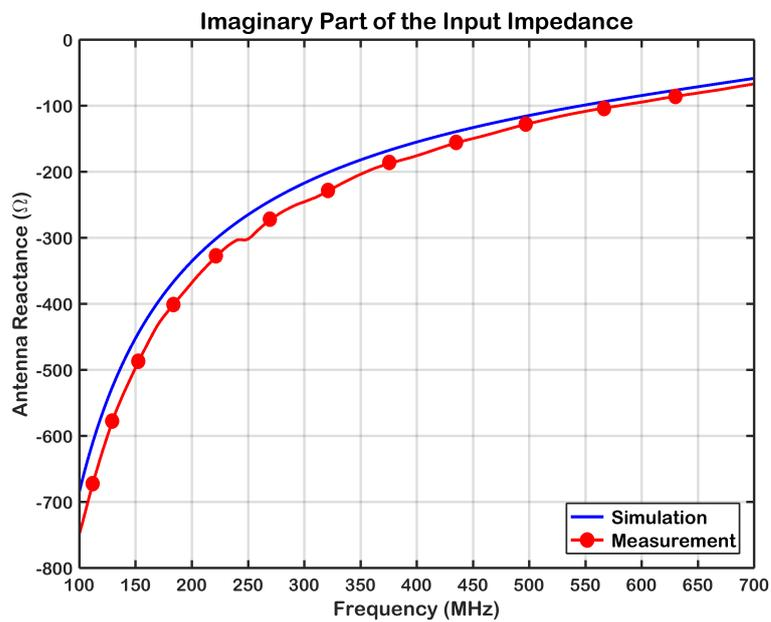
Figure 2.9: The simulated and measured results of imaginary part of the input impedance of the monopole antenna. The blue and red curves represent the simulated and measured results, respectively.
