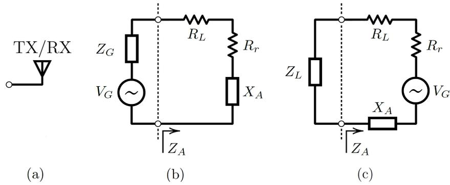
Figure 2.5: Demonstration of the equivalent circuits for transmitting and receiving antennas. (a) A transmitting or a receiving antenna. (b) Equivalent circuit model for the transmitting antenna. (c) Equivalent circuit model for the receiving antenna. [4]
