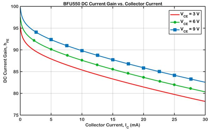
Figure A.3: DC current gain of the transistor BFU550A vs. the collector current ( $I_C$ ) for different collector–emitter voltage levels ( $V_{CE}$ ) plotted using AWR Microwave Office®.
