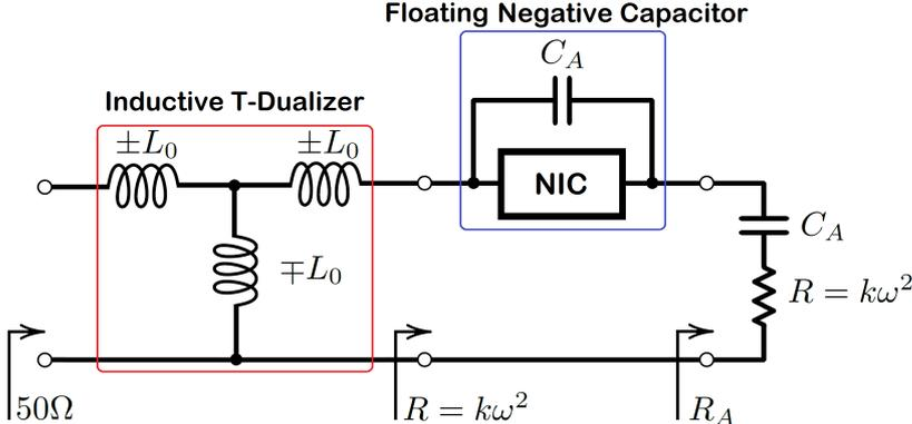
Figure 4.6: The ideal impedance matching circuit that cancels the capacitive reactance of the antenna and frequency–dependent radiation resistance [6].
