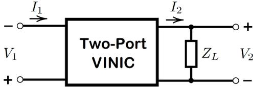
Figure 4.10: The voltage–inversion negative impedance converter (VINIC).
