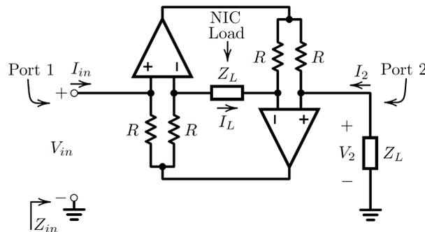
Figure 4.20: An operational amplifier–based floating negative impedance converter.
