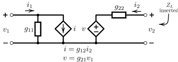
Figure 4.9: The inverse-hybrid (g) parameter representation of a general two-port network.
