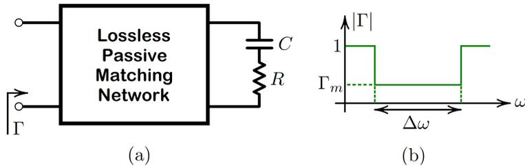
Figure 4.2: An example demonstration of Bode–Fano limit [5]. (a) A series RC circuit and a lossless passive matching network. (b) The reflection coefficient vs. frequency with a minimum reflection coefficient ( $\Gamma_m$ ) in the passband  $\Delta\omega$ .
