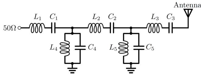
Figure 4.3: An example passive matching network designed to match the electrically–small monopole antenna to 50Ω.
