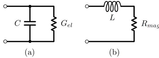
Figure 2.1: The equivalent circuit representation of Wheeler's antennas: (a) Electric dipole. (b) Magnetic dipole. [1, 2]
