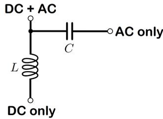
Figure 5.3: Bias-tee configuration that separates the DC and AC signals.
