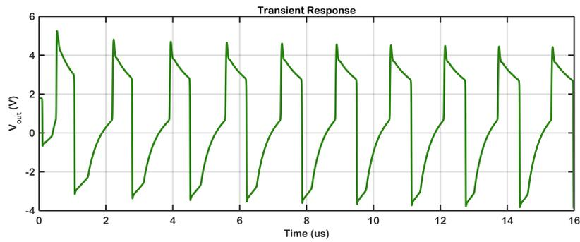
Figure B.3: Transient response of the grounded NIC circuit for  $16 \mu\text{s}$ .
