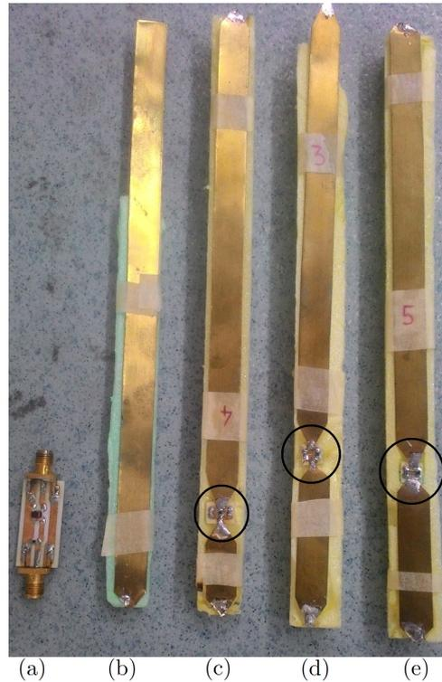
Figure 3.9: Unloaded and reactively-loaded thin monopole antennas. Loads are shown in the black circles. (a) External matching circuit. (b) Unloaded antenna. (c) Loaded antenna used in Design #2. (d) Loaded antenna used in Design #1. (e) Loaded antenna used in Design #3.
