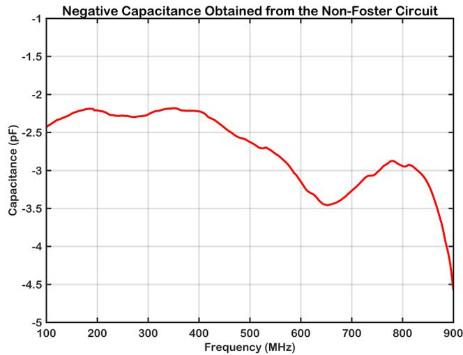
Figure 5.16: Negative capacitance obtained from the designed non-Foster circuit.
