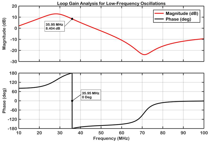
Figure 5.5: Loop gain analysis for the non-Foster matching network at low frequencies. A potentially unstable point at 36 MHz is shown using the magnitude-phase plot.
