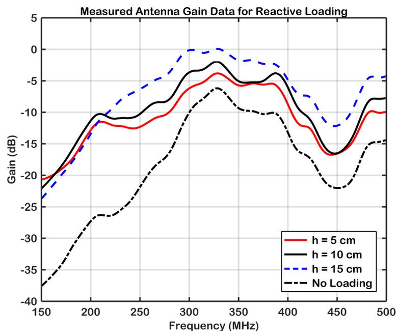
Figure 3.8: Measured antenna gain data of Design #3 for different reactive load positions and the antenna without reactive loading.
