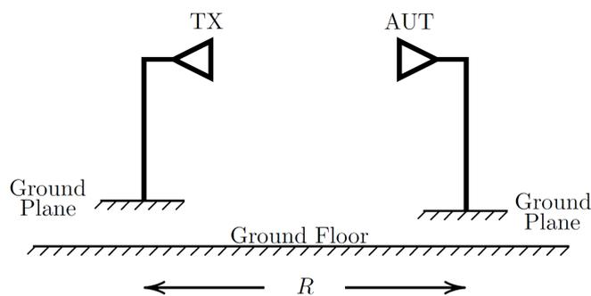
Figure 5.17: Simple demonstration of the gain measurement setup. TX and AUT refer to transmitter antenna and the antenna under test, respectively. The figure is not drawn to scale.
