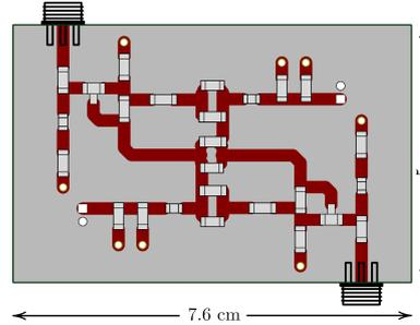
Figure 5.9: Layout of the fabricated non-Foster matching circuit for the electrically-small antenna described in Section 2.2.
