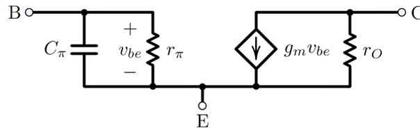
Figure 4.18: Small-signal hybrid- $\pi$  model of a bipolar junction transistor [8].
