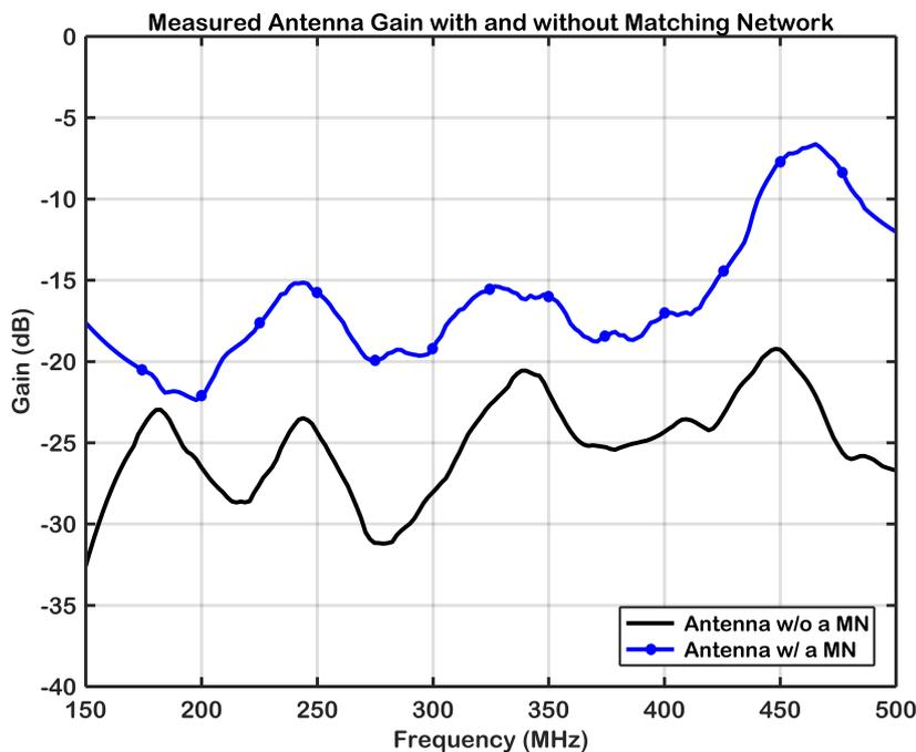
Figure 5.19: Measured antenna gains with and without non–Foster matching network in frequencies between 150 MHz and 500 MHz. Solid dotted blue curve and solid black curve represent the antenna gain with and without a non–Foster matching network, respectively.
