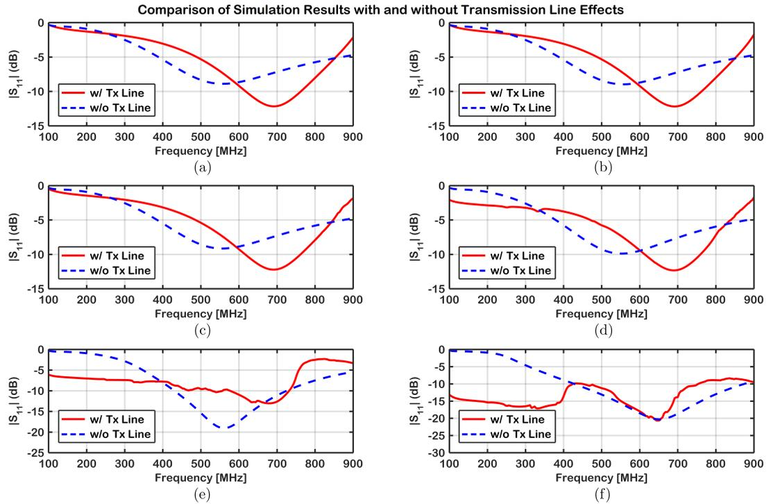
Figure 5.11: Comparison of simulation results of return loss for the designed non-Foster matching network and the antenna with and without taking transmission line effects into consideration. The simulation results are obtained for different input power levels: (a)  $P_{in} = -3$  dBm. (b)  $P_{in} = 0$  dBm. (c)  $P_{in} = 3$  dBm. (d)  $P_{in} = 6$  dBm. (e)  $P_{in} = 9$  dBm. (f)  $P_{in} = 12$  dBm.
