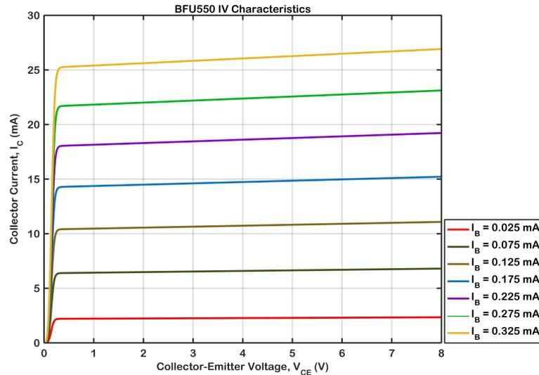
Figure A.1: BFU550 transistor collector current ( $I_C$ ) vs. collector-emitter voltage ( $V_{CE}$ ) characteristics for various base currents ( $I_B$ ).
