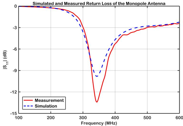
Figure 3.3: Simulated and measured return loss of the unloaded monopole antenna. The solid red line and the blue dashed line represent measured and simulated  $|S_{11}|$  data, respectively.
