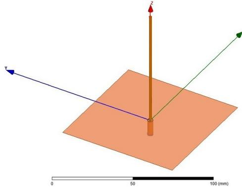
Figure 2.6: HFSS simulation of wire monopole antenna on a metal ground plane.
