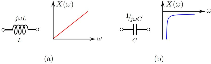
Figure 4.1: Reactance curves for Foster elements: (a) An inductor. (b) A capacitor.
