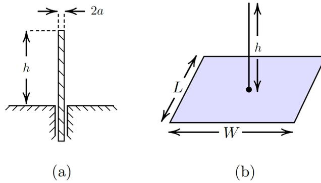
Figure 2.3: The geometry of a monopole antenna with wire and the ground plane. (a) Side view. (b) 3D view.
