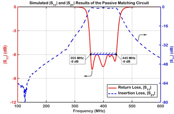
Figure 4.4: Simulated return loss ( $S_{11}$ ) and insertion loss ( $S_{21}$ ) results of the matching circuit comprised of passive lumped circuit elements and the electrically–small antenna.
