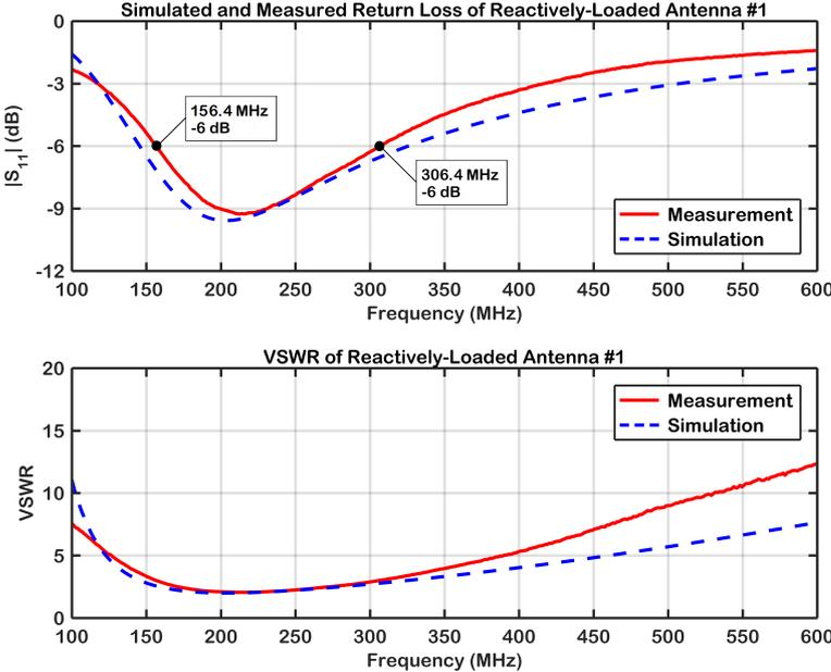
Figure 3.5: Simulated and measured return loss ( $S_{11}$ ) and VSWR data for Design #1. The solid red and blue dashed lines correspond to measured and simulated data.
