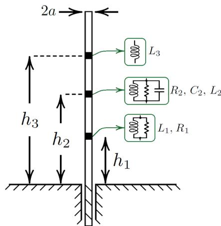
Figure 3.1: An example demonstration of a loaded wire monopole antenna with three different load sections with  $h_1$ ,  $h_2$  and  $h_3$  being the heights of each load, and  $a$  is the wire radius.
