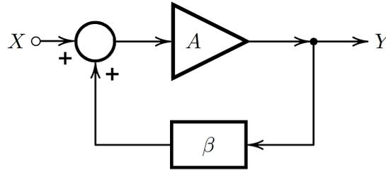
Figure 4.21: A general positive feedback circuit.
