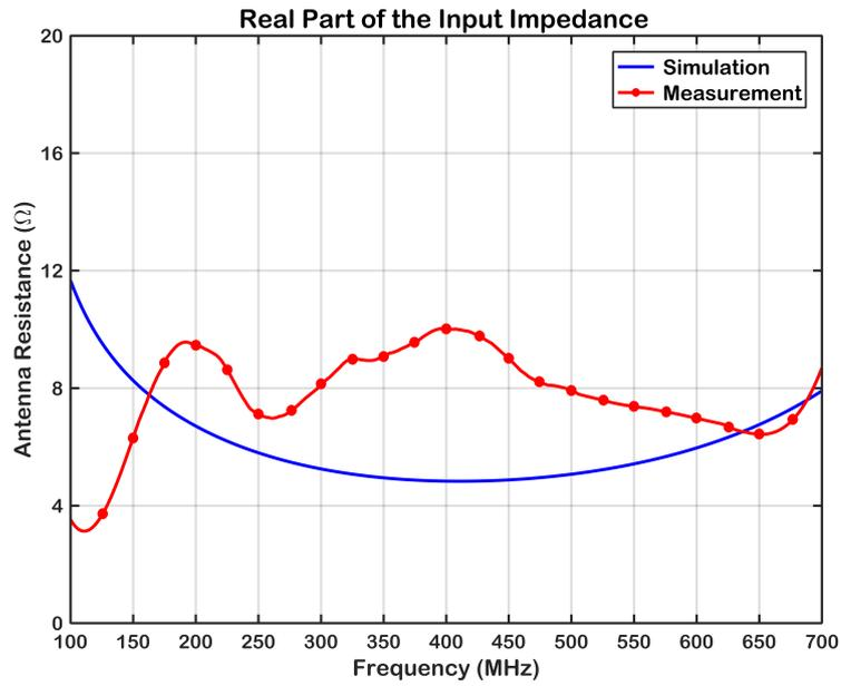
Figure 2.8: The simulated and measured results of real part of the input impedance of the monopole antenna. The blue and red curves represent the simulated and measured results, respectively.
