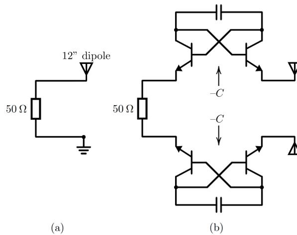
Figure 4.24: The measurement setup presented in Sussman–Fort’s paper [7]. (a) 12" dipole antenna connected to  $50\Omega$  line. (b) 12" monopole antenna connected to two floating NICs.
