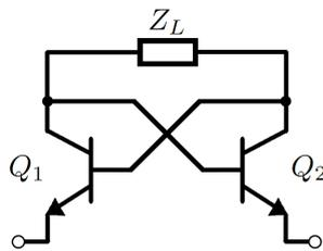
Figure 4.17: Linvill's floating OCS negative impedance converter circuit.
