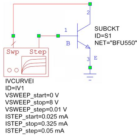
Figure A.2: Implementation of IVCURVEI element of AWR Microwave Office<sup>®</sup> software for the characterization of BFU550A transistor.
