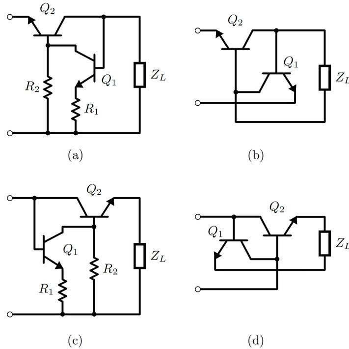
Figure 4.15: Linvill's ideal negative impedance converters terminated by an arbitrary impedance  $Z_L$ . (a) Grounded OCS NIC circuit. (b) Floating OCS NIC circuit. (c) Grounded SCS NIC circuit. (d) Floating SCS NIC circuit.
