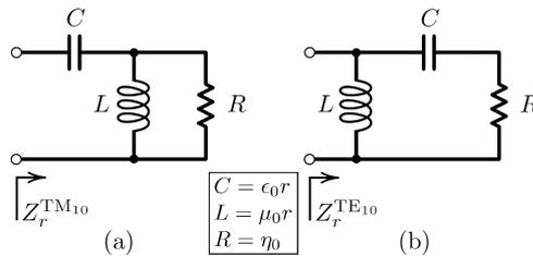
Figure 2.2: The equivalent circuit model for (a)  $TM_{10}$  mode and (b)  $TE_{10}$  mode [1, 3].
