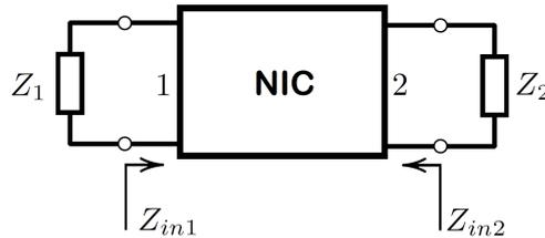
Figure 4.16: Demonstration of Brownlie-Hoskins theorem. Port 1 and Port 2 are terminated by impedances  $Z_1$  and  $Z_2$ , respectively.
