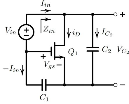
Figure 4.13: A MOSFET circuit generating a negative resistance.
