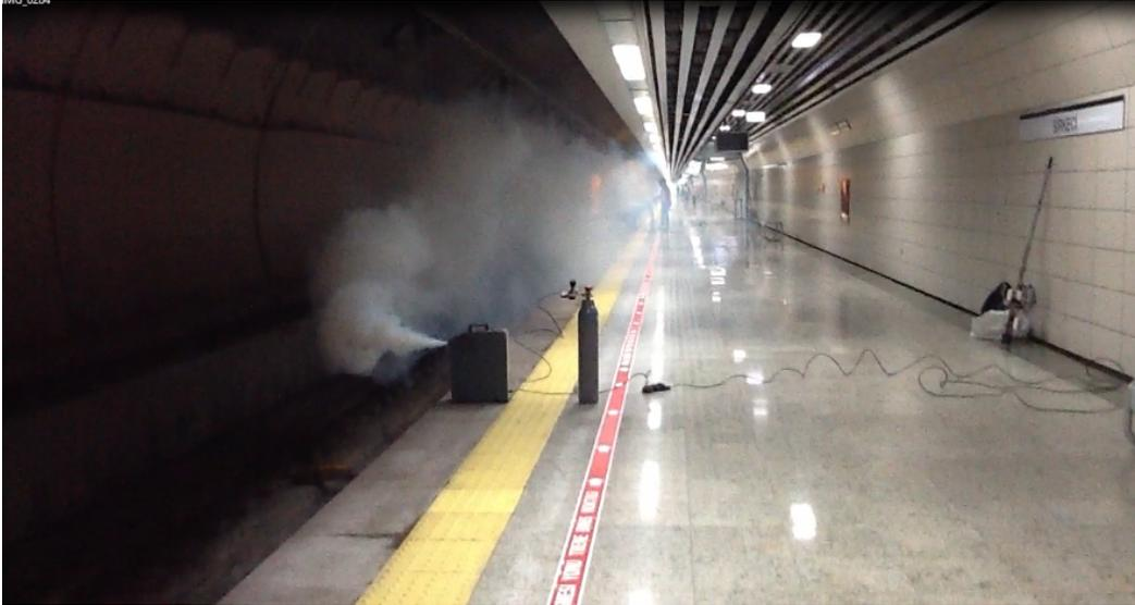
Figure 1.13: Smoke Test in Sirkeci Metro Station
