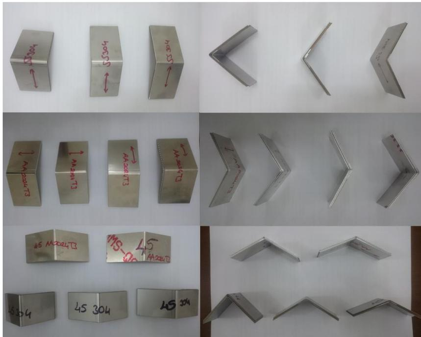
Figure 5.16 Specimens after bending operation
