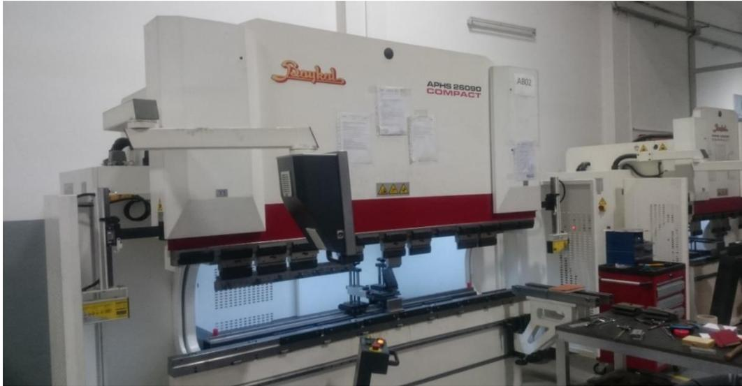
Figure 5.12 Hydraulic bending press used during experiments
