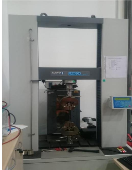
Figure 5.3 Lloyd LR100K tension test machine
