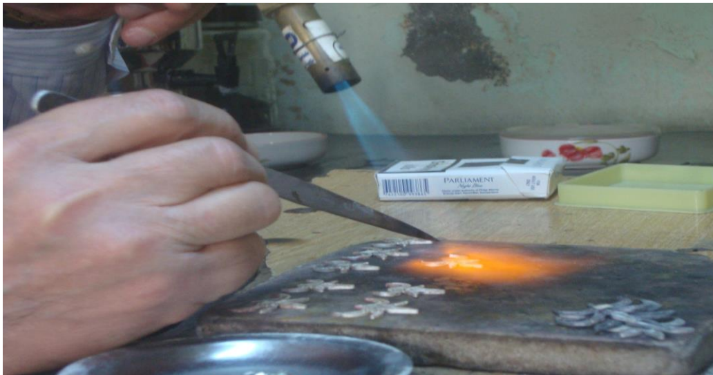
Photo 4.3: This phase is welding of millimetric wires
