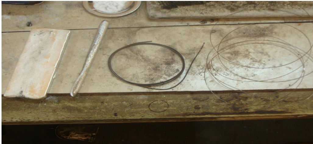
Photo 4.1: Bullion of silver is turned into silver sticks in a rolling mill and then these sticks are worked up into a wire (thinner than a strand of hair) by artisan.
