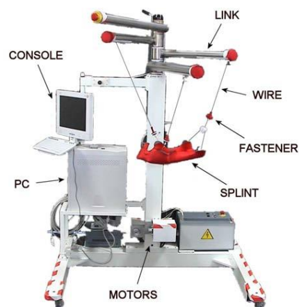
Figure 1.15: Cable Robot with 3 Wires used for Upper Limb Neurorehabilitation, named NeReBot [17]
