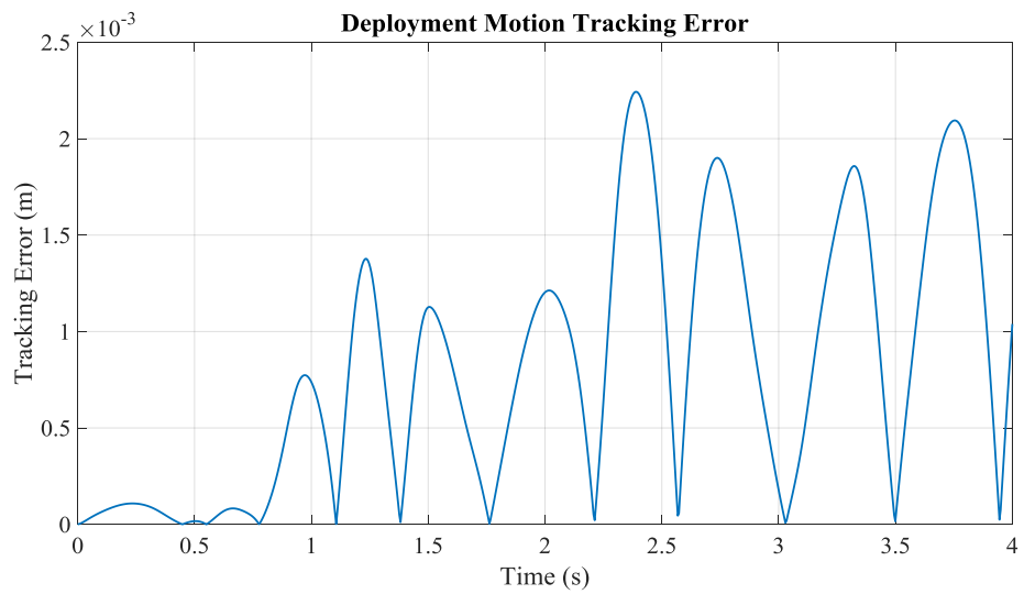
Figure 4.45: Deployment Motion Tracking Error under Command “D-P3-x”
