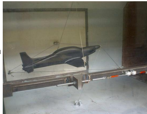
Figure 1.24: A Cable Robot with 8 Cables used in Low-Speed Wind Tunnel [27]
