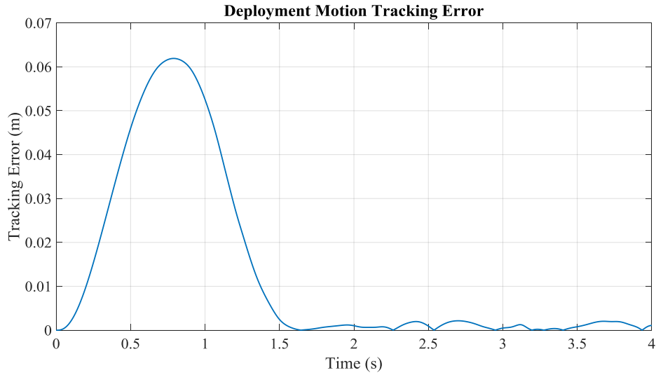
Figure 4.89: Deployment Motion Tracking Error under Command “D-P3-x”
