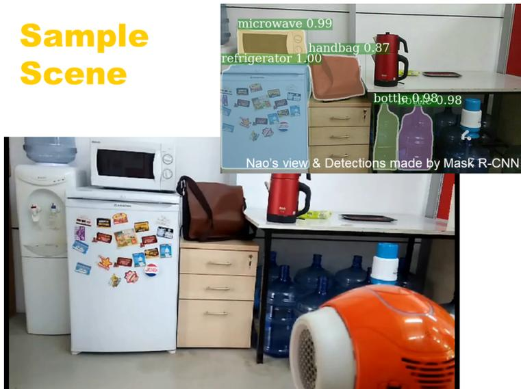
Figure 5.13: A snapshot of an experiment performed with Nao (Task 9). Nao uses Mask R-CNN to detect objects in the scene, and COSMO is initialized with these detections. Once this has been performed, Nao can reason about relations, affordances, missing objects or out-of-context objects in the scene. See the accompanying video (also provided at <https://bozcani.github.io/COSMO>) for the experiments.
