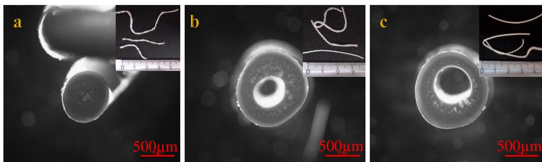
**Figure 3.29.** Microscope images of the membranes H133 (a), H132 (b) and H131 (c).
