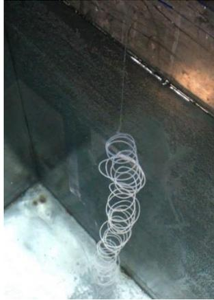
**Figure 1.12.** Liquid rope coil effect forming large coils on the PES solution.
