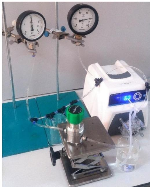
**Figure 2.4.** Picture of performance tests cross-flow system.
