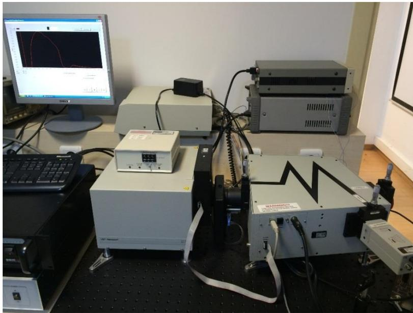
**Figure 3.13:** Monochromator device and overall setup utilized in responsivity measurements.
